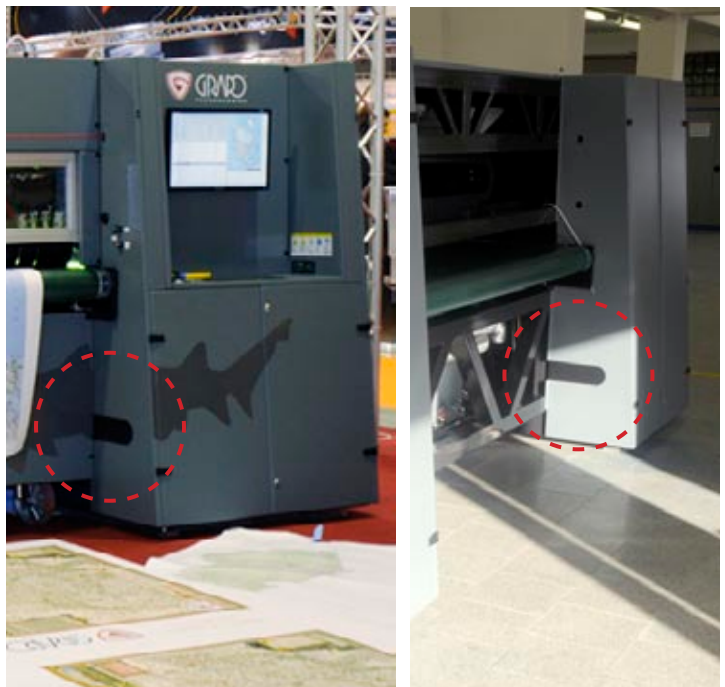
The slots in the lower areas at the front and at the back show that this printer will have the option of a fixed spindle (or saddle) to hold rolls of media. The only combo printer using pinch rollers that I can think of is the IP&I 1606.
