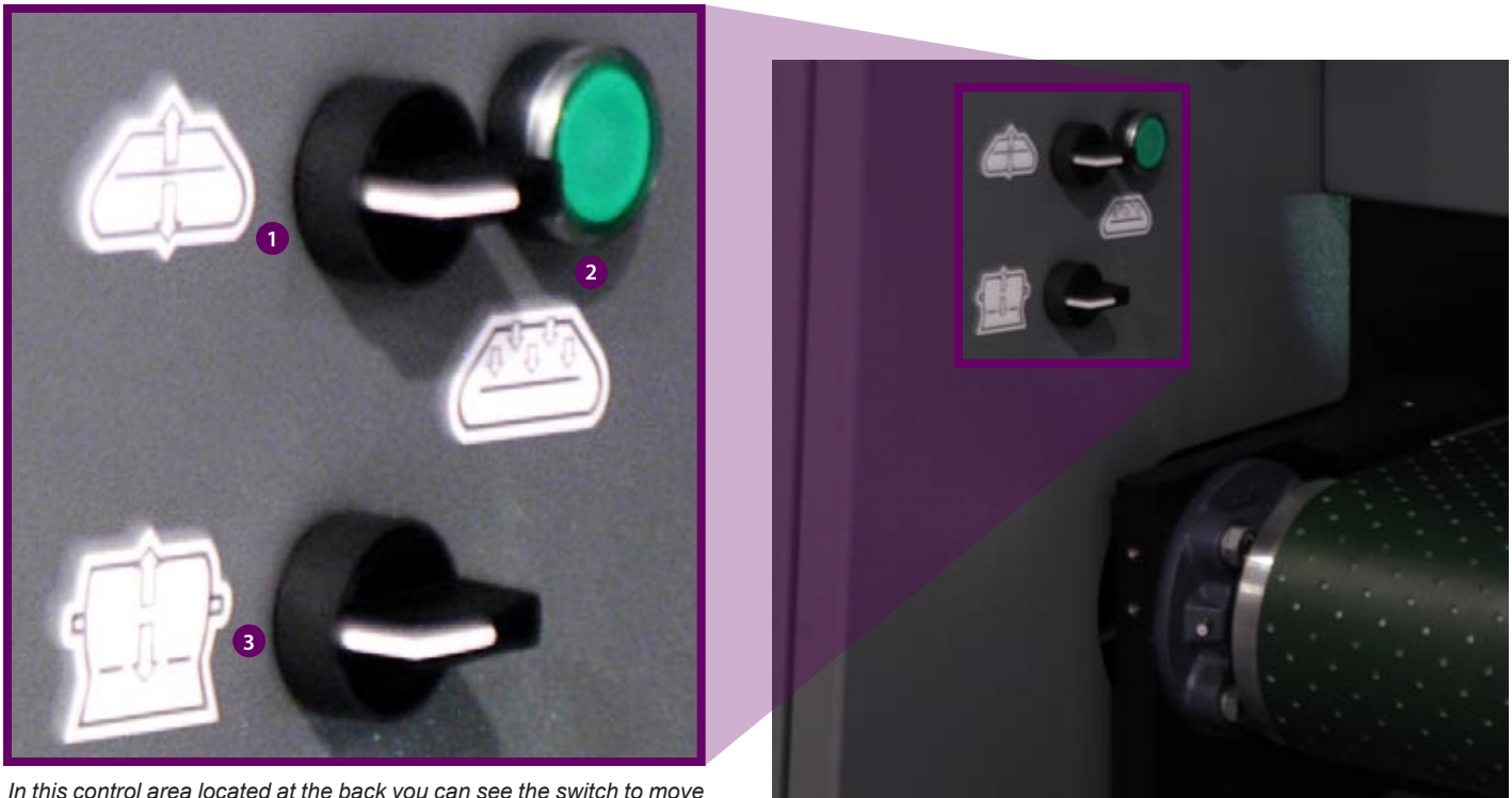
In this control area located at the back you can see the switch to move the transport belt forwards and backwards (1), turn on and off the vacuum (2), and wind/rewind the spindle (3).
