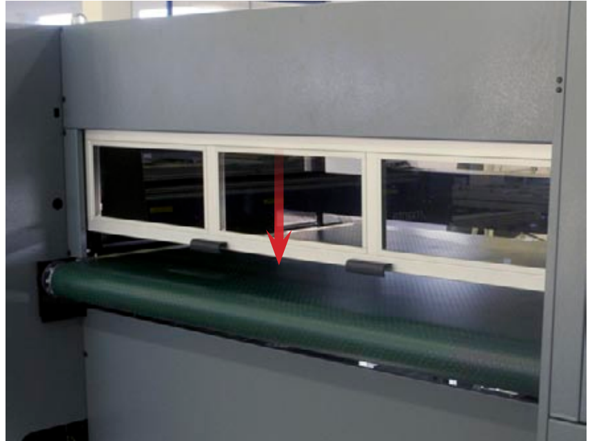
The design of the hood is unique in the sense that most hoods open up with hinges.
