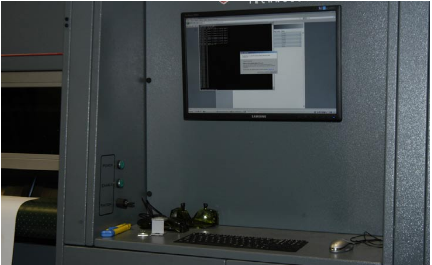
The design of the main control area is clean. there are only a few buttons. Most operations are software-based: the operator controls the printer using the keyboard and the mouse.
