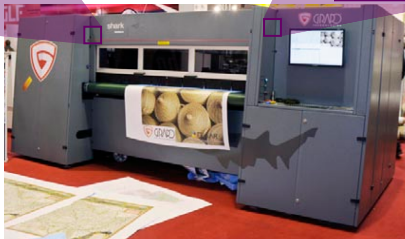
At the top you can see industrial-size screw-eyes to lift the printer.
