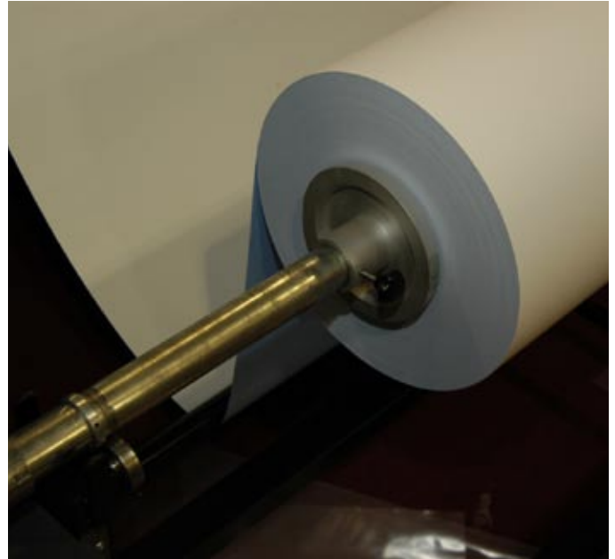
Roll-fed material is held on a spindle. As you can see, the structure that holds the spindle is not fixed into the printer, it is an independent frame.
