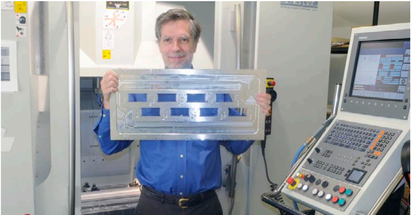
Grapo has their own CNC machining tools. Here is Nicholas with a precision tooled printhead plate for a test prototype of a predecessor of the Shark. The actual printer model today has a different configuration. When you have your own CNC machine in-house you can build a better printer more quickly.
