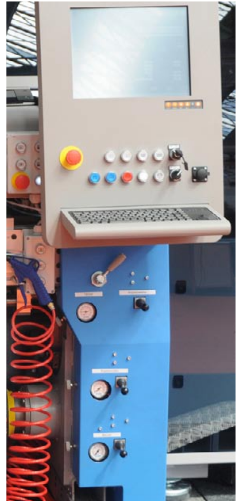
Most of the operations are controlled via software, but below the keyboard you see levers, toggles and gauges.
