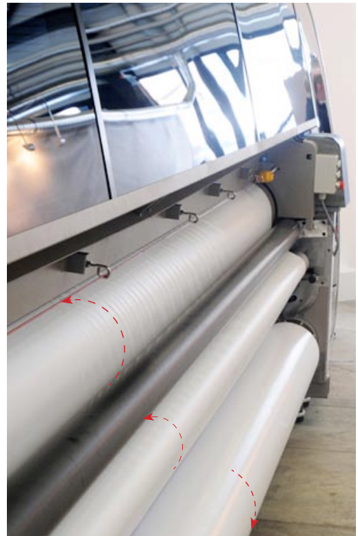
The WP Digital Virtu RR50 is a dedicated roll-to-roll printer.
