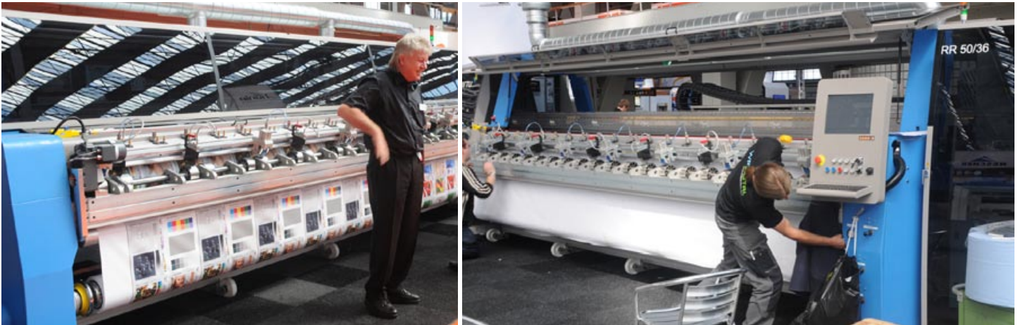
The hood opens upward. In the photo at the left you see the hood down; in the photo at the right, the hood has been lifted.
