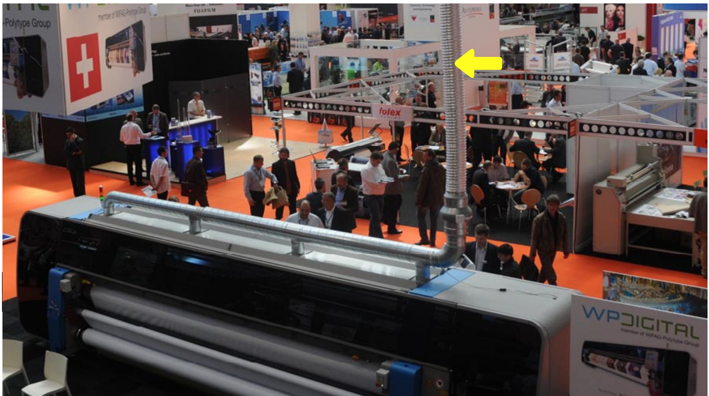
WP Digital booth shot from above at FESPA '09. You can see the exhaust hose necessary to maintain a healthy work environment.
