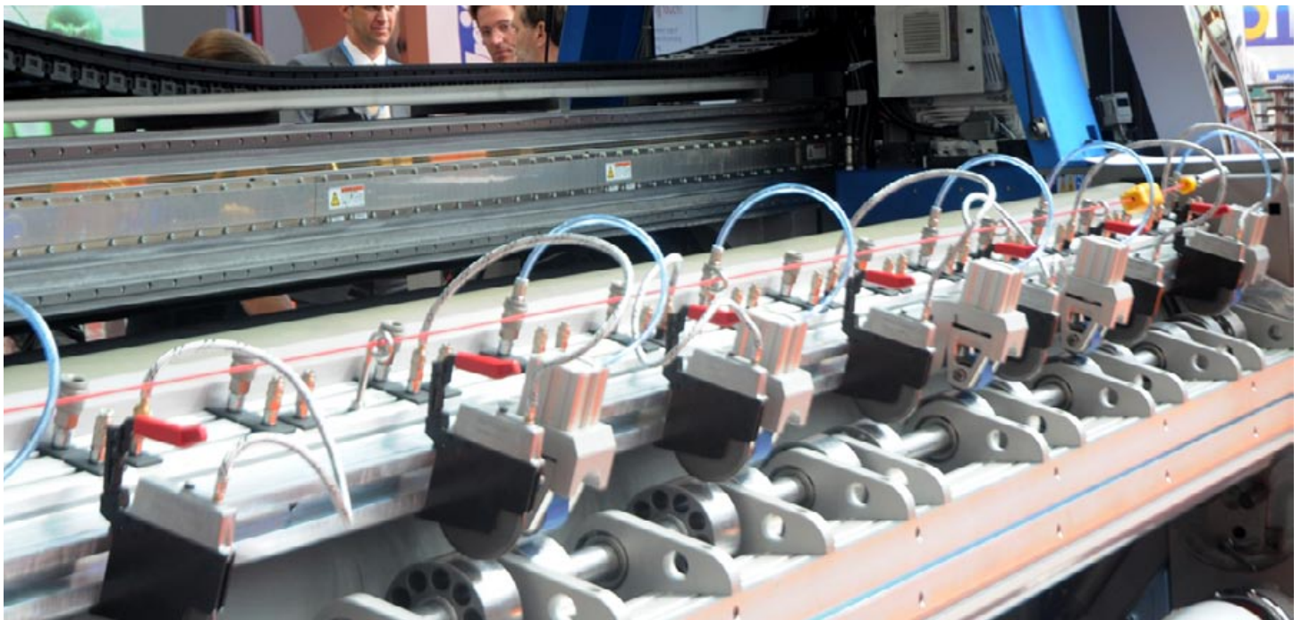
The slitting unit is located at the front, just after the printing area. These knives are adjusted manually but they work automatically.
