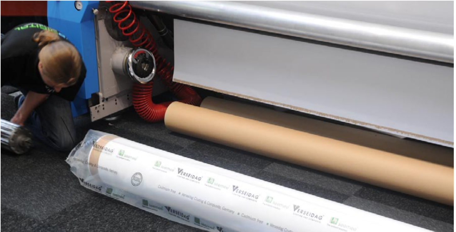
Here you see one of the operators about to introduce the spindle to through the core of a fresh roll. Most roll-fed materials don't need cleaning or any major preparation.
