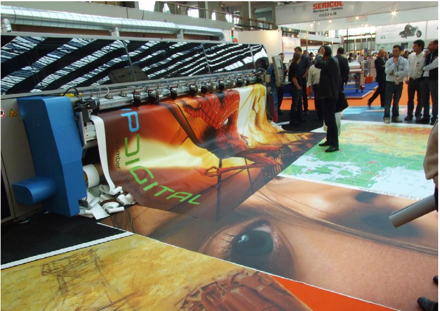
The samples printed by the Virtu RR50 were awesome. The colors looked real and the quality of the images was also excellent. If you notice the media being printed is being cut in the Y axis (look at the edges) so that the printed image is borderless.
