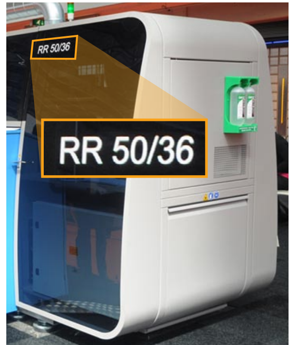
The 50 stand for the 5000mm print width and the 36 represent the number of printheads. So there is a version called WP Digital Virtu RR 50/48.
