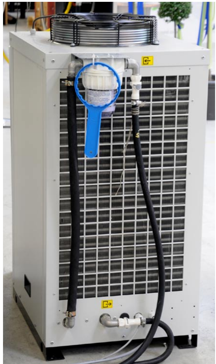
The UV-curing system is cooled by this unit that works with water.
