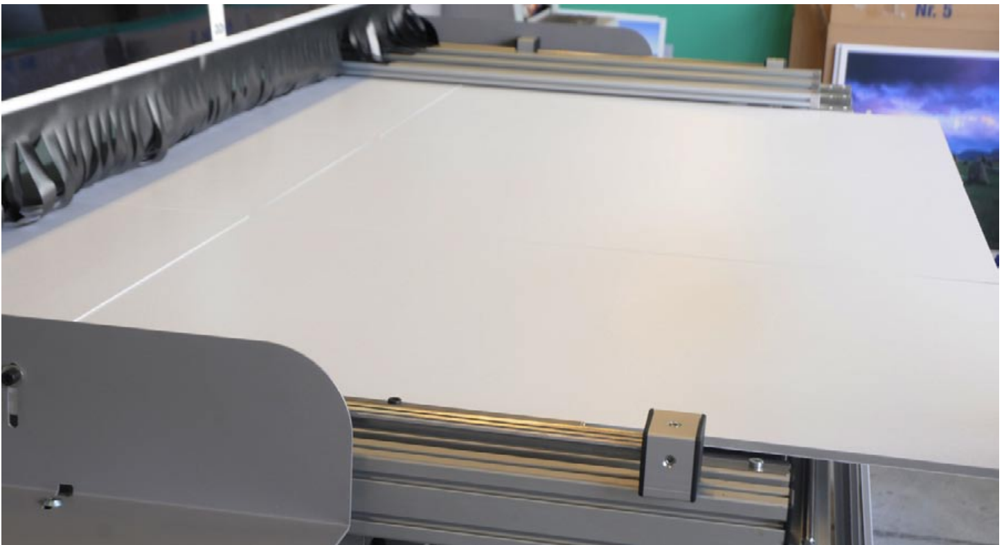
As discussed earlier, this is a combo printer. The advantage of this type of printers is that it handles rigid and roll-fed media.
