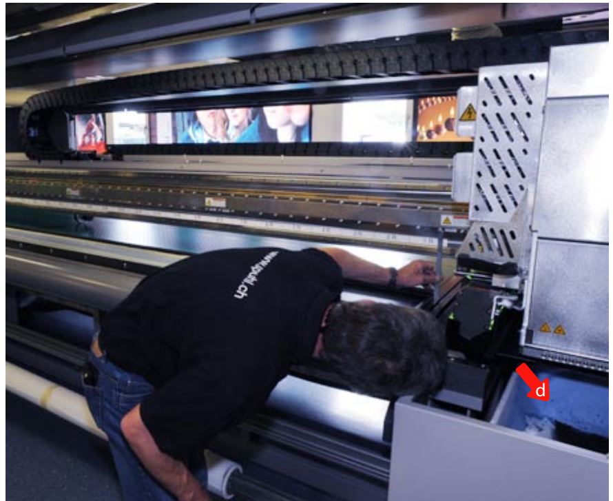
The cleaning station is at the front right. The inks that are purged go to a drip tray (d).
