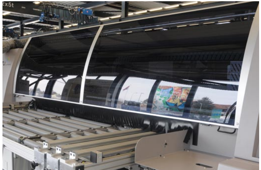
UV light is shielded by Plexiglas tinted windows at the front and back.
