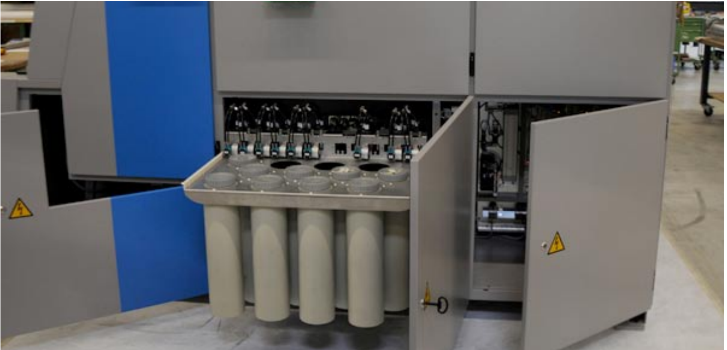
Ink containers located at right end cabinet.
