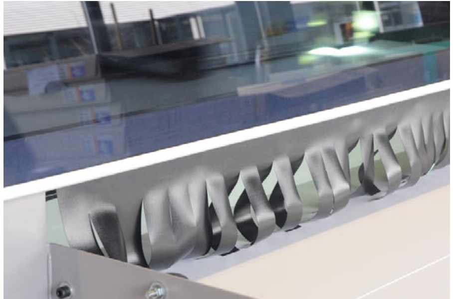
The hood has rubber-like flaps on the edge to let rigid media through. This flaps also protect from the UV-light.
