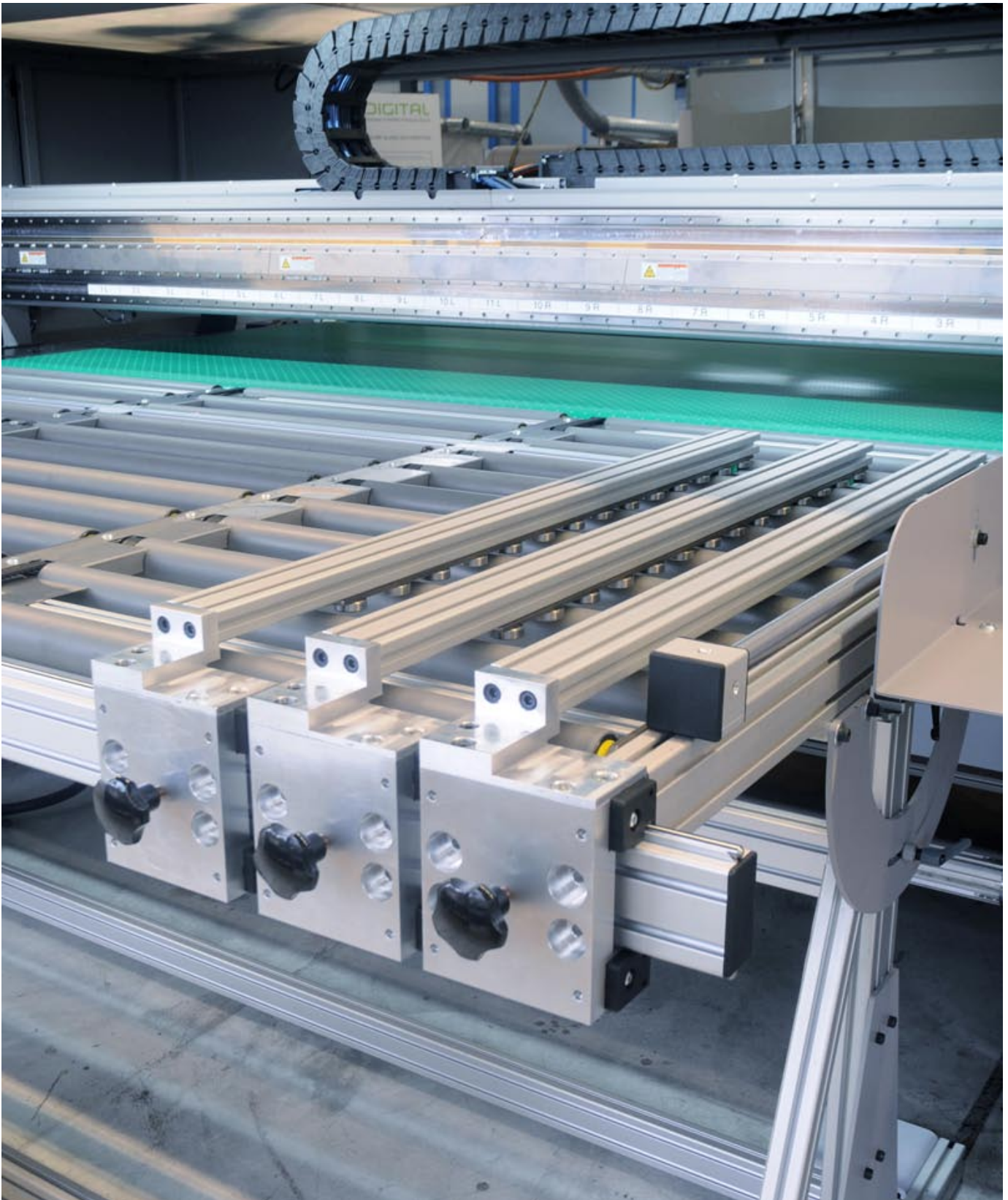
The front table is a sophisticated structure that has adjustable edges to align multiple boards of rigid media.
