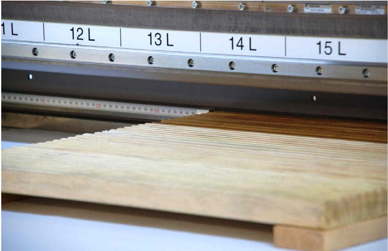
Wooden floor block for a sauna positioned in the UV-curable combo flatbed printing machine.
