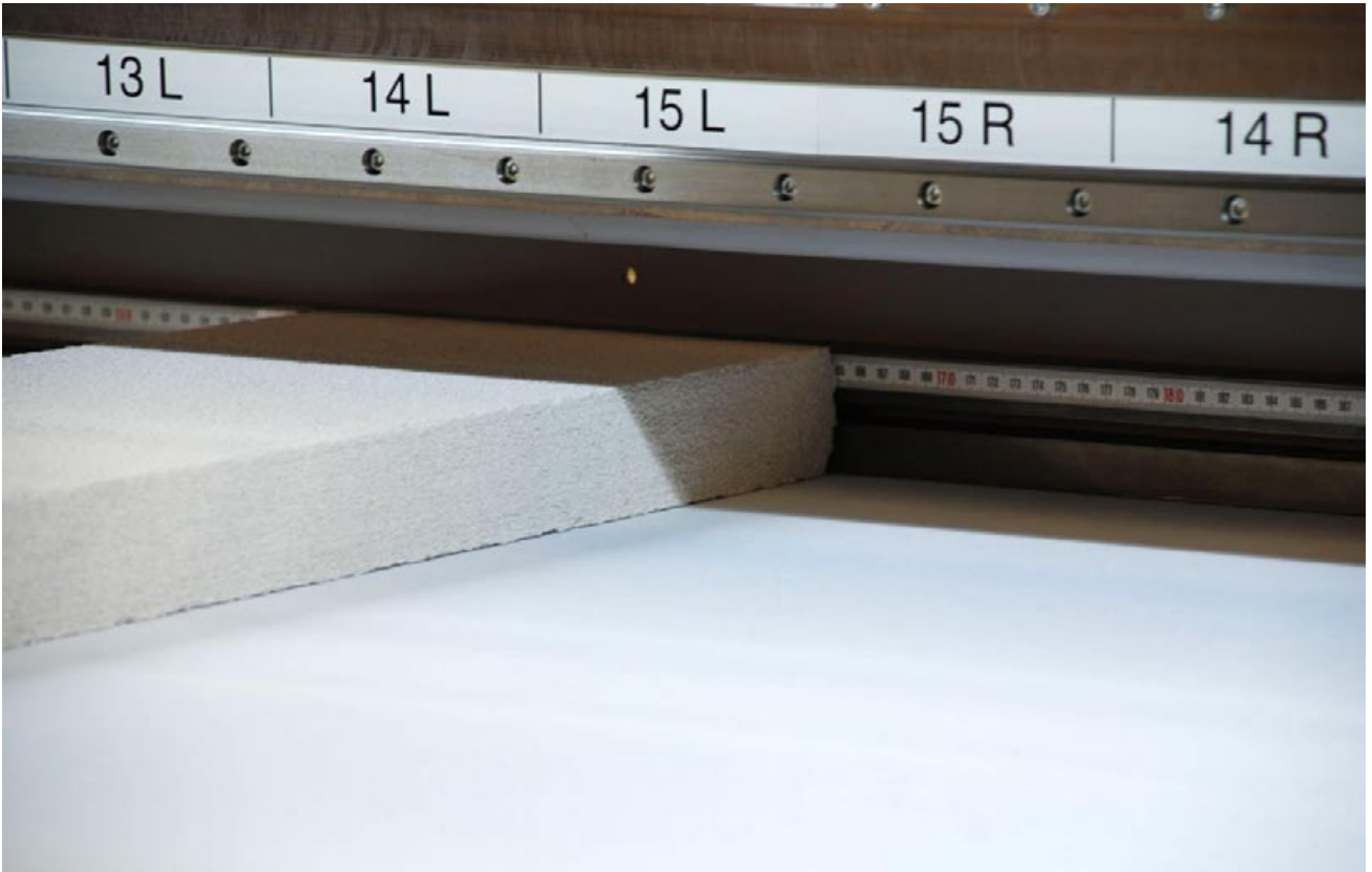
Concrete in the WP Digital Virtu R Concrete slab inside the WP Digital Virtu RS35 UV printer. You might want to consider using a vacuum cleaner to suck off excess dust before you start printing. S35 UV printer.
