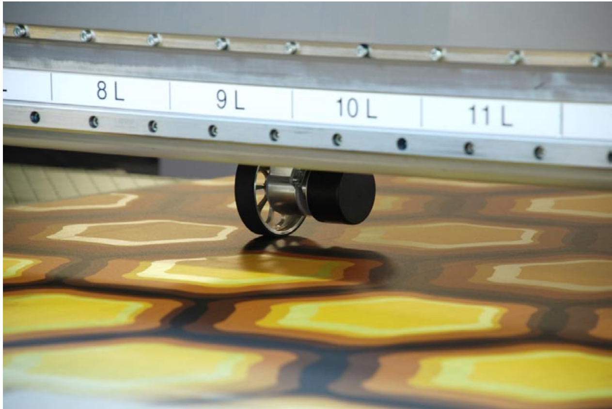
Wooden floor printing in dedicated flatbed mode, notice the encoder wheel.
