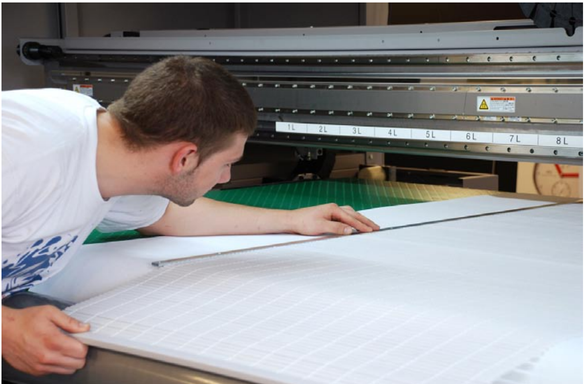
A plastic curtain being positioned in the machine before printing. Yes, you can print on dozens and dozens of materials for interior decoration: thick, thin, rigid, roll-fed.
