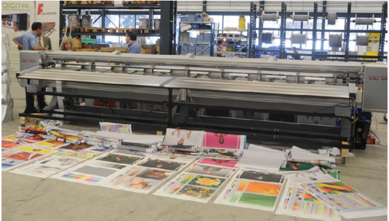
Fotoba cutter-trimmers cleverly occupy a niche of trimmers that, so far, no other competitor has successfully gone into. Fotoba cutters are not intended for foamcore; Zund, Gerber M, and DYSS cutters handle all that.
