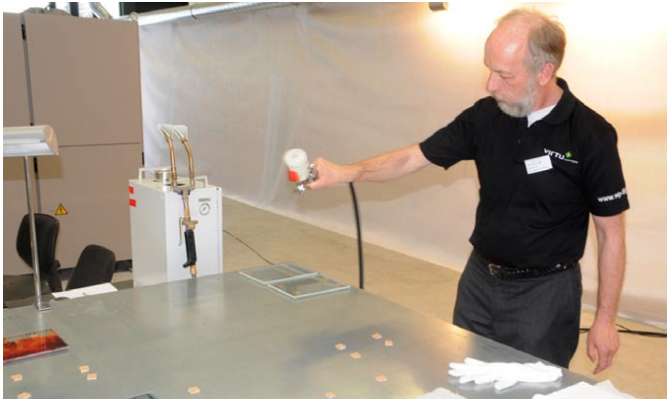
Third step in glass preparation, spray-on the primer.
