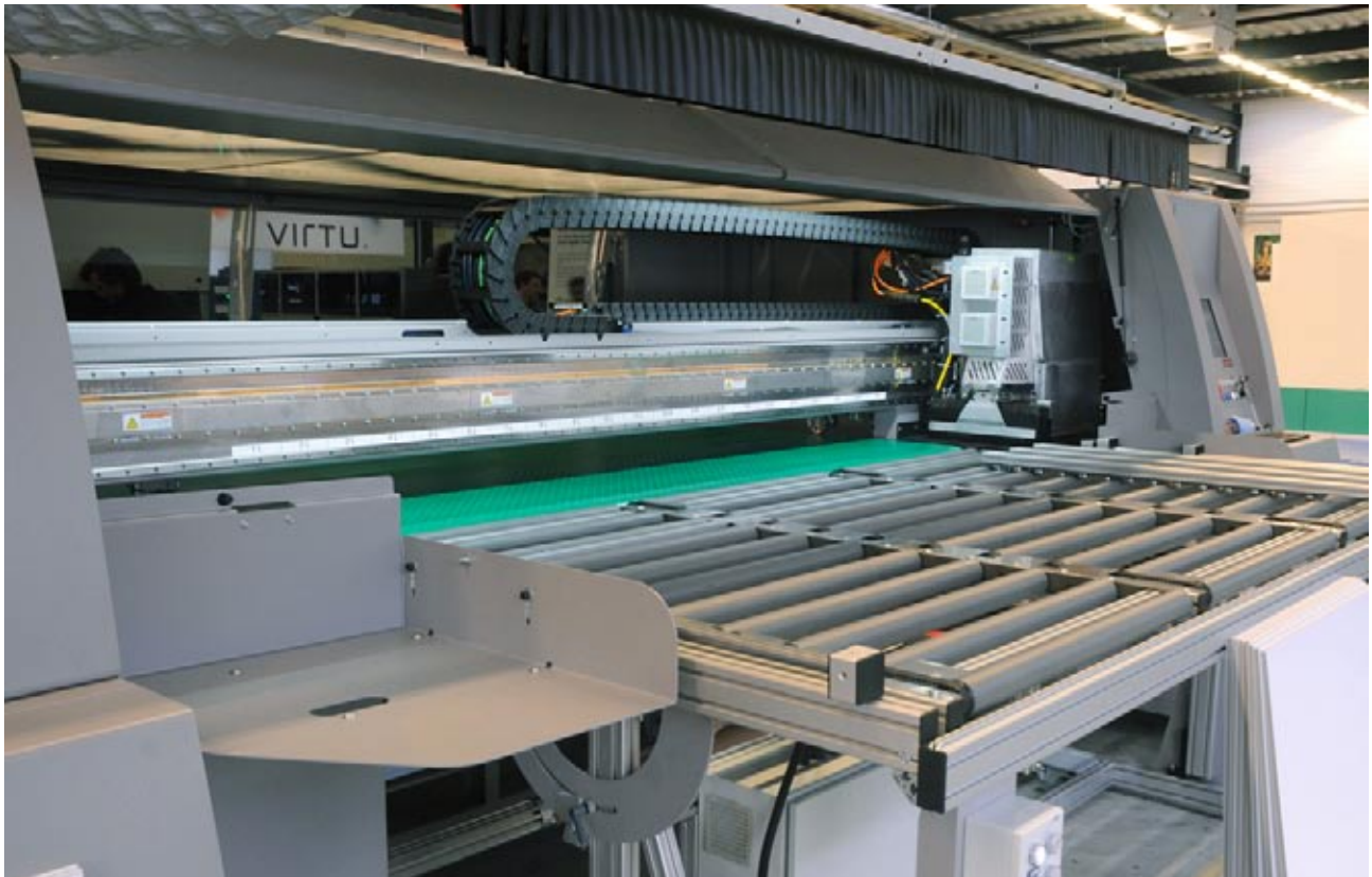
RS25/48 front view of special table for feeding multiple boards simultaneously. Complete workflow for board printing.
