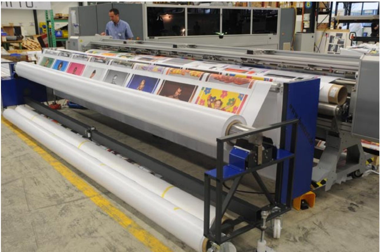
This is the Fotoba XXL 500 xy cutter, an intermediate step in the workflow.
