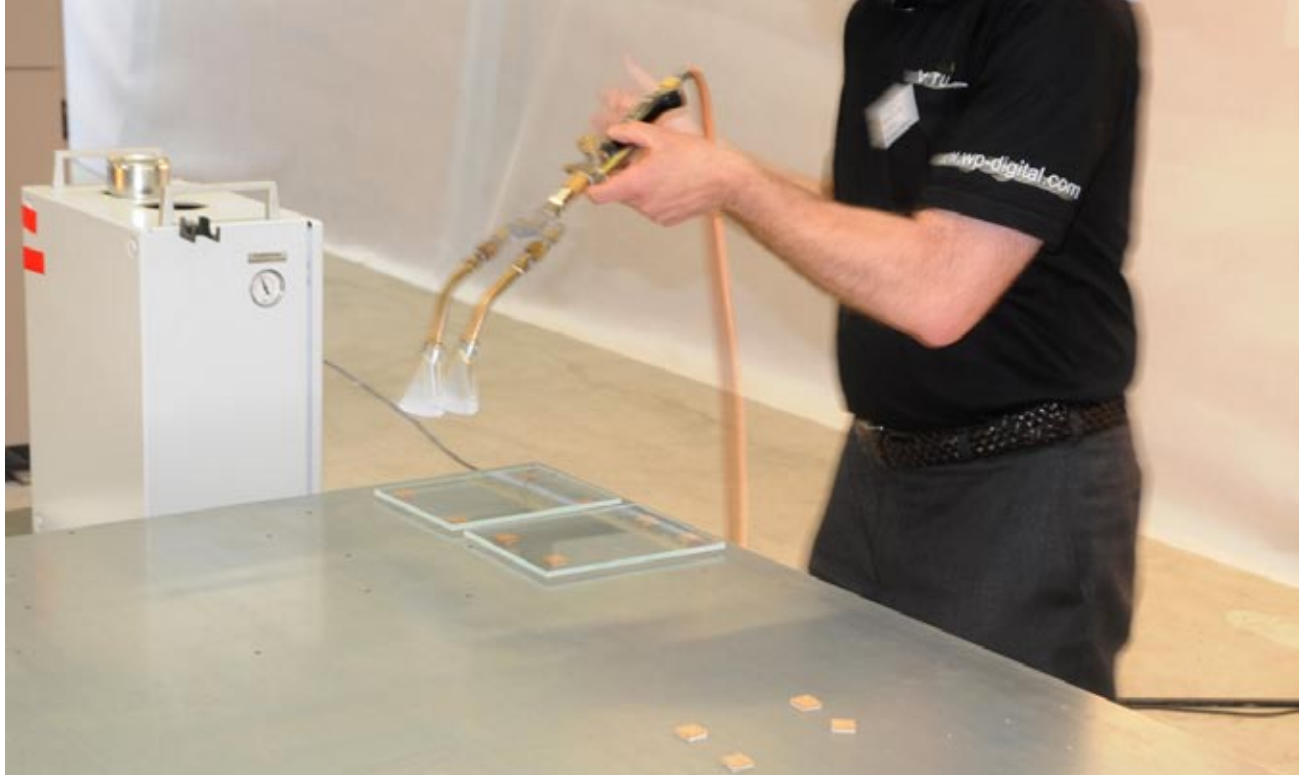
Second step in glass preparation, flame treatment done by Norbert Steinmann.
