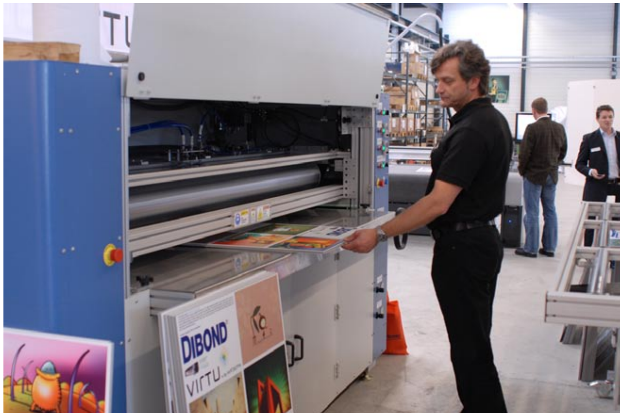
Printed boards: increased durability and scratch resistance by laminating.
