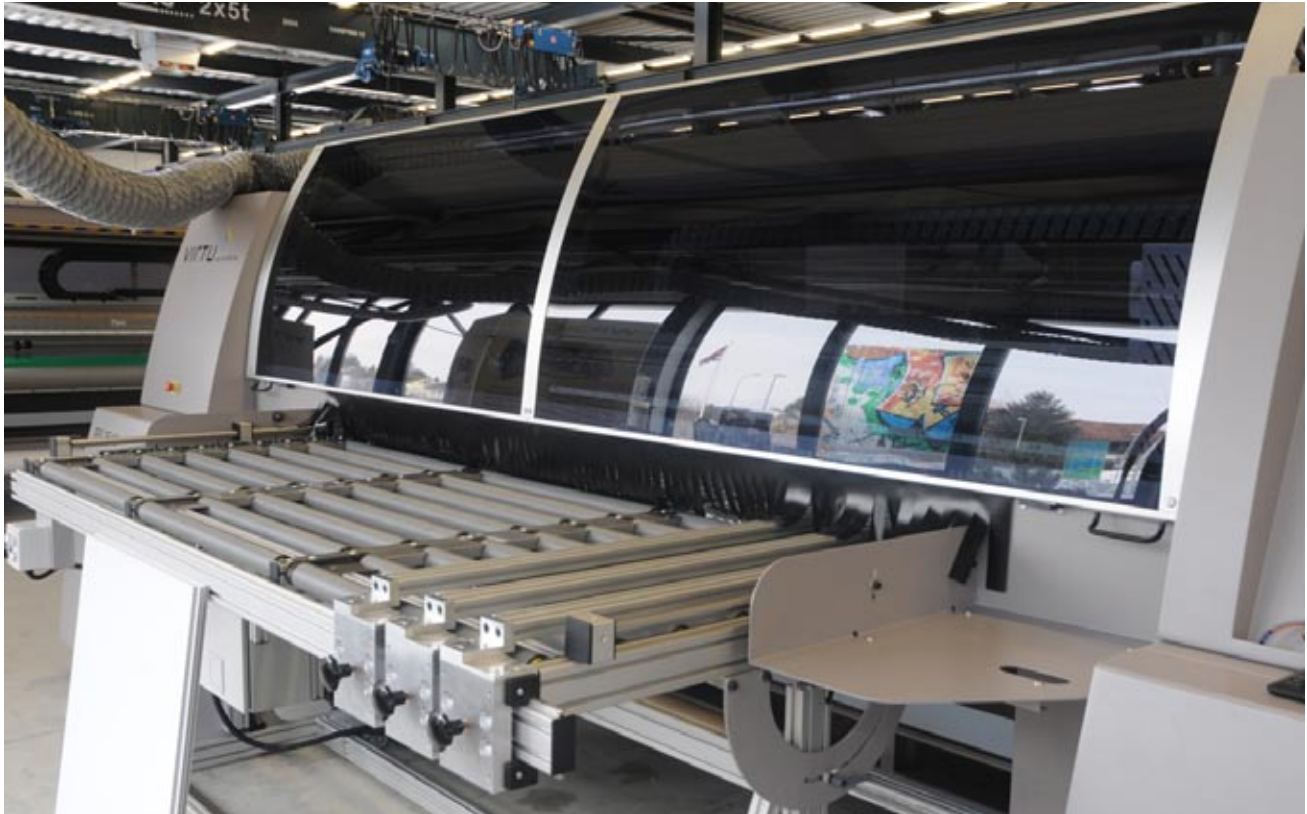
RS25/48 front view of special table for feeding multiple boards simultaneously. Complete workflow for board printing.
