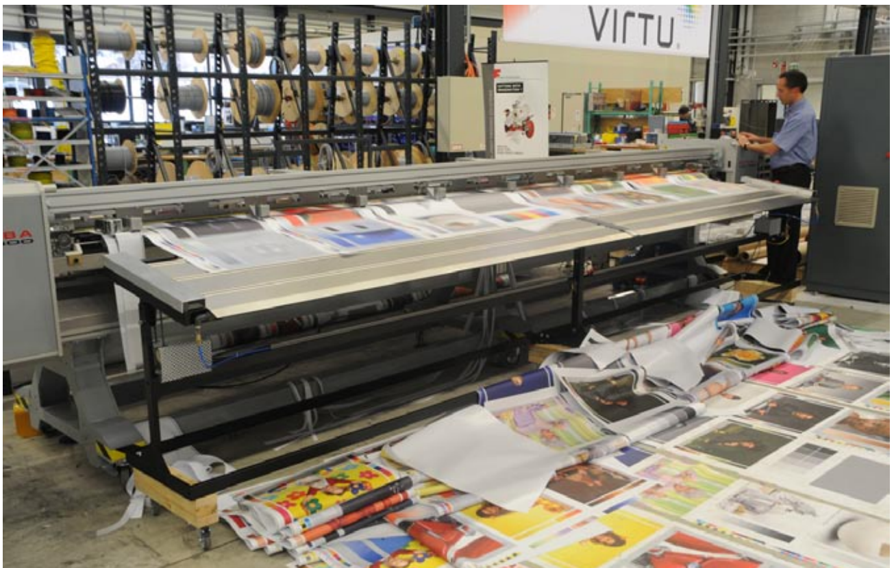
Here you can see the new Fotoba XXL 500 xy cutter. They showed how you can cut longitudinally or crosswise directly after printing in the future.
