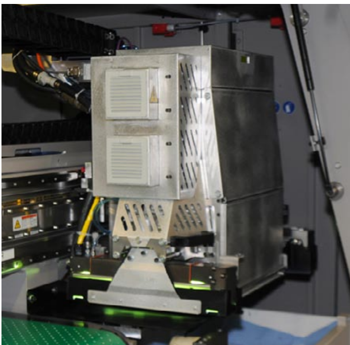
Water-cooling carriage for the UV lamps, at WP Digital factory 08
