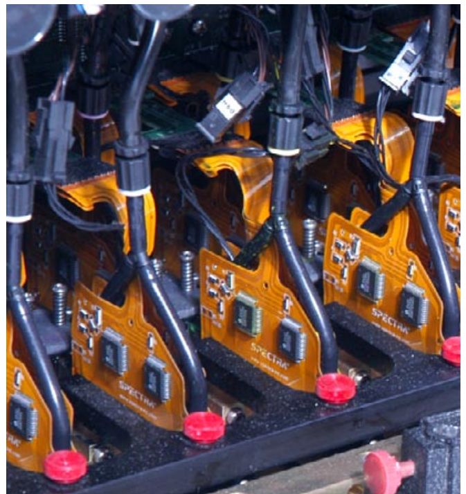
Brand and model of printhead determine the drop size of your printer. Achievable resolution will also vary from printhead to printhead.
