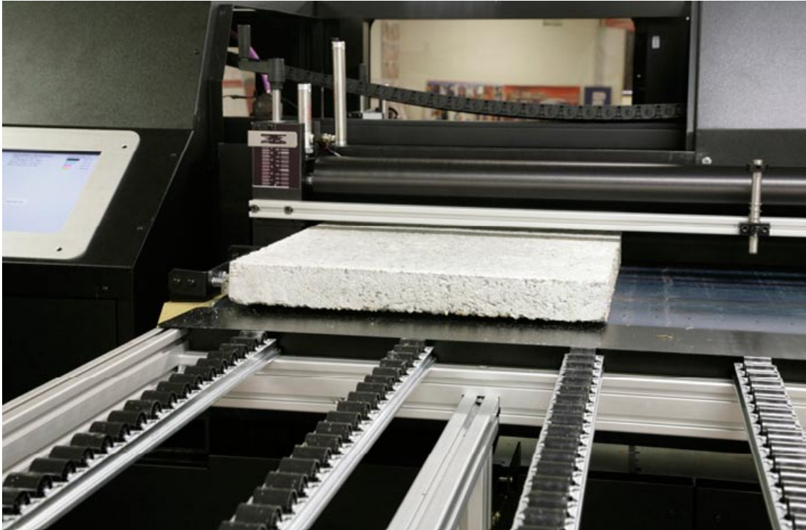
Horizontal bars with rows of rollers on the ColorSpan 9840uv.
