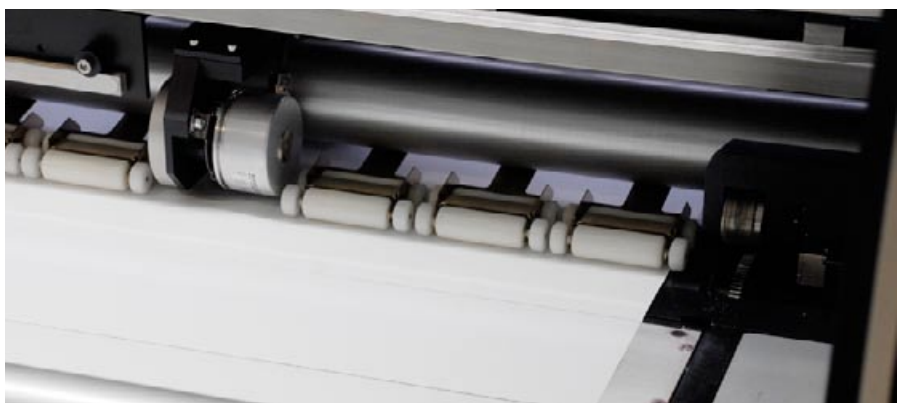
Although this printer was called Zund 250 Combi, it is actually a hybrid printer. In the lower photo you can see the pinch roller system.
