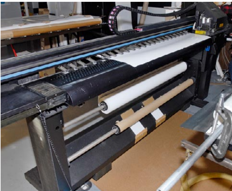
The ColorSpan 72uv series were hybrid printers. Most hybrid printers were solvent printers that were retrofitted to handle UV ink. As you can see in the photo at right, a table is incorporated to handle boards. This ColorSpan hybrid was a very successful UV printer, but most UV machines of this type of feeding mechanism tend to have problems with rigid media.
