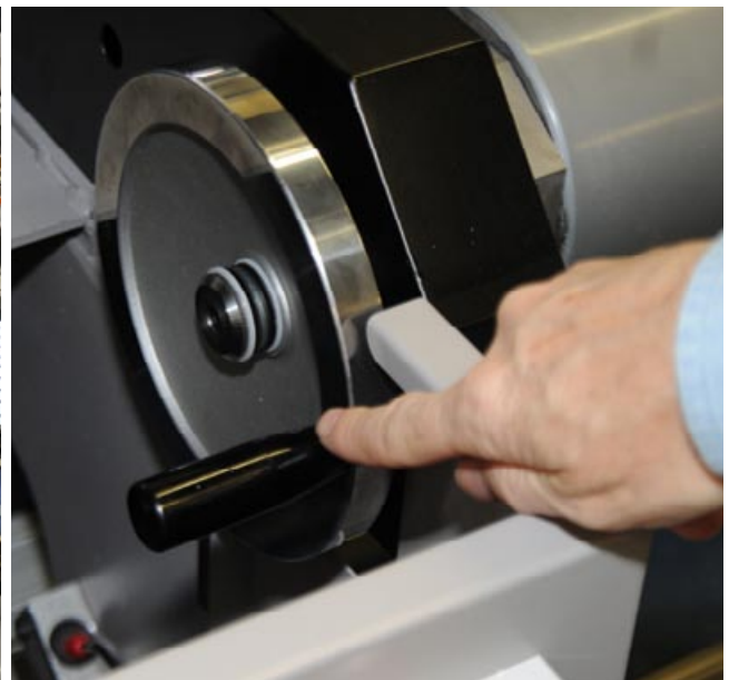
Besides the ability to handle traditional rigid and roll-fed media, it has a trough (e) to capture ink if you need to print on textiles, mesh or similar media. The photo at right shows the handle to move the trough upwards and downwards.
