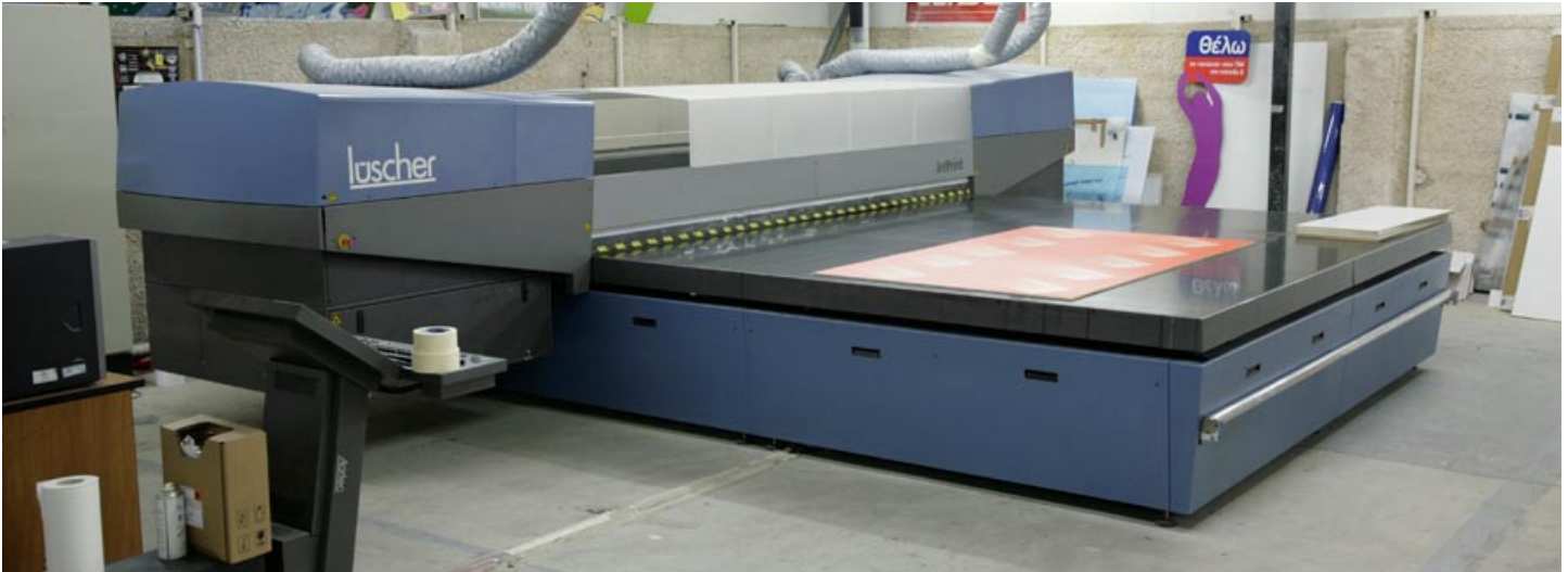
The Luscher JetPrint 3530 is a dedicated flatbed. It handles only rigid media. This printer attempted to use LED curing before it was mature technology. Plus this company had never made a UV-cured inkjet printer before. The printer was also simply too large, and too difficult to service. After a few sales even the manufacturer realized this printer was not a success (clearly they read the FLAAR Reports). Finally this entire project was abandoned. So before you buy from a printer in this price range, be sure that the UV manufacturer intends to stay in business and can continue to provide tech support during the entire 3 to 5 year life of the printer.
