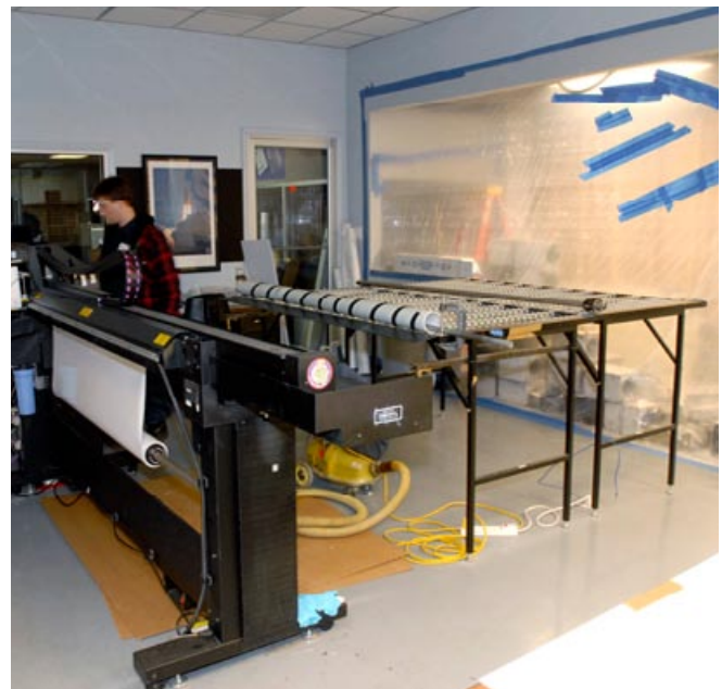
The ColorSpan 72uv series were hybrid printers. Most hybrid printers were solvent printers that were retrofitted to handle UV ink. As you can see in the photo at right, a table is incorporated to handle boards. This ColorSpan hybrid was a very successful UV printer, but most UV machines of this type of feeding mechanism tend to have problems with rigid media.
