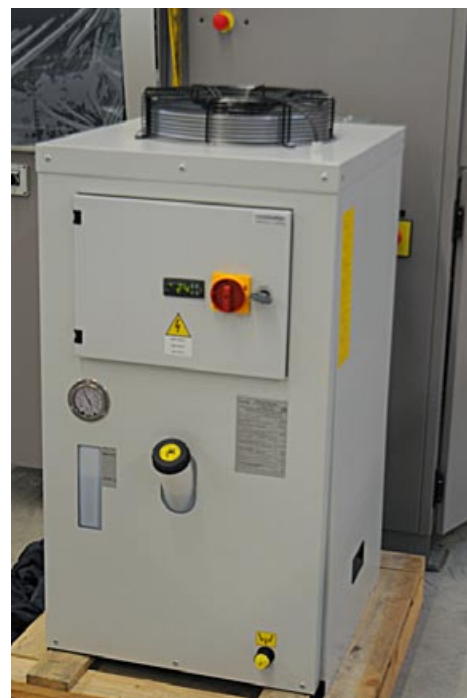
UV lamp cooling, at WP Digital factory 08
