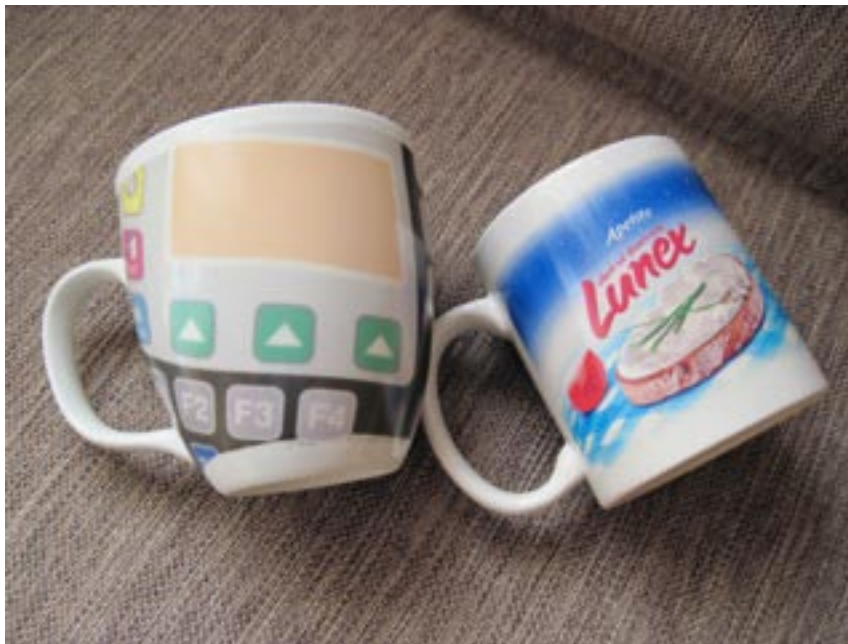
A special film printed with Sepiast inks was stoved into a ceramic part. This was done by low temperature stoving with 220°C.
