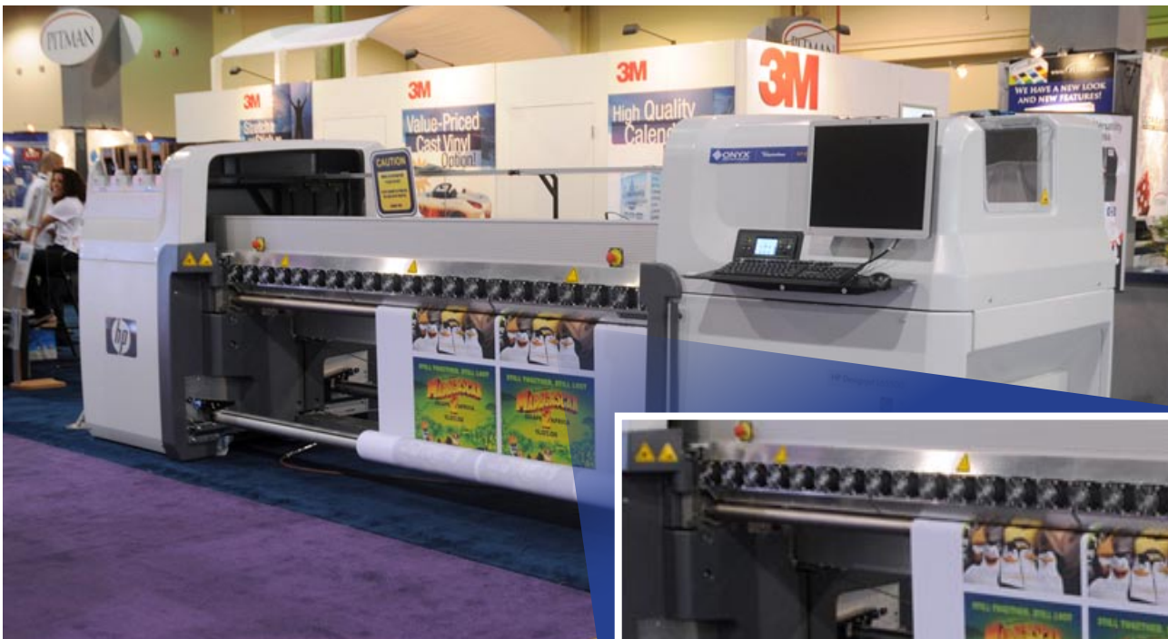
HP Designjet L65500 printer, at ISA 09. In the exploded view you can see that this printer is a dedicated roll-to-roll (handles only flexible media) like all latex printers at the moment.
