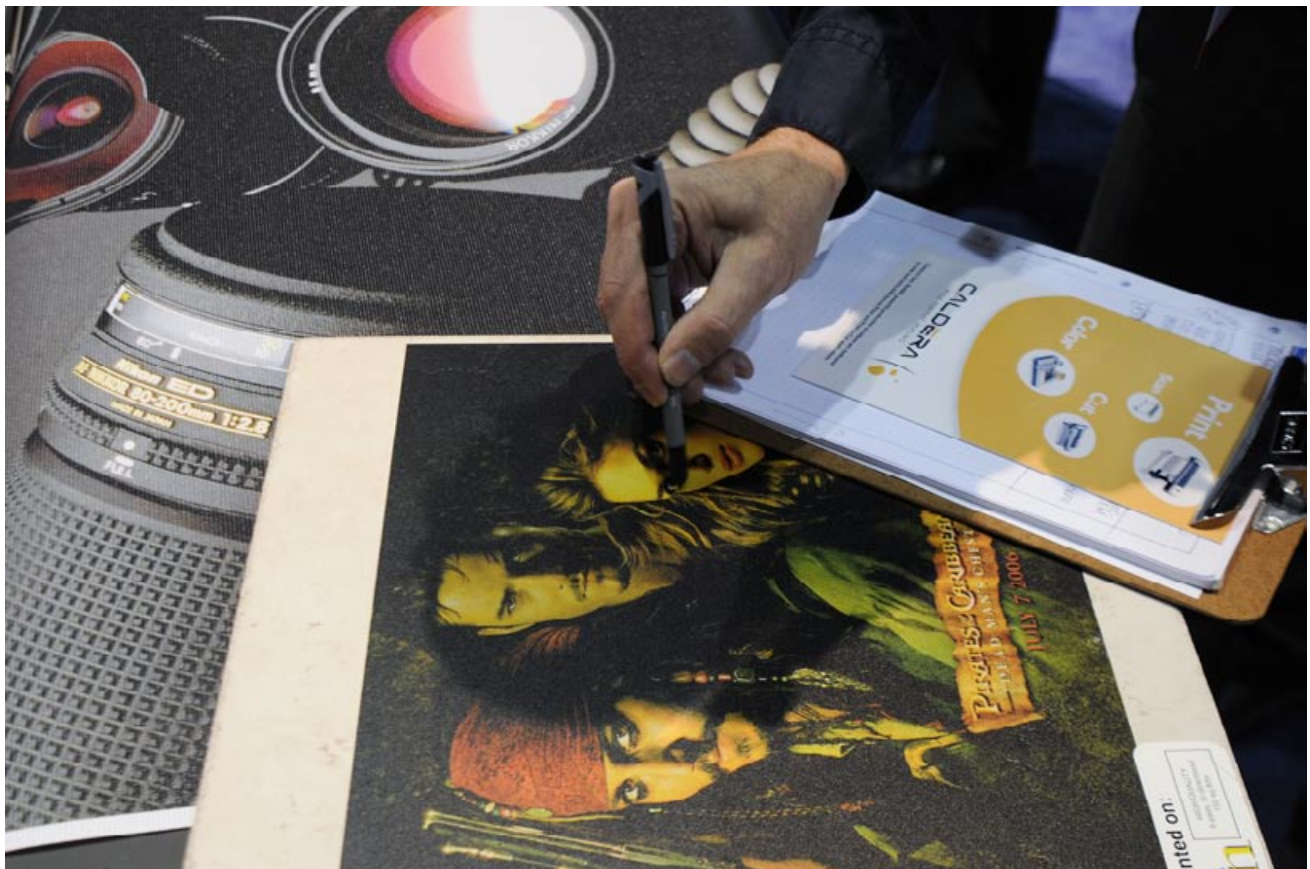
Adhesion and scratch resistance are some of the aspects being evaluated by FLAAR to determine the quality of the UV ink used by a printer. In this photo, Dr. Nicholas Hellmuth is testing a print sample with a ballpoint pen.
