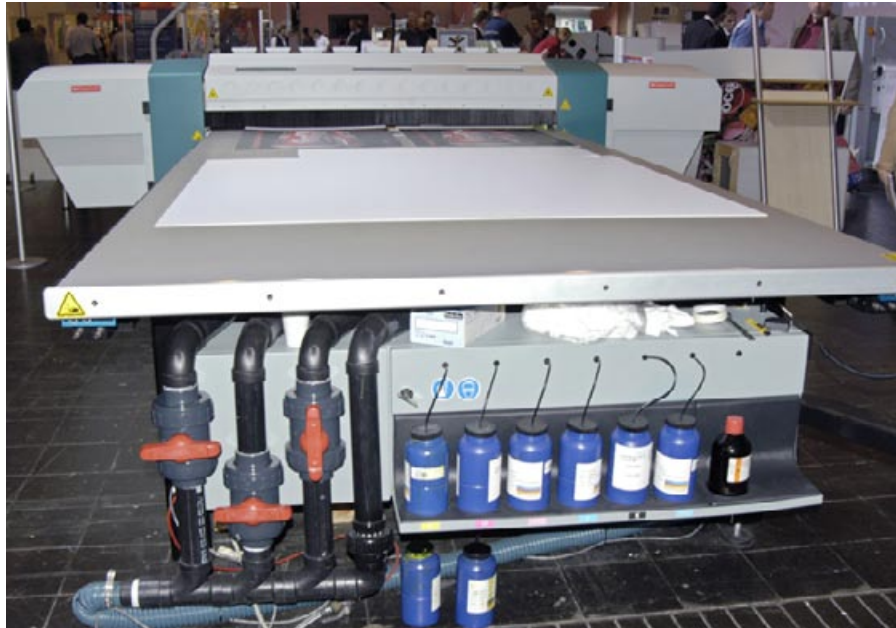
The Océ Arizona 220 was designed as a dedicated flatbed (only to print rigid materials), without the roll-to-roll option.
