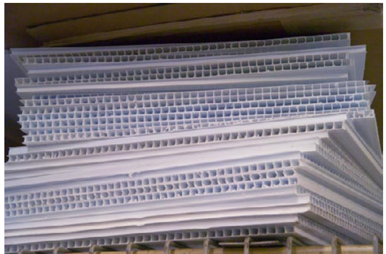
Coroplast is one of the substrates that requires pre-treatment with at least one major brand of UV ink. With this one brand of ink, unless Coroplast is pre-primed by hand or spray in your shop, the ink will tend to fall off the Coroplast in a few weeks (if not sooner).
