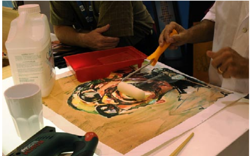
Here you can see an example of how some materials need to have a top coat after printing on them to avoid ink fall off.
