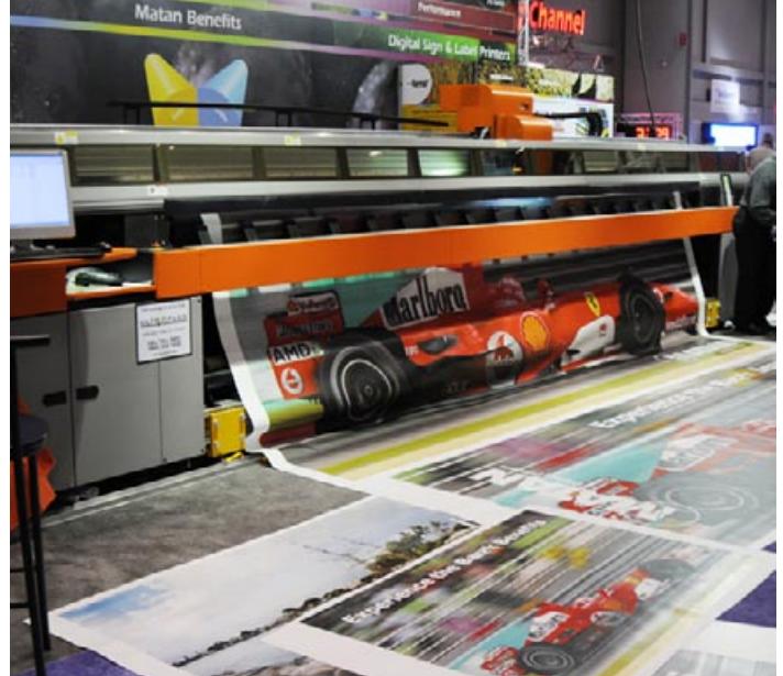
The ink of the Matan Barak5 UV printer is formulated to print on roll-fed media but it also handles rigid media.
