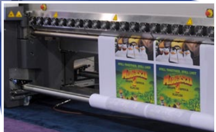
HP Designjet L65500 printer, at ISA 09. In the exploded view you can see that this printer is a dedicated roll-to-roll (handles only flexible media) like all latex printers at the moment.
