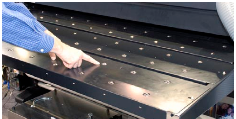
The tables that are necessary for UV hybrid printers have various design concepts to move rigid media into the enclosed printing area. You can have cylindrical-shaped rollers inset into a flat table, or spherical-shaped rollers set into a flat table. Most tables though are made of many parallel rows of roller bars.
