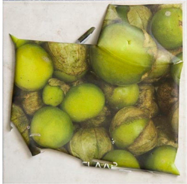
Floor tiles were printed on as part of a FLAAR evaluation in the Gandinnovations UV printer manufacturing plant. Months later one of the floor tiles had begun to peel off (in part because it had been put on top of a mini kitchen oven).
