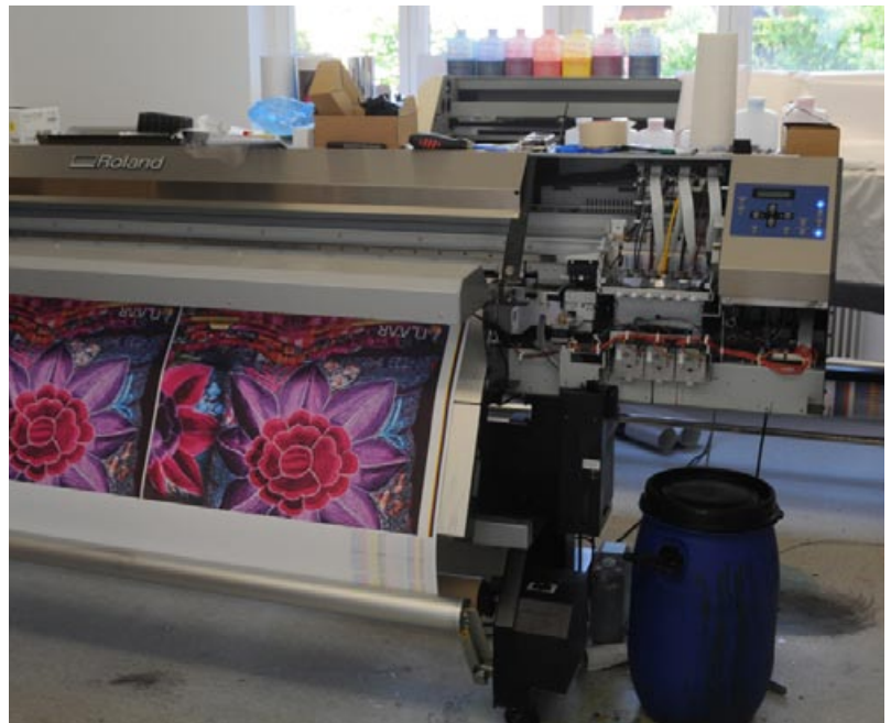
Sepiax ink being used in a Roland printer in the R&D facilities in Austria. Here Sepiax ink is printing directly onto uncoated canvas paper.
