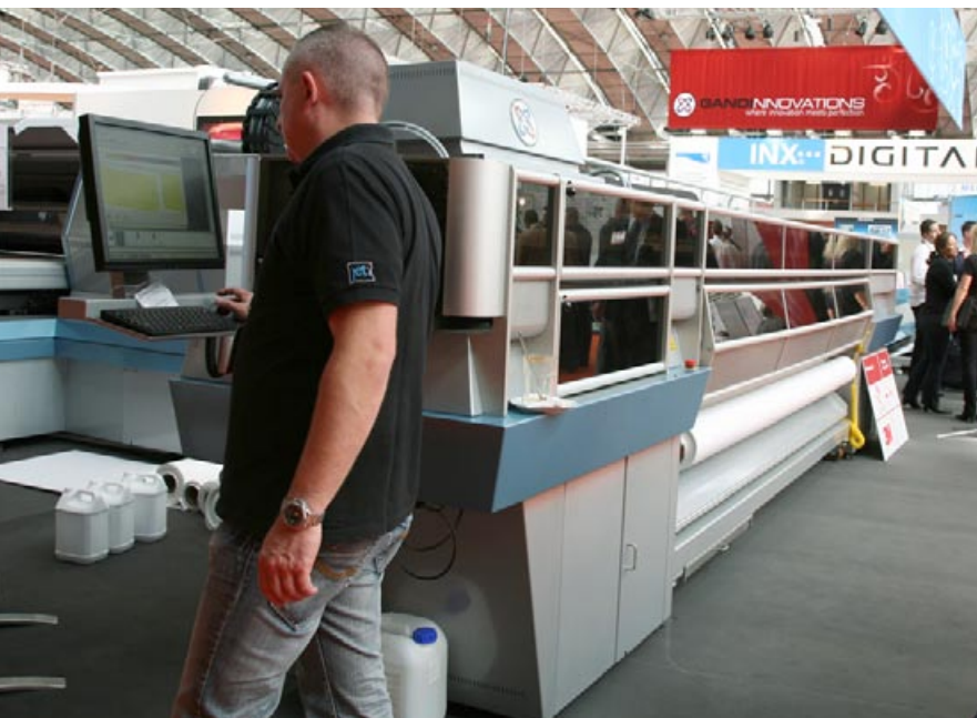
It is advisable that a UV printer be attended at all times by an operator. Here the Gandinnovations Jeti 3348 UV JetSpeed at FESPA Amsterdam '09.
