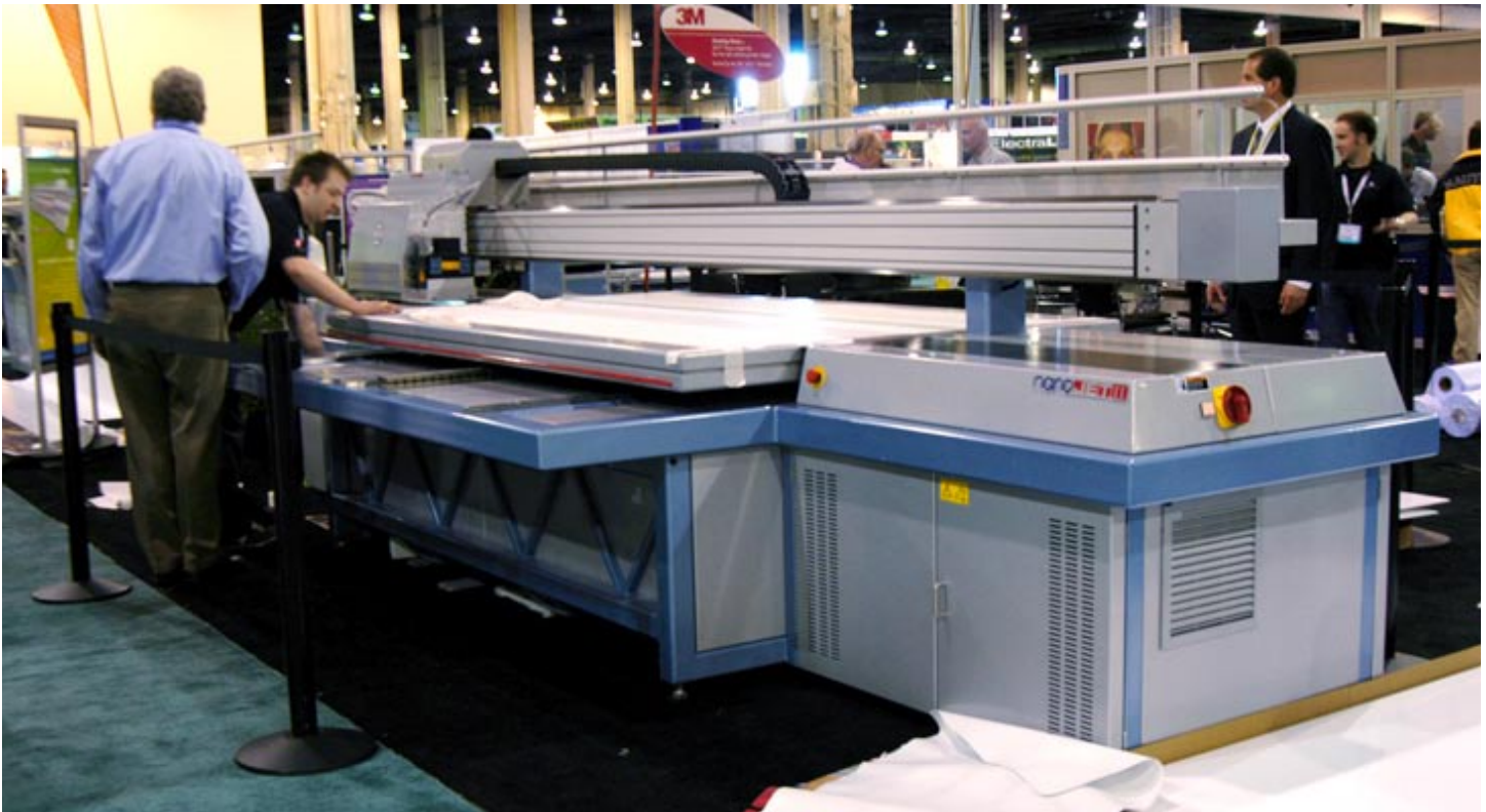
Gandinnovations Jeti 1224 Nano Jet II at ISA'09. The Jeti printers have traditionally used Spectra heads, but this newer model uses Ricoh heads to produce a higher quality.
