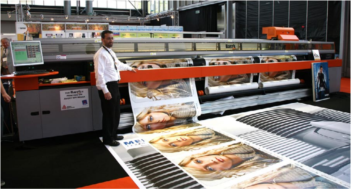
Matan Barak roll-to-roll printer at FESPA '09. This is one of the UV printers that uses Ricoh heads.
