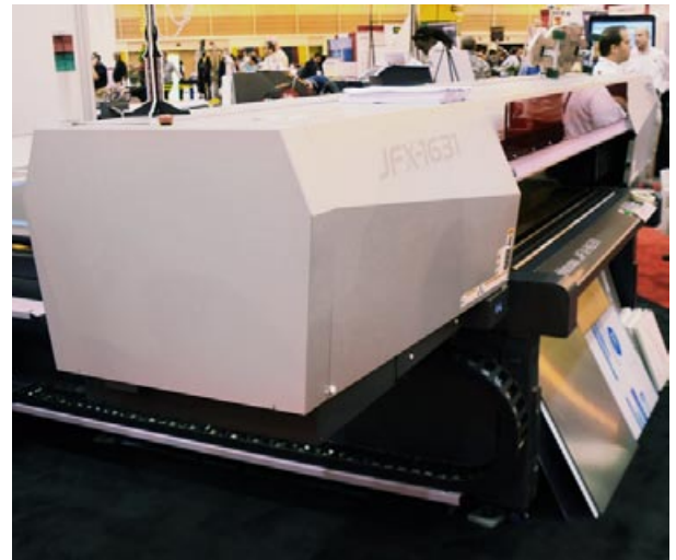
The Mimaki JFX-1631 is replacing the JF-1631 printer. This new model uses LED lamps, but it continues to use Toshiba Tec heads.
