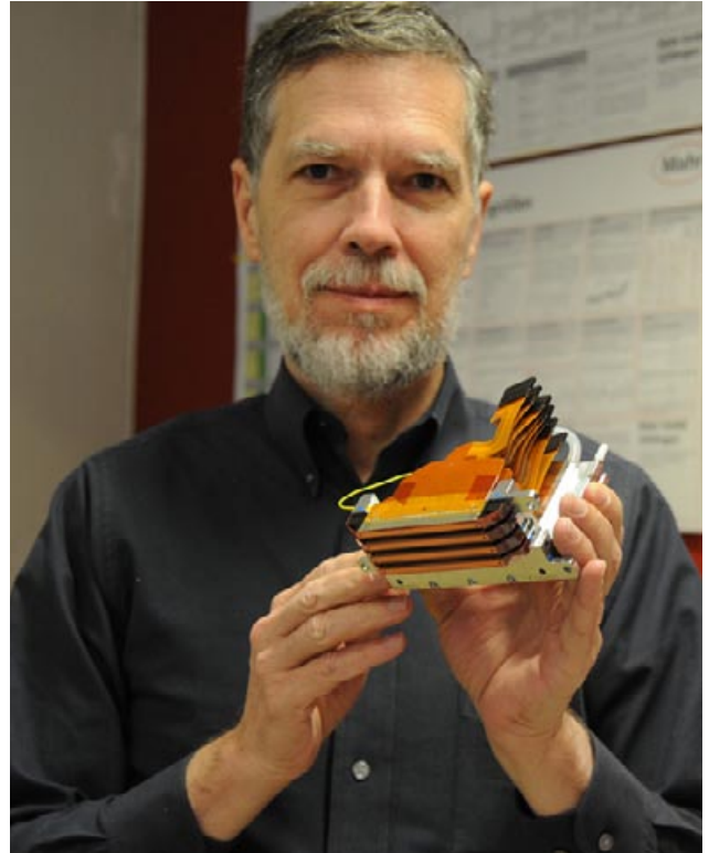
Dr. Hellmuth holds a Quadro Array system based on Spectra printheads at the Durst factory in Lienz, Austria.
