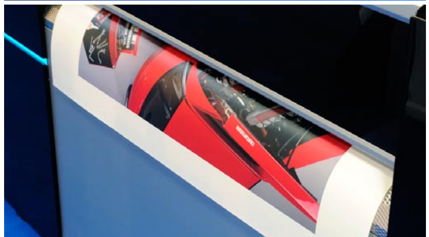
Konica Minolta KMIJ-X UV printer at DRUPA '08. This prototype came with CMYK inks and cured with LED lamps.
