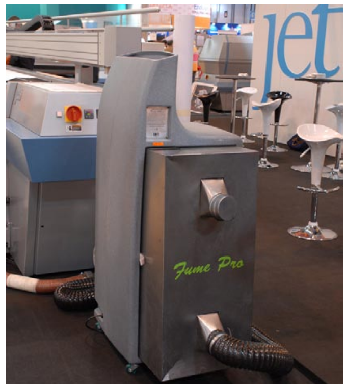
The Island Clean Air, Fume Pro is an attachment that provides source capture and ambient air filtration.
