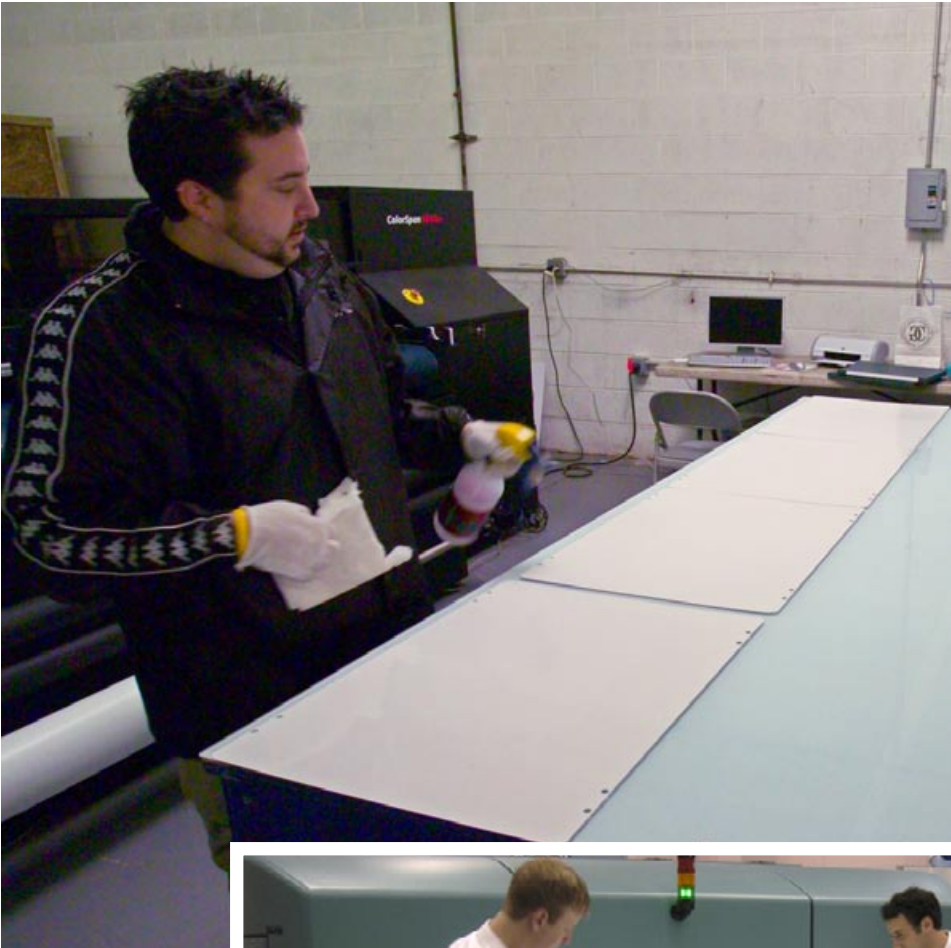
Most print shops use ISP alcohol. However alcohol (if not totally dried and wiped off) can leave a smear which shows up as an actual smear pattern when the ink is printed on top of it.
