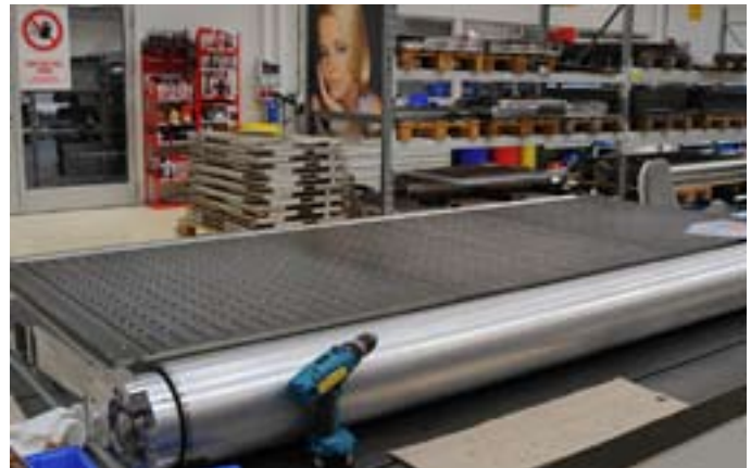
Durst Rho 800 UV printer at Lienz factory. You can see the grill on top of which the transport belt will be placed.
