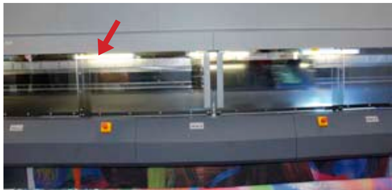
Fluorescent light inside the hood
