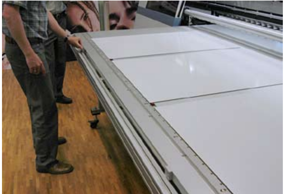
Zund 250 UV printer at demo room. Alignment of the flat rigid material
