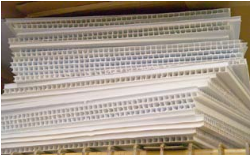
Coroplast is one of the most common rigid substrate to print in flat printers
