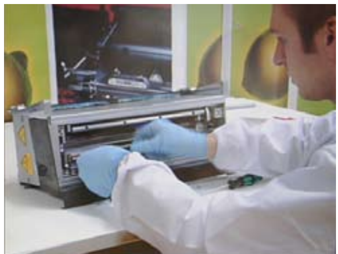
Durst Rho 351 UV lamp, being cleaned
