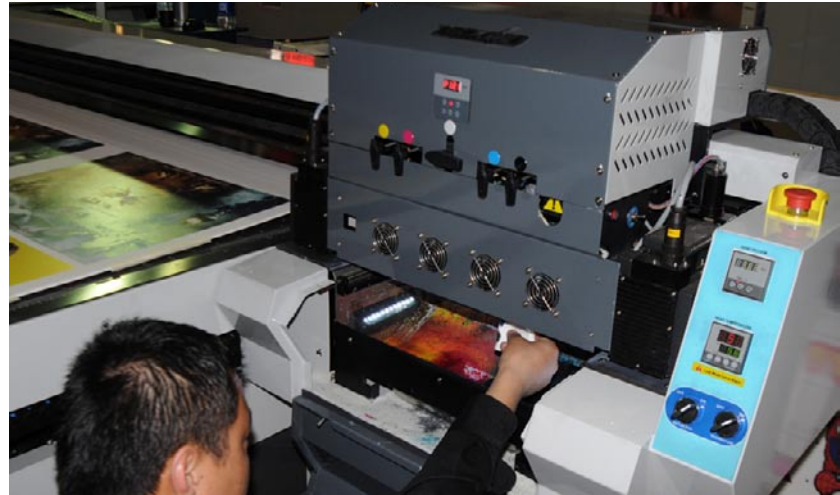
The service station of the Teckwin TeckStorm UV is at the right.
