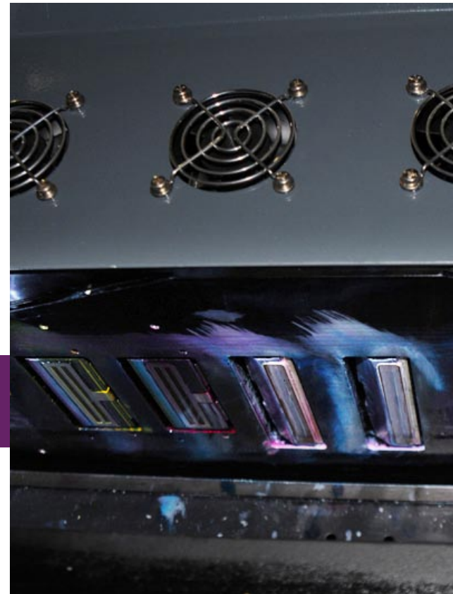
This photograph shows a printhead carriage taken from below. Since printheads are set in a vertical position, negative pressure is needed to keep the ink from dripping out of the heads.
