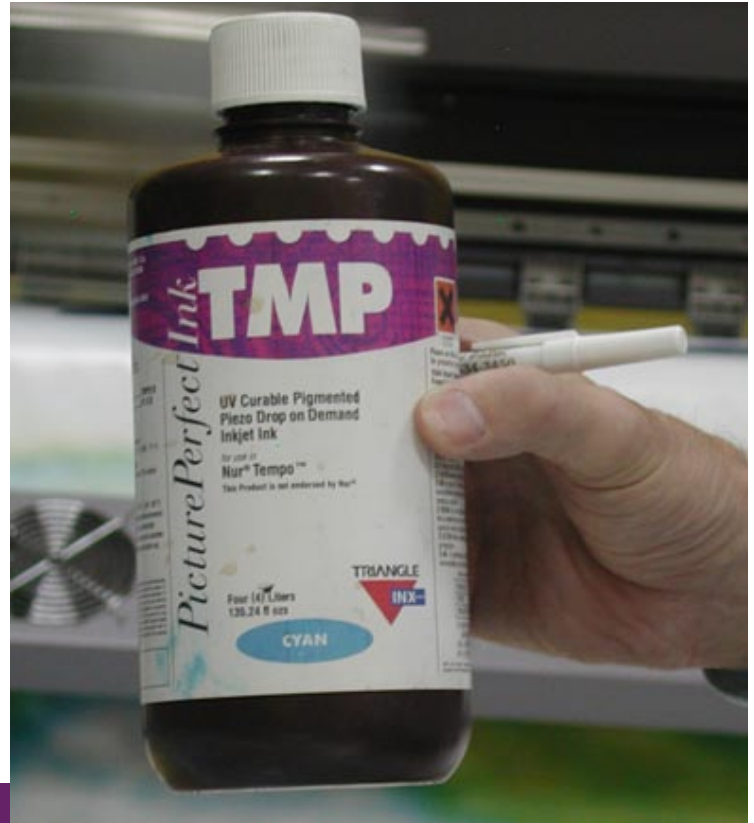
UV ink bottle of an Infiniti UV hybrid printer.
