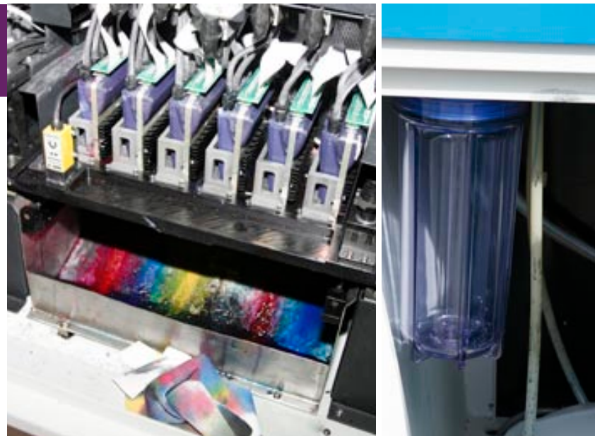
Waste ink goes into a drip tray, and then into the waste ink container. Teckwin TeckSmart 1600 UV.
