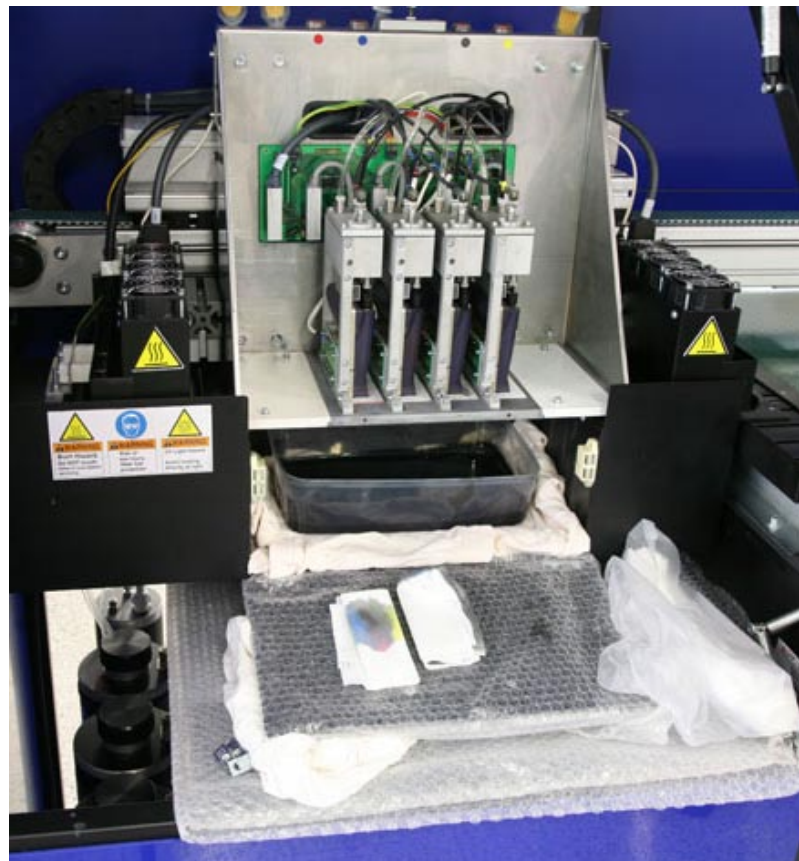
When the printheads purge ink out, it generally goes into a drip tray placed below the printhead carriage in the service station. In the photo, the first generation of the Grapo Octopus purging ink.
