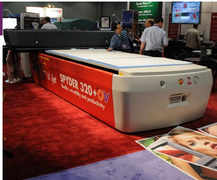
Inca Spyder 320+OV UV printer at ISA '08. Inca has a long tradition of UV-cured flatbed printers.
