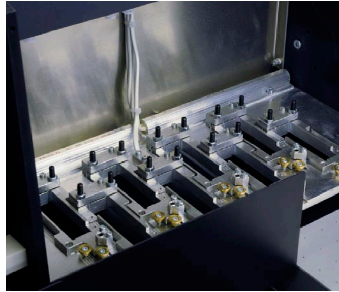
Nozzle plate of the Grapo Octopus UV printer. Printheads are going to be placed in the holes you see here.
