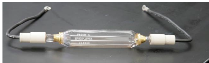
The VUTEk printers use mercury arc lamps.
