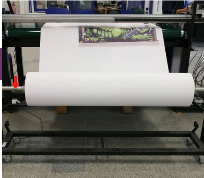
Once printed on, the roll-fed material is collected on the take-up reel. Grapo Octopus UV printer at Grapo factory visit.
