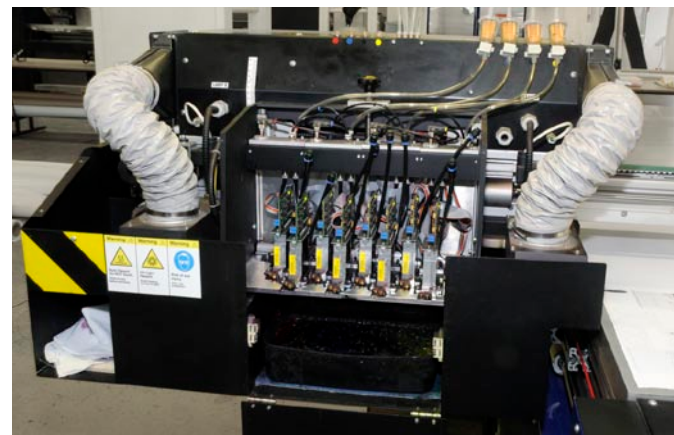
Printhead carriage of the Grapo Manta UV flatbed printer.
