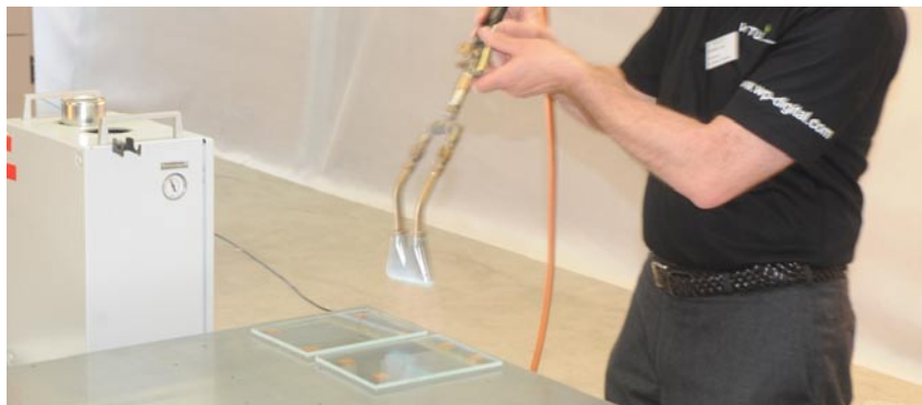
Flame treatment for pieces of glass that will be printed on a UV machine.
