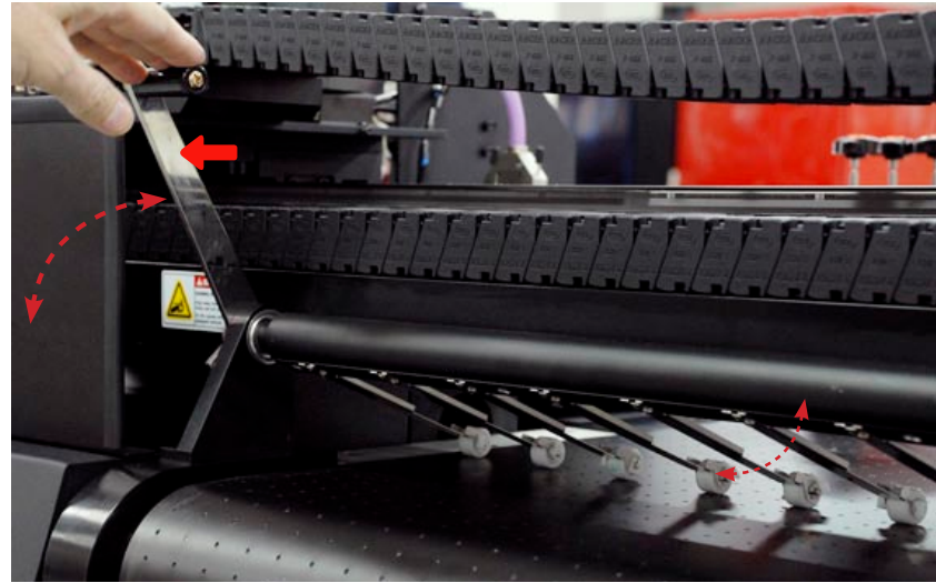
An example of pinch rollers on the IP&I 1606 CUBE UV combo printer. Pinch rollers can be raised or lowered by a lever, but some complex printers move their pinch rollers electronically.
