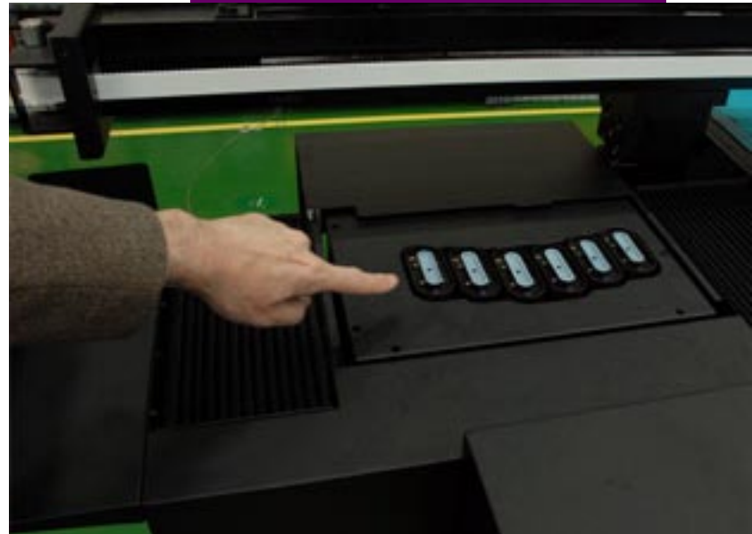
Dilli Neo Titan capping station. Heads are covered by lowering the print-head carriage. Dilli factory visit, 2008.
