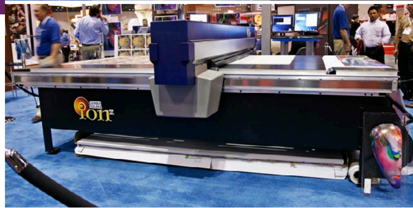
Above, the Inca Spyder 150uv at FESPA 07. Below, the Gerber Solara ion ® at SGIA 07. As you can see, both models are designed with a gantry which houses the printhead carriage. The latter model uses cationic cured ink.
