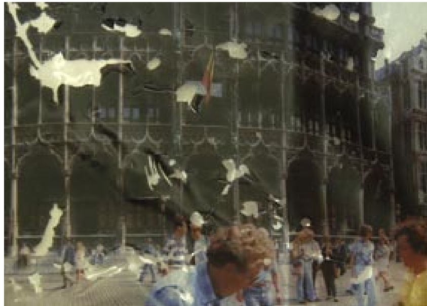
This is an example of how the ink begins to flake off, when adhesion is bad.
