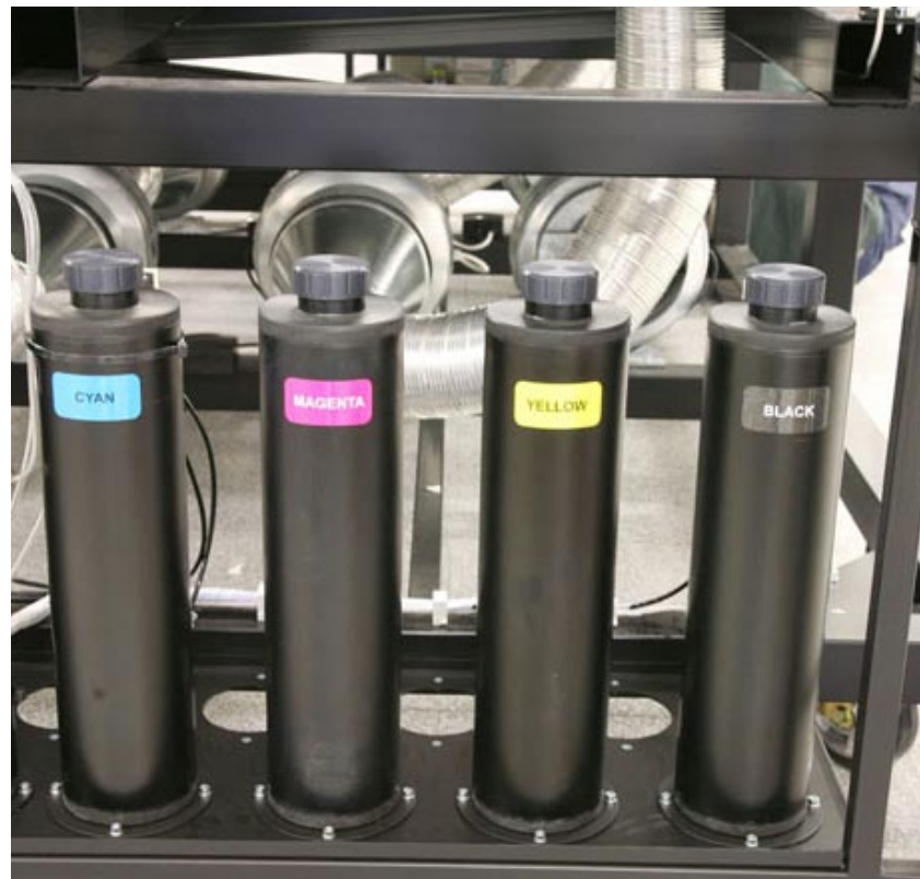
UV ink containers of the Grapo Manta UV dedicated flatbed printer. As you see, most containers, hoses and tubes are dark because UV ink is sensitive to sun light.
