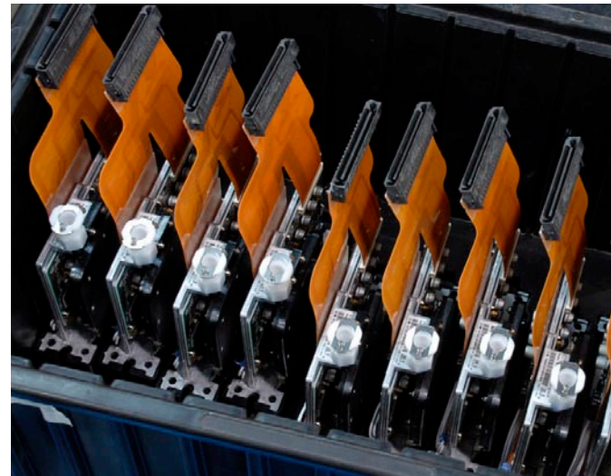
Printhead set ready to be installed in a VUTEk 320/400 FC+. VUTEk factory visit, 2008.
