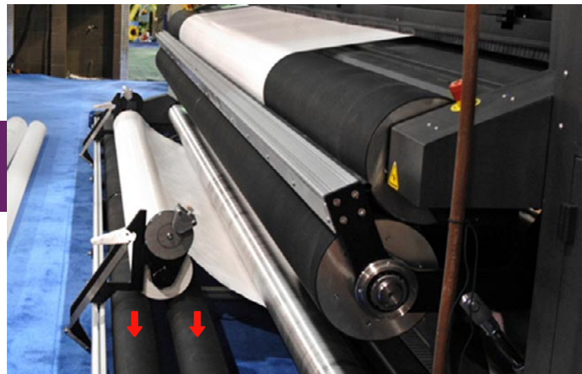
The efi VUTEk GS5000r holds the roll in a saddle. This is common in 5-meter roll-to-roll printers since the long rolls would tend to sag.
