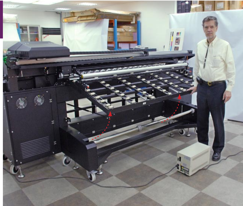
The GCC StellarJet 183uv is a hybrid printer. You can see the table that is pulled up for flatbed applications. But it can be lowered for roll-to-roll option.
