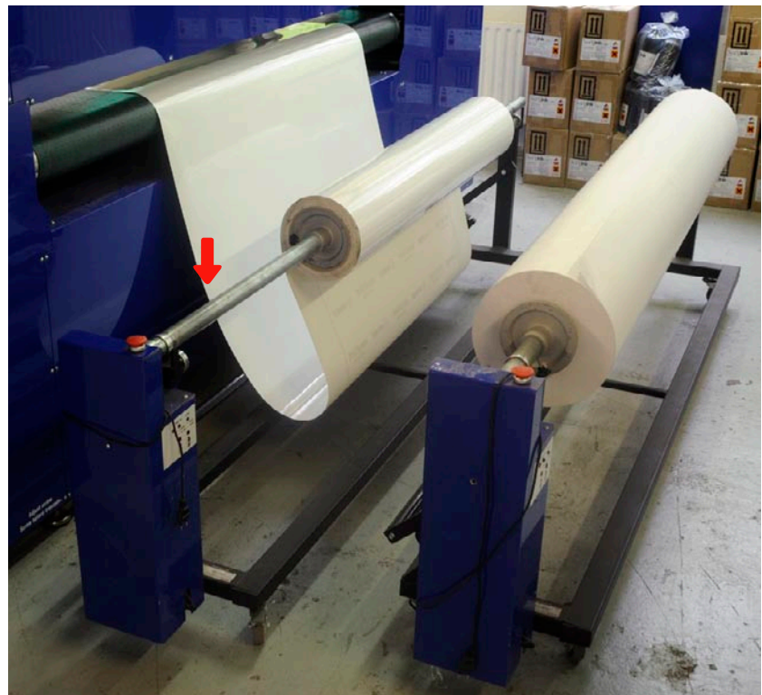
The spindle of a Grapo Octopus UV printer. Some feeding systems are physically attached to the printer. In the case of the Grapo Octopus the feeding spindle is a component that can be wheeled away.
