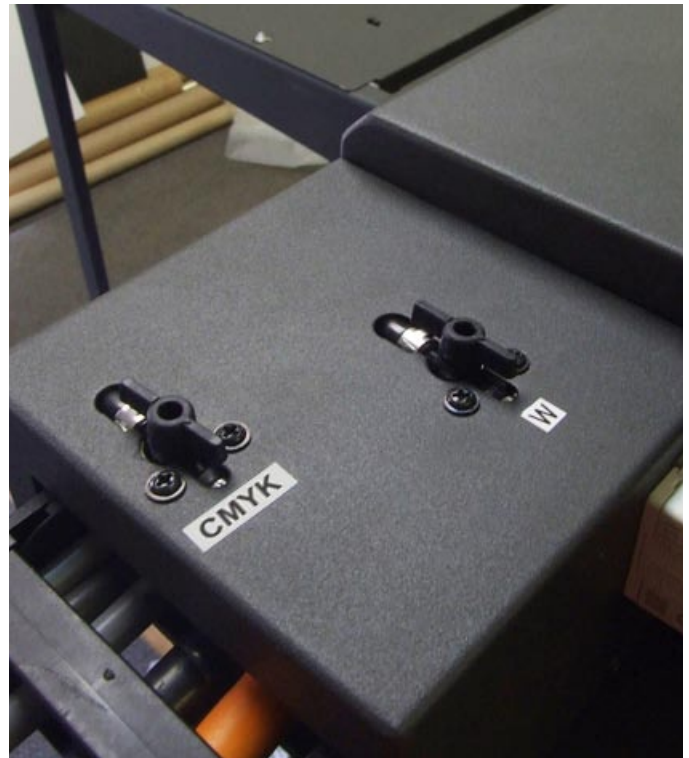
In the EFI Rastek H650, even the purging system for white is independent of the CMYK channels.
