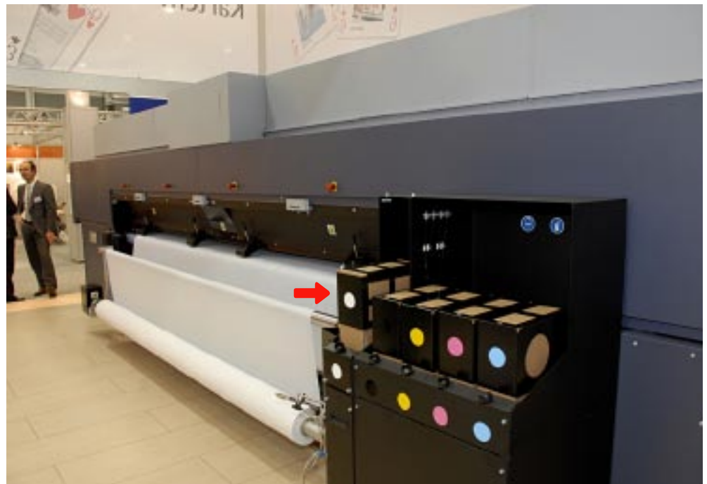
Durst Rho 351R. The white ink is at a different level than the rest of the inks.
