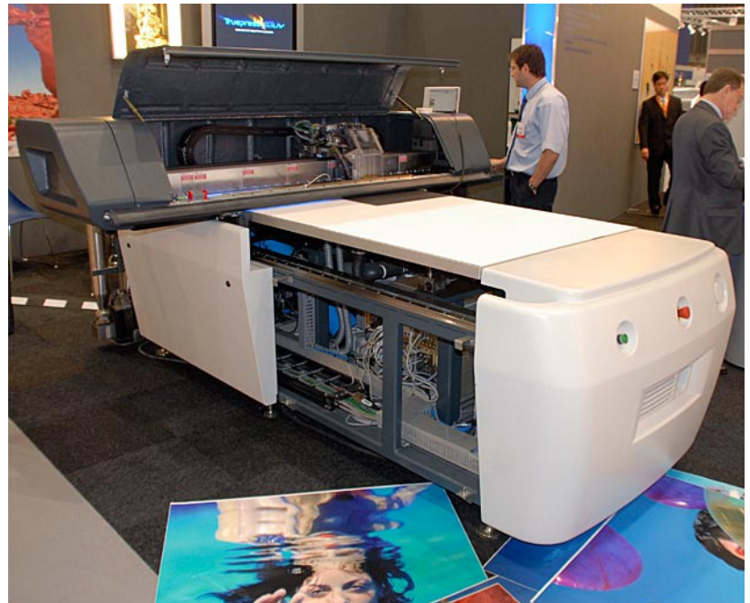
Inca Spider 150 UV at FESPA 07. This printer uses the LED lamp technology for the process of curing the ink into the media.
