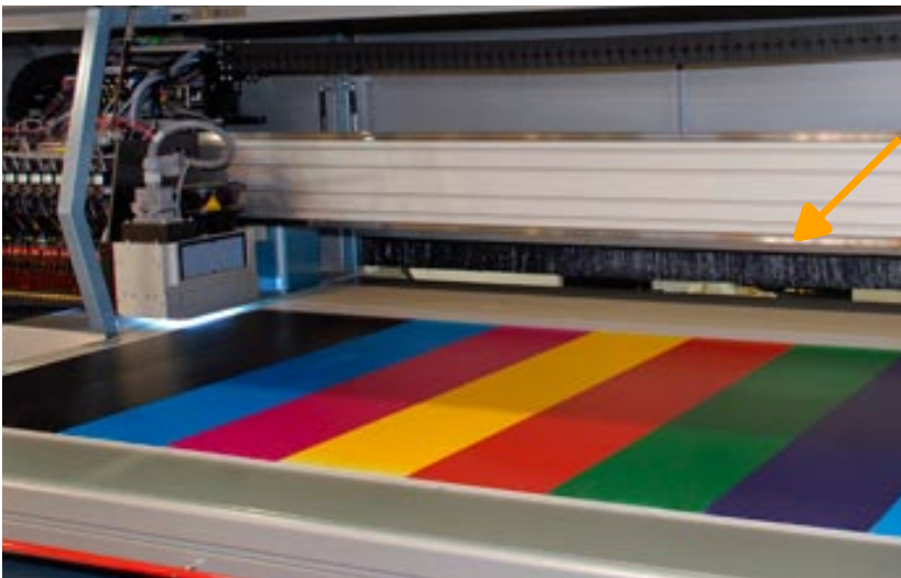
Process of printing. The UV light is curing the ink.
