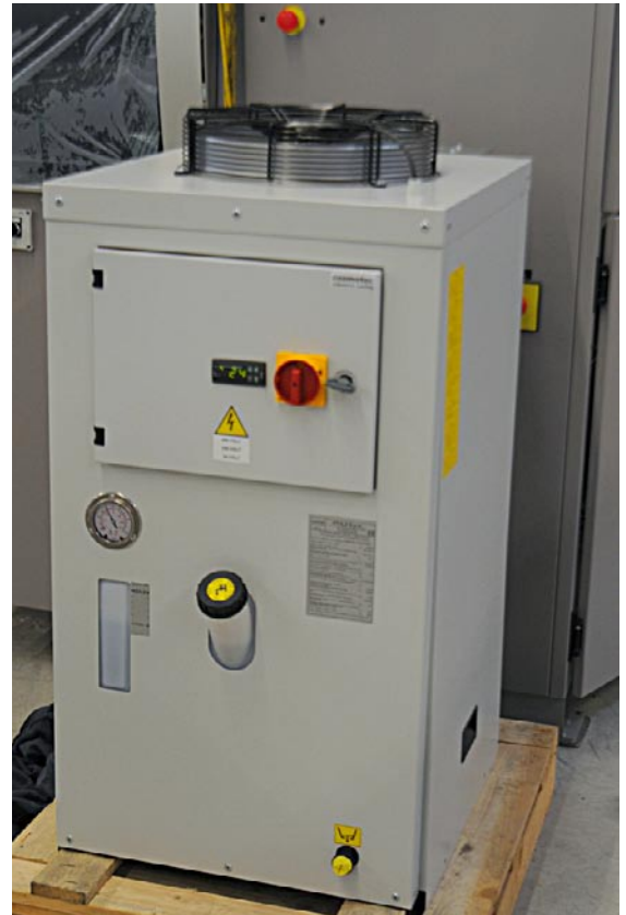
UV lamp cooling, at Spuhl factory 08
