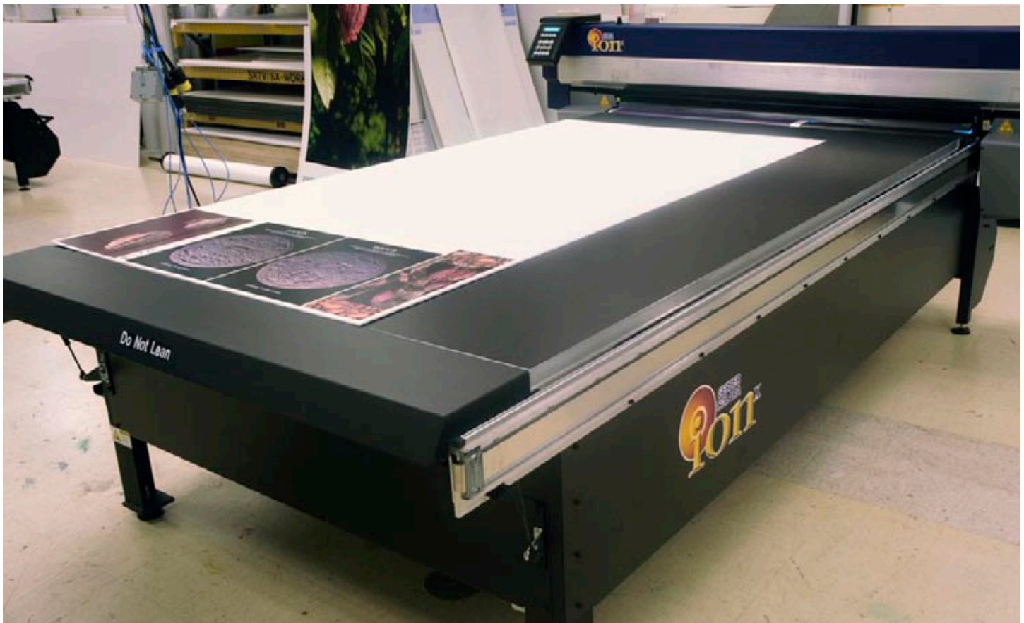
Testing the Gerber Solara ion X for hours inside the factory demo room. The ion x can print rigid materials up to 1" thick.
