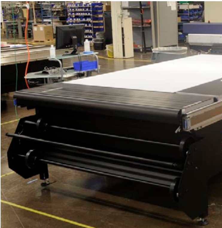
The original printer was conceived with the roll-to-roll option from the beginning, therefore, it is physically attached to the printer.
