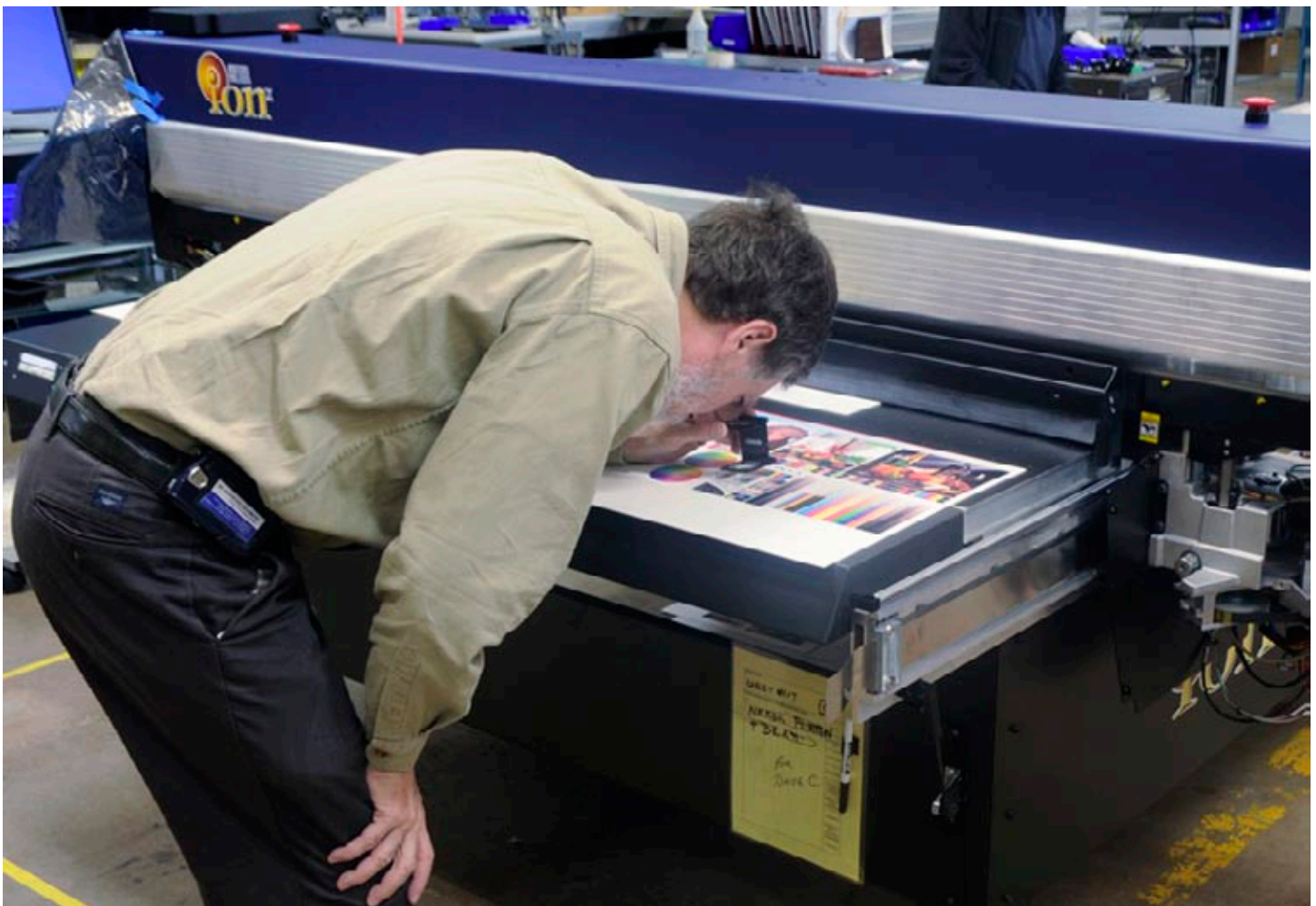
Dr. Hellmuth at the Gerber factory evaluating the quality of the printed samples. Drop size and color gamut are some of the aspects considered in our evaluations.
