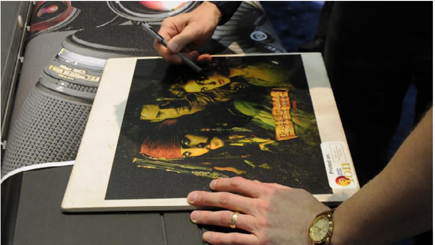
Another aspect evaluated is adhesion. Here, Dr. Hellmuth scratching a print sample with a pen at ISA 08.
