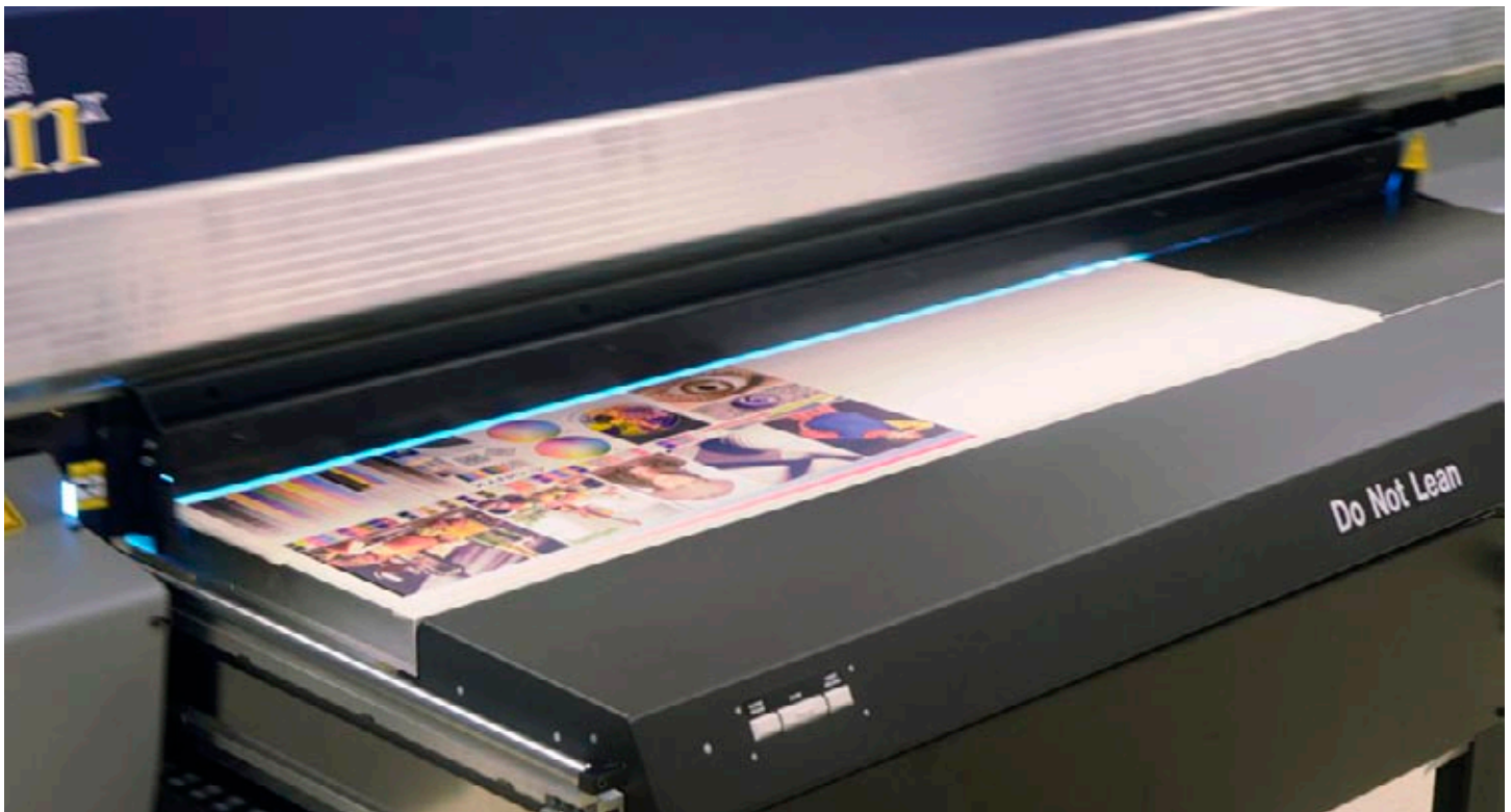
The light you get to see in the edge of the gantry shows that the lamp covers the print width.
