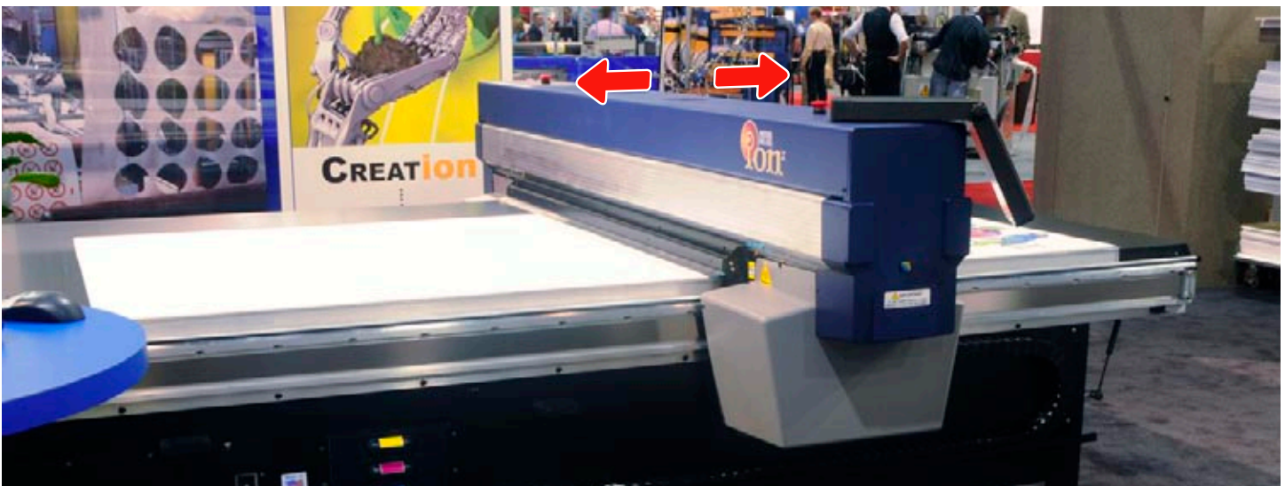
The whole gantry moves along the flatbed table. This means the rigid material is fixed while it is being printed on. SGIA '08 trade show.
