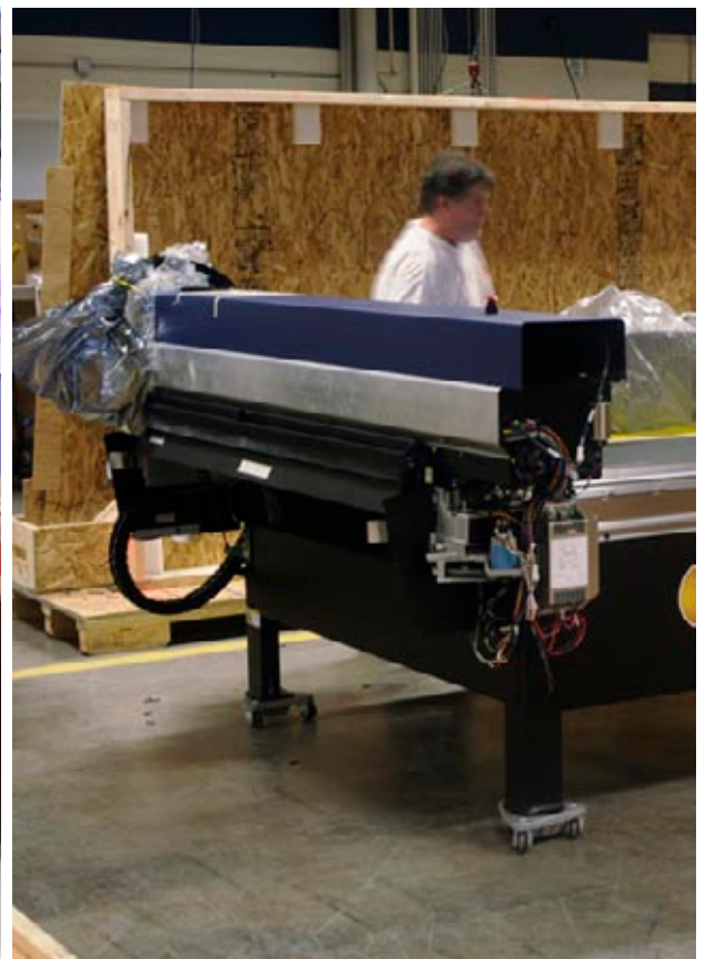
As you can see in these photos, the receptacle where the printhead carriage moves is totally enclosed. Dr. Hellmuth examined the assembly of the gantry (above). Here, the Gerber ionx at FESPA Mexico 2008 (lower left). Components being installed at the ends of the gantry (lower right).
