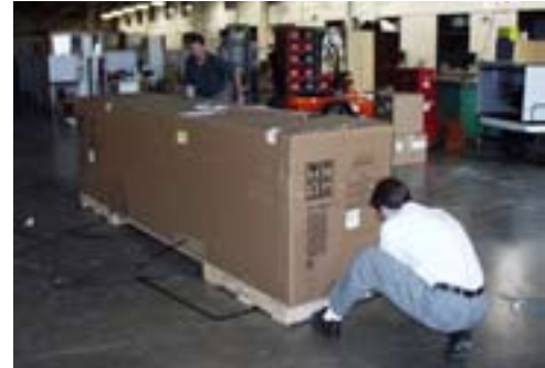
Removing the packaging staples.
