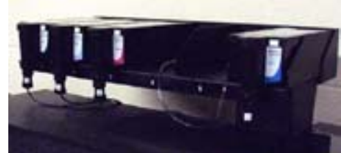
Four, six, and eight color ink system: installing an eight-color Endura-Chrome dye system.
