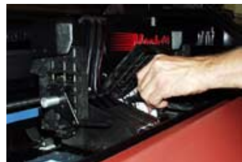
Installing the print heads.
