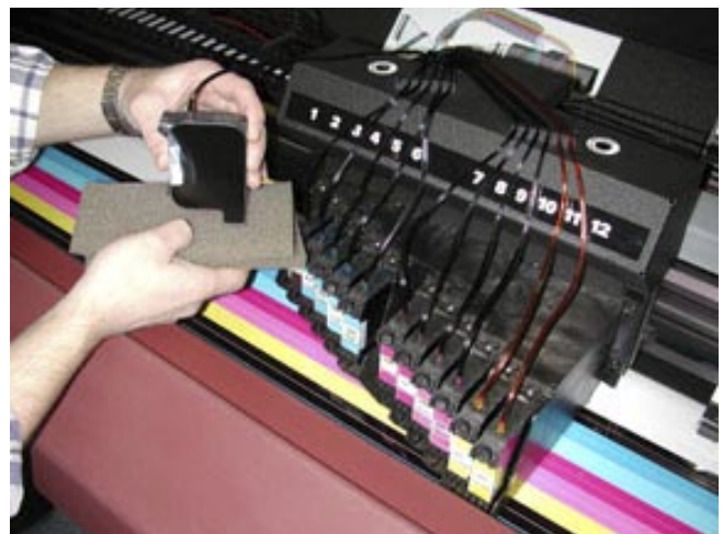
Cleaning the 12 printheads of the ColorSpan
