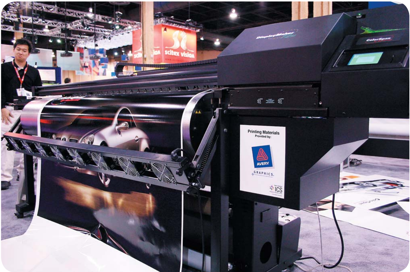
ColorSpan 72SI solvent ink printer as seen by Nicholas Hellmuth at ISA trade show, 2005
