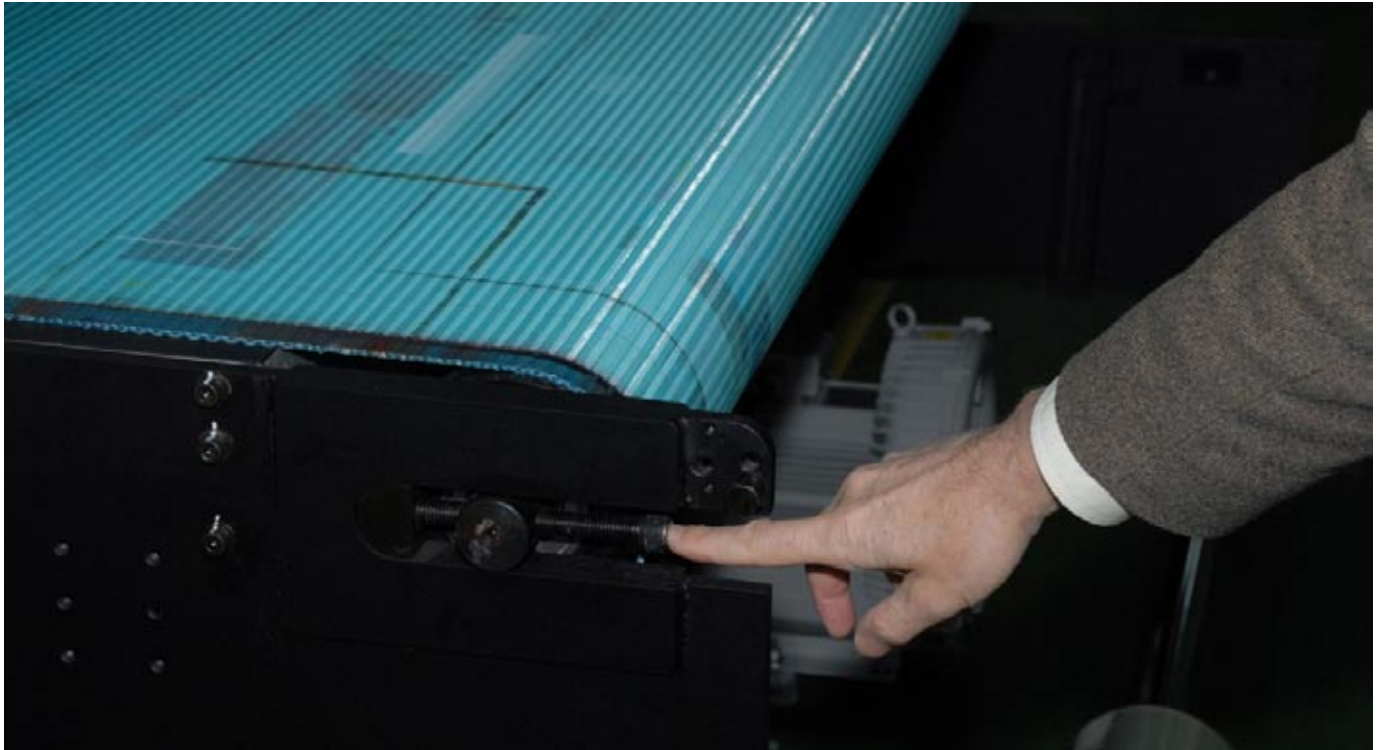
Transport belt adjustment system, Dilli factory, 2007.
