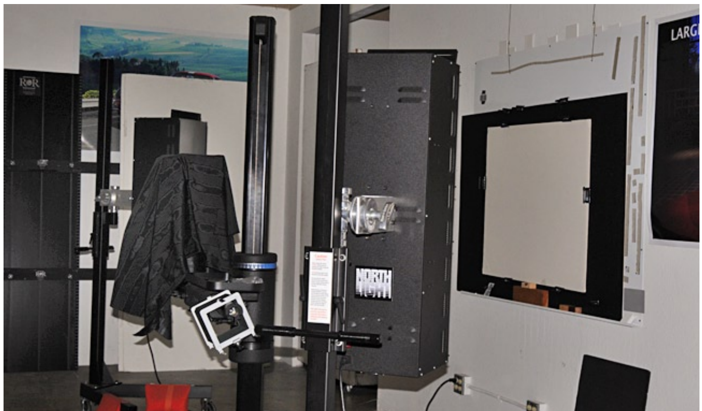
TTI stand and North Light studio lights, these equipment helps to take art photos with excellent illumination and to hold the camera without making any shadow.
