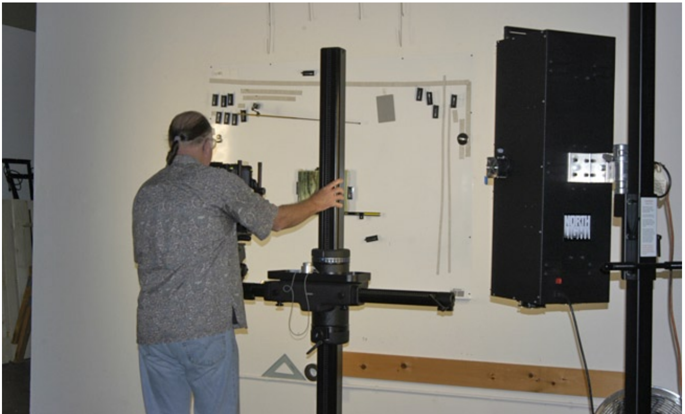
The Betterlight focusing card is place in front of the art canvas in order to achieve proper focus and fine detail.
