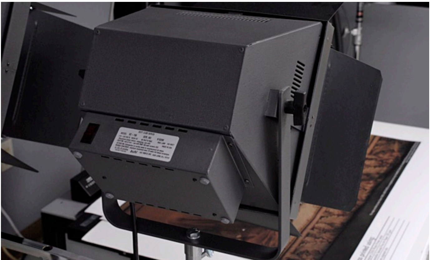
The trend today is to use studio lamps other than tungsten halogen. The new style of studio photo lamps for use with digital cameras is called CD (ceramic discharge) or HID (high intensity discharge). The lamps shown here (at Parrot Digigraphic) are from Buhl.
