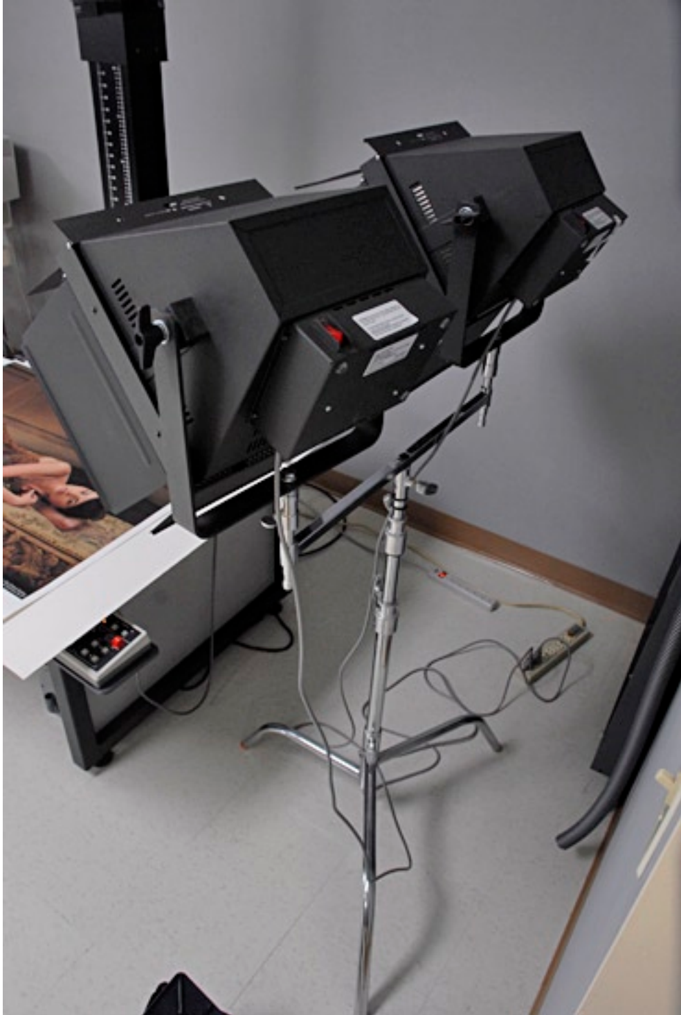
Set of Buhl maps that provide even lighting for the BetterLight scanback but don't overheat the painting.
