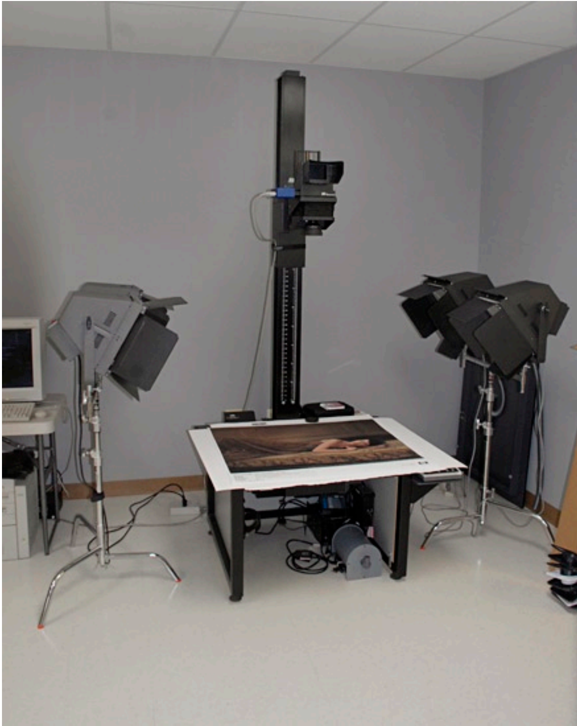
BetterLight scanback on a copy stand to take photographs of a painting: Parrot Digigraphic, 2007
