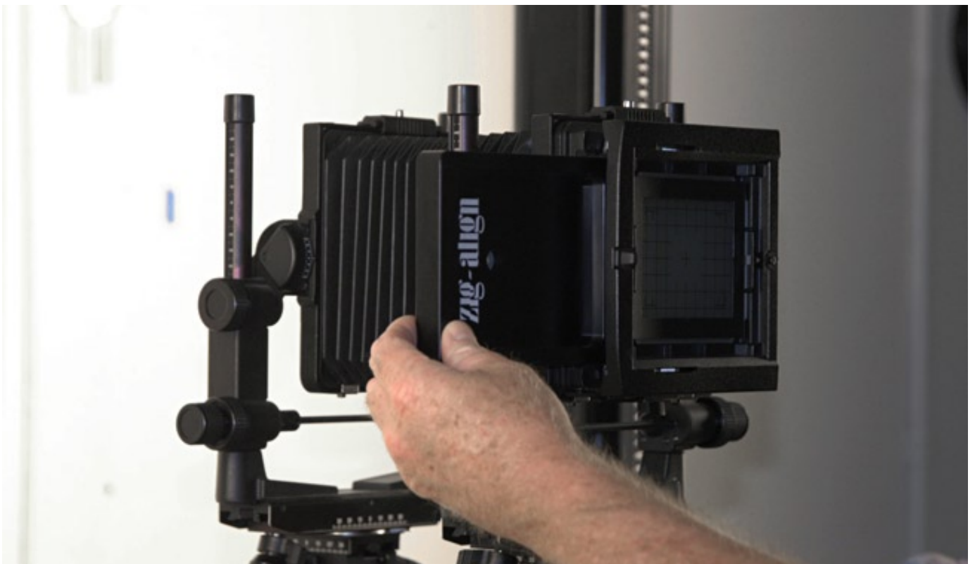
The following step is aligning the large format camera parallel to the art canvas; Zig Align is a company that has developed a system composed by mirrors that allow total parallel alignment.
