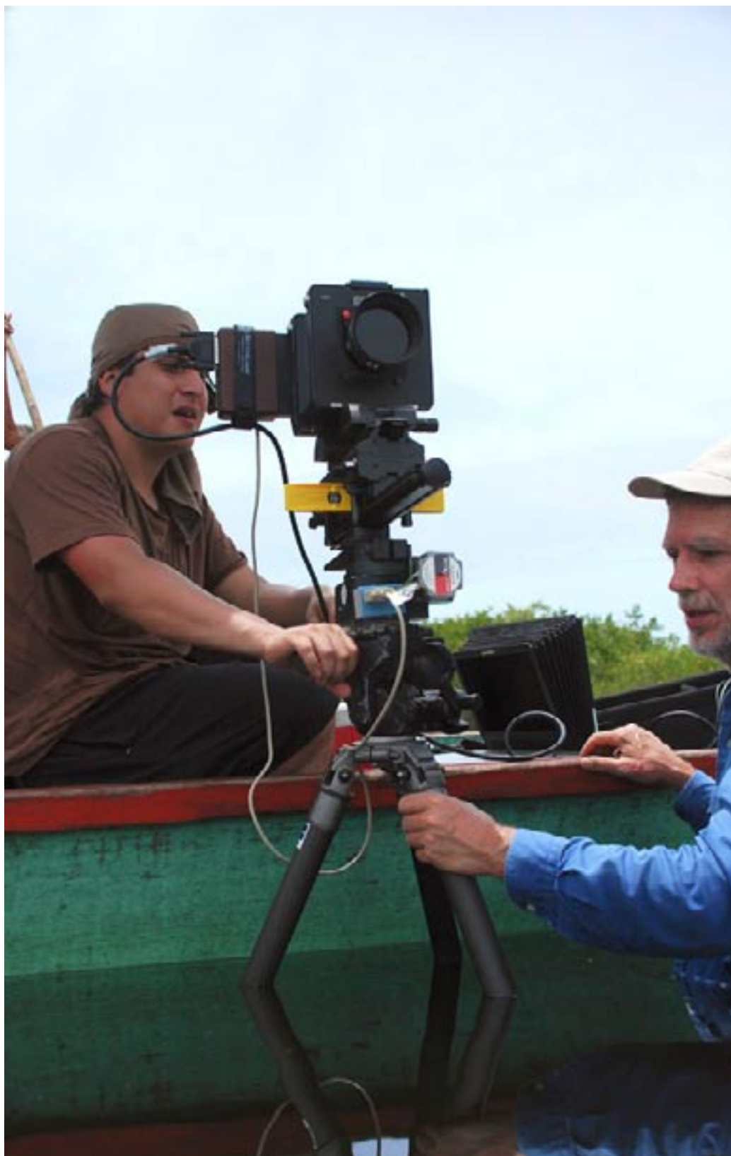
Is very important to have the camera level, since it is in the middle of the swamp everything was rocking. For this we have a special bubble level you can see it in the middle of the camera rails.
