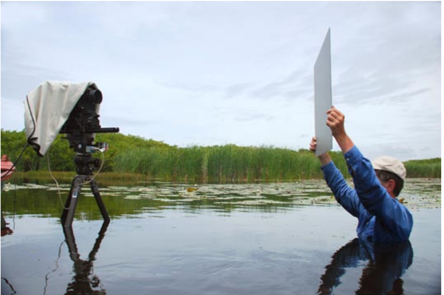
Don't forget to the the gray balance before you take any photograph. Here is Dr. Nicholas Hellmuth holding the gray balance card.
