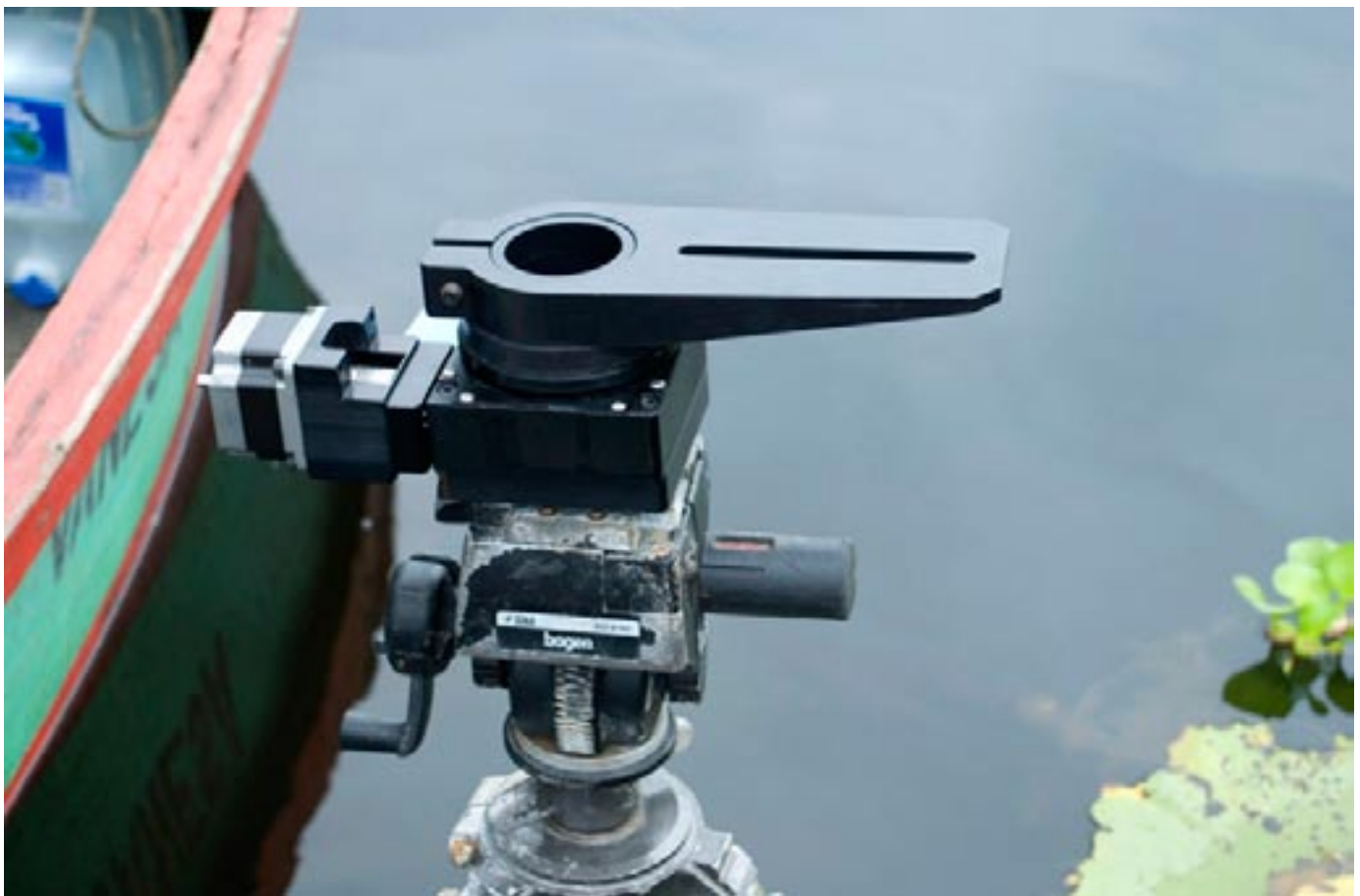
Here is the Better Light pano head adaptor to mount the Cambo 4x5.
