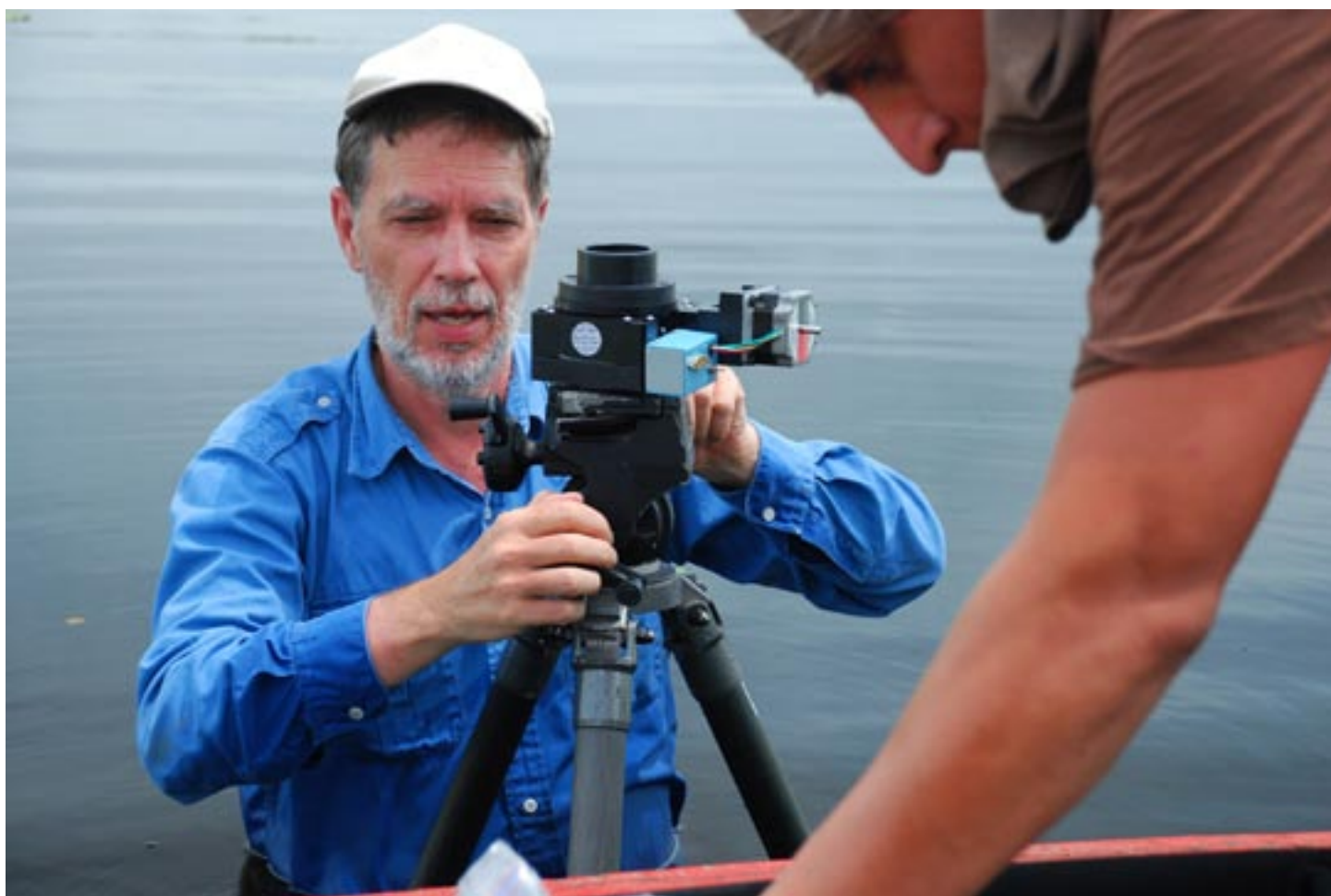
Here we are attaching the motor to the Manfrotto 3263 tripod head (from Bogen) for the Betterlight system to do panoramic photography.
