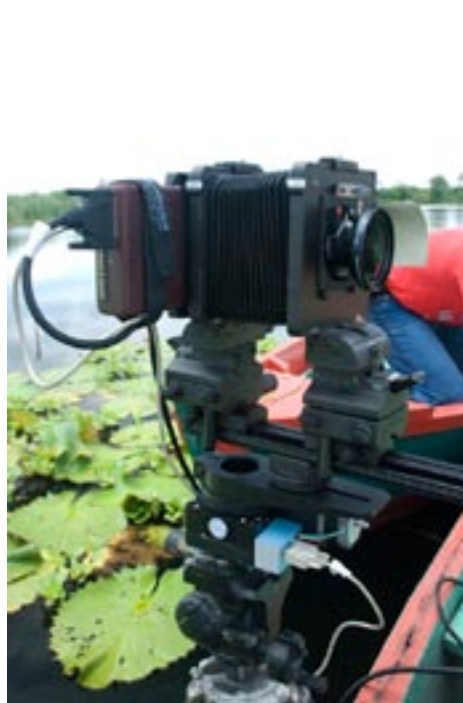
Here Luis is connecting the Betterlight Scan Back to the computer and to the Cambo 4x5.
