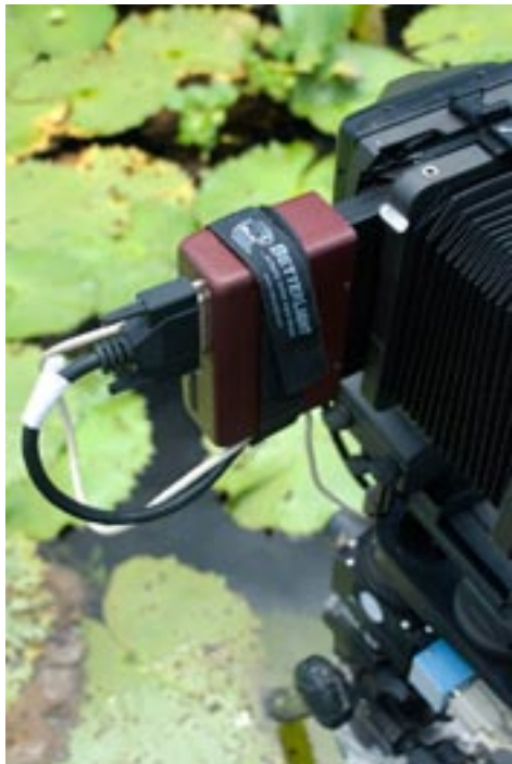
Here Luis is connecting the Betterlight Scan Back to the computer and to the Cambo 4x5.
