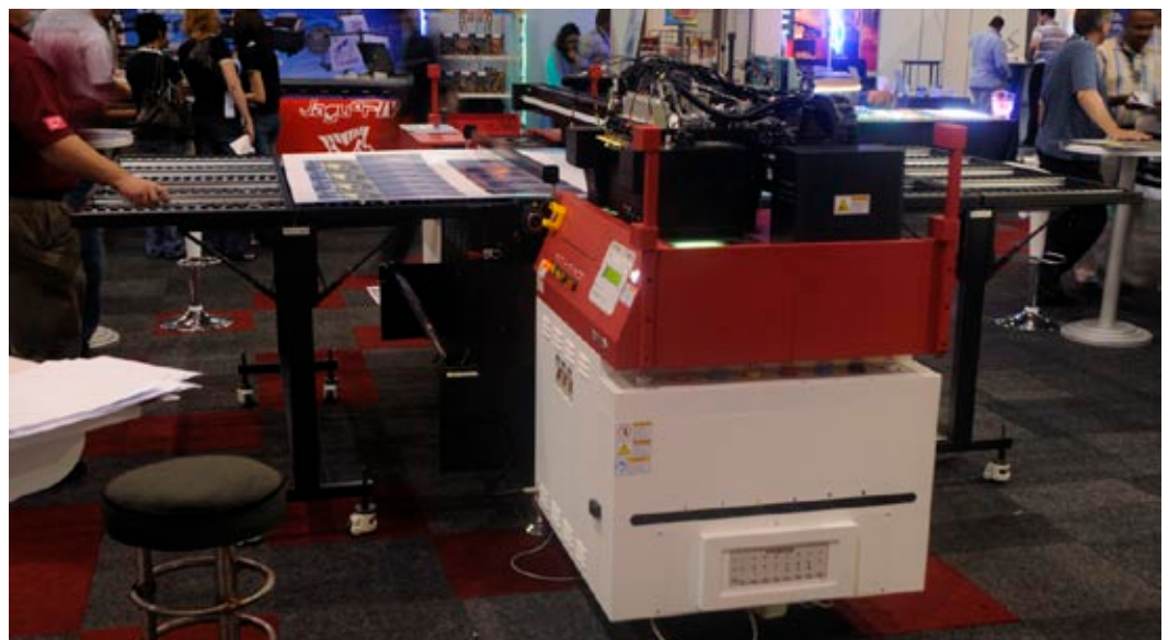
The front and rear tables of the :Anapurna Mv are easily detachable from the main chassis.
