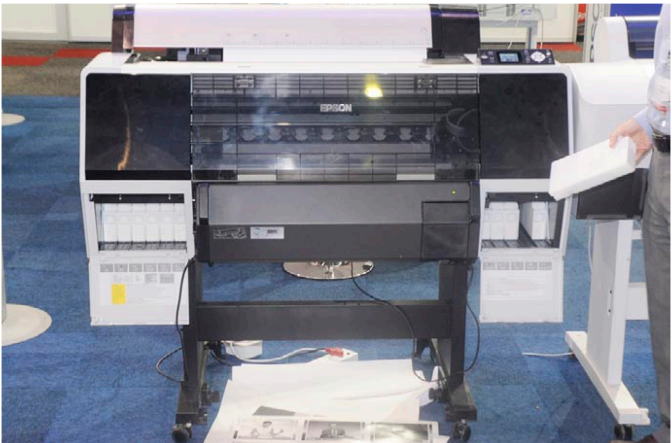
The Epson 7900 is said to use HDR (high dynamic range) ink in an 11-color configuration.
