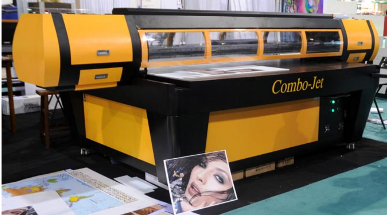
ESS, Electronic Sign Supply Combo Jet (Shanghai Electric, Human Digital) (Chinese, dedicated flatbed despite misnomer of Combo)
