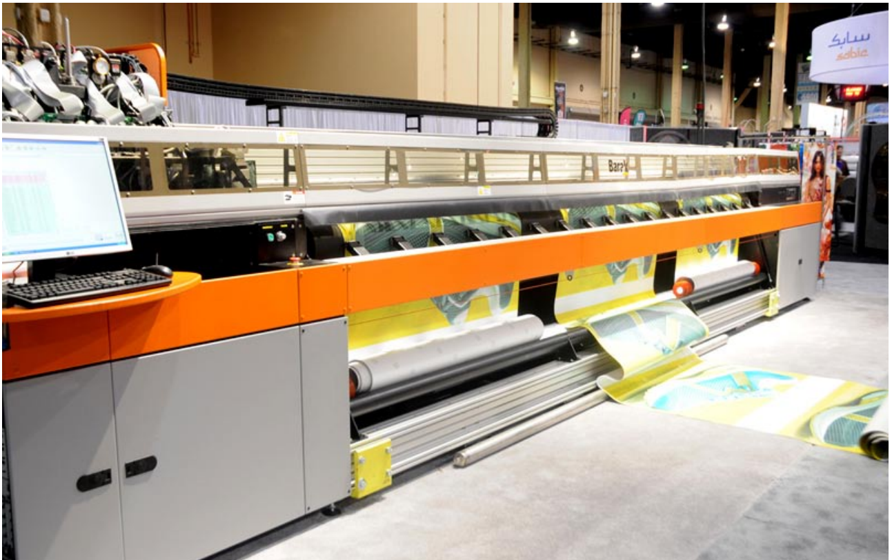
Matan Barak5, a dedicated 5-meter roll-to-roll with modest hybrid option for some flat material if you add front and back tables.
