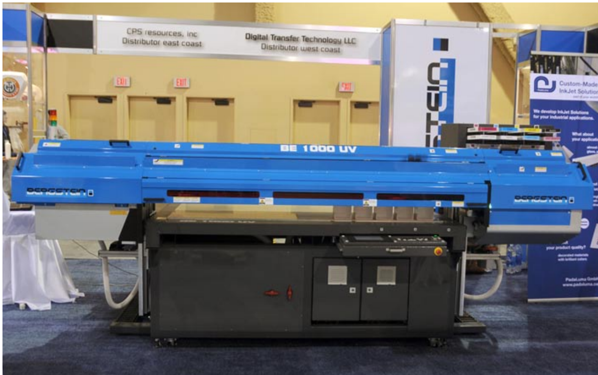
BE-1000UV, flatbed, based on a Mimaki chassis (shown at FESPA Geneva last year).
