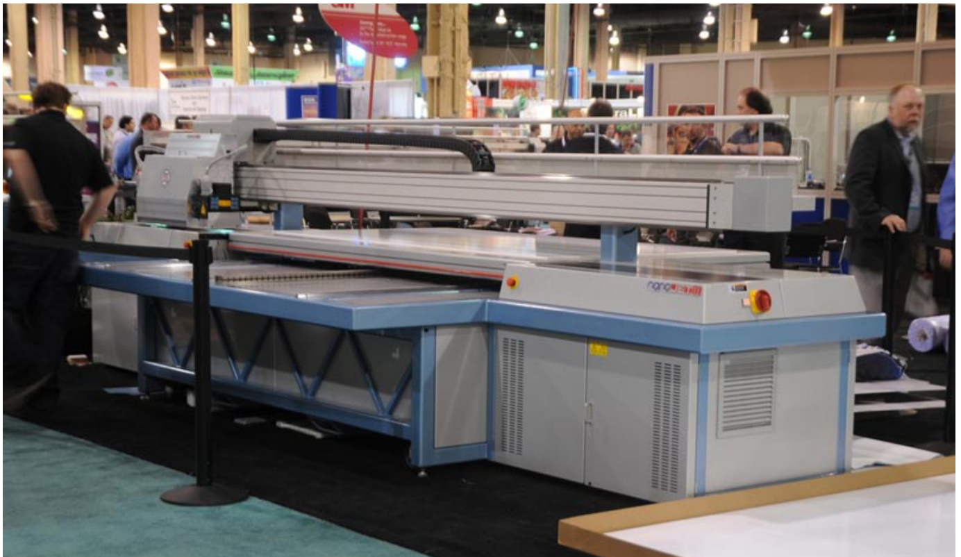
Gandininnovations Nano II (flatbed with Ricoh printheads)
