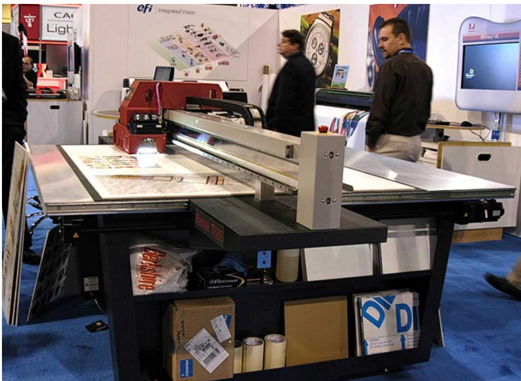
EFI Rastek T660, small flatbed with Toshiba Tec heads instead of original M Class
