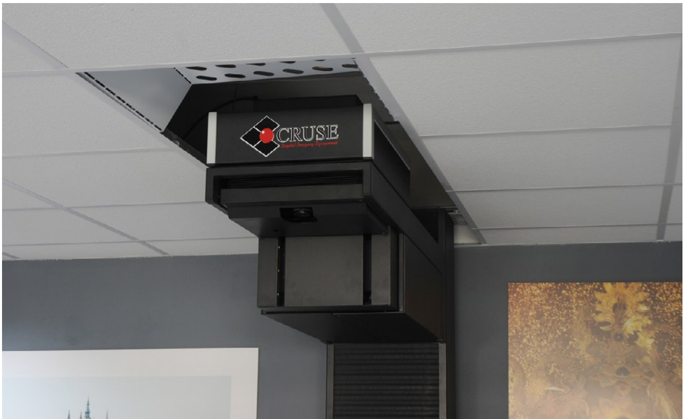
Tri-linear sensor and lens area of Cruse scanner. Note that the height of the scanner is necessary in order to capture large paintings, maps, etc.
