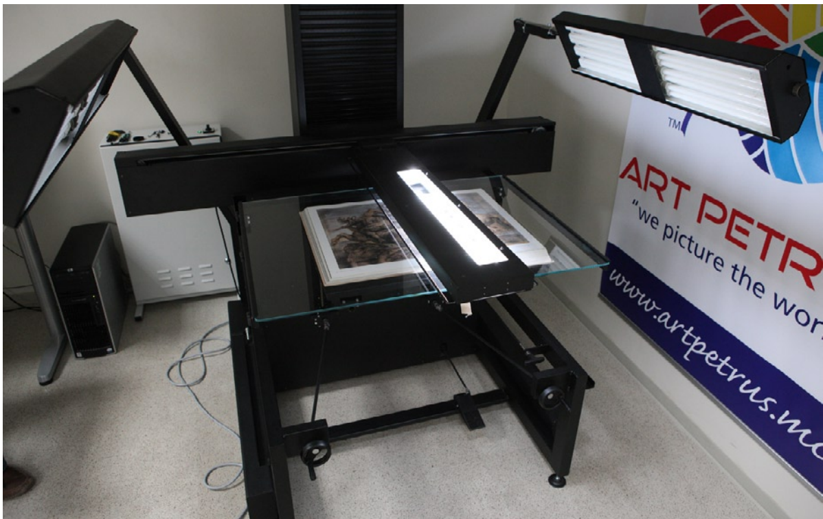
Archival scanner that Art Petrus occasionally uses for archive works and smaller documents and certain books as it has a book cradle. There are many different configurations and various models because they do many different kinds of high-end scanning for important clients throughout Europe.
