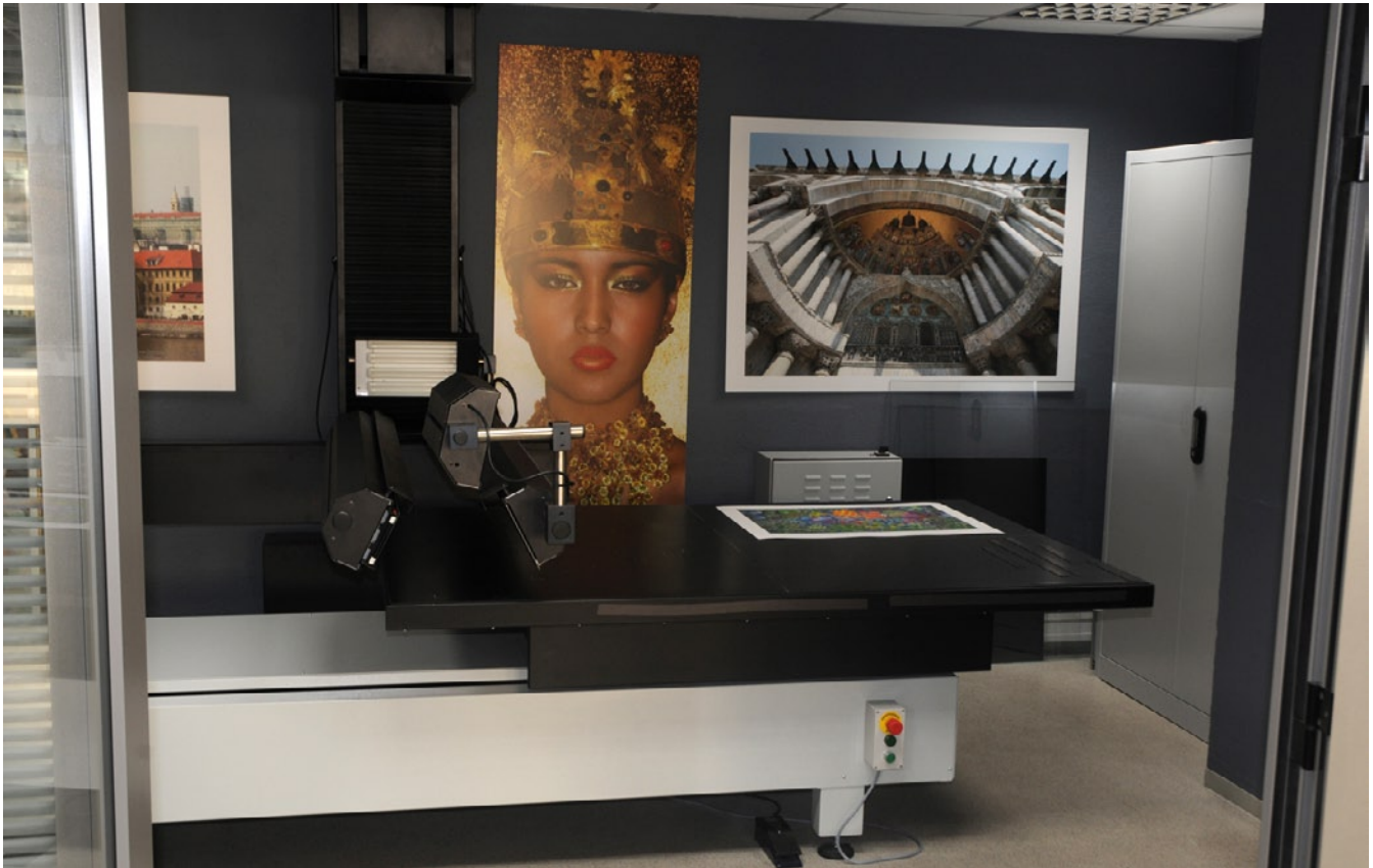
Cruse reprographic scanner with moving table (more precise than with moving lighting)
