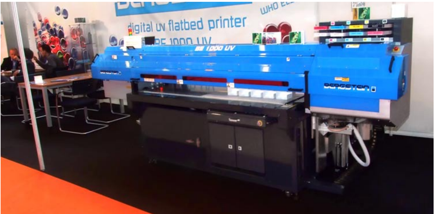
Bergstein 1000 UV, flatbed based on Mimaki JF-1610 chassis but adapted.
