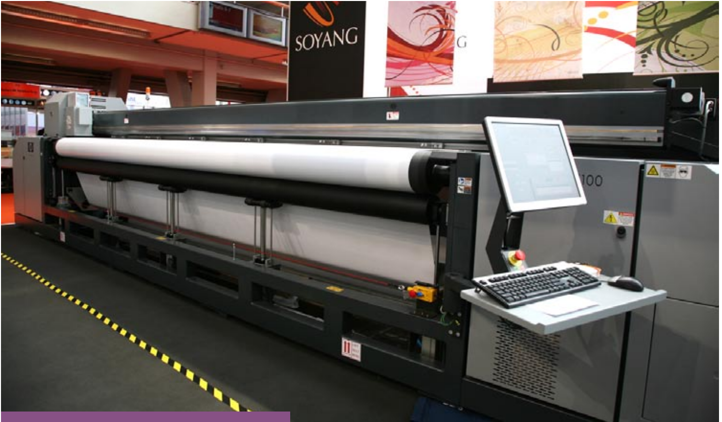
HP Scitex XP 5100 roll-to-roll UV printer.
