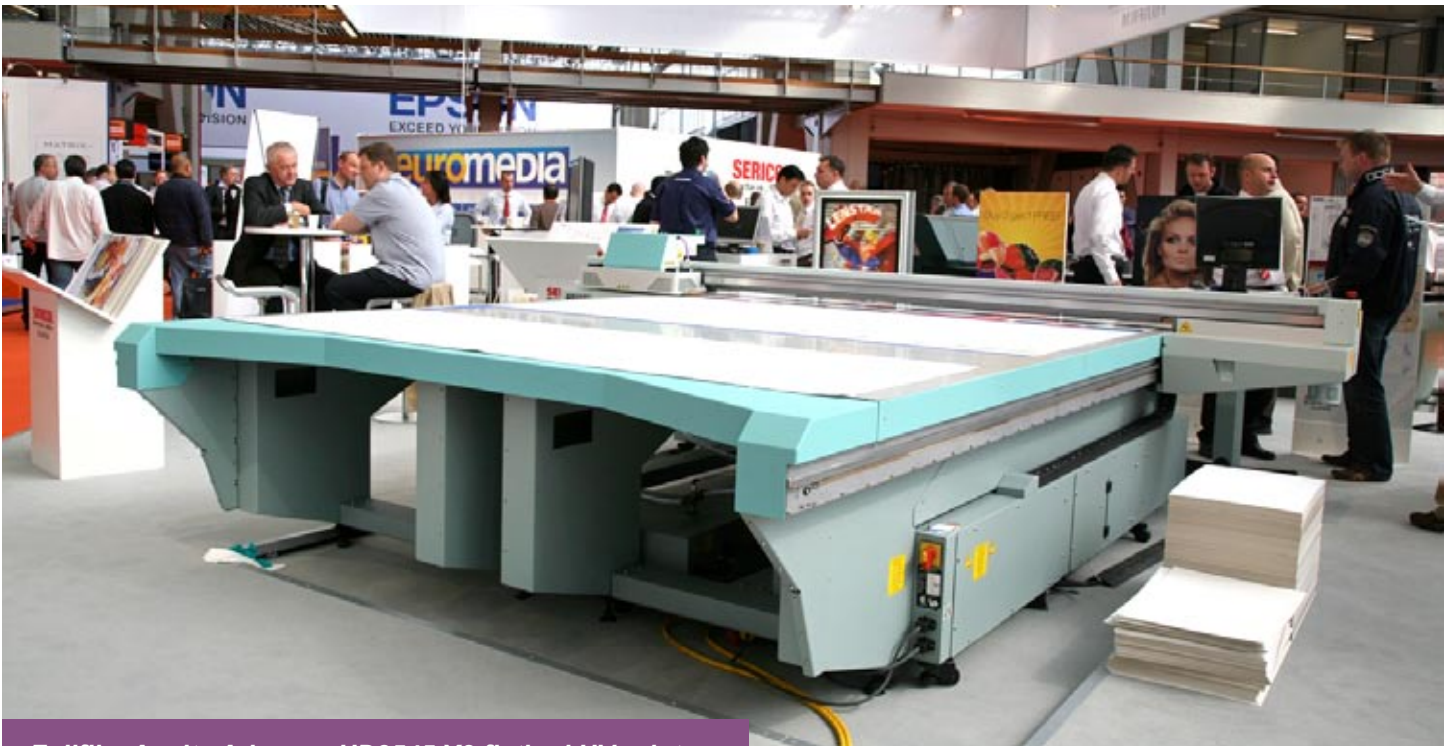
Fujifilm Acuity Advance HD2545 X2 flatbed UV printer.
