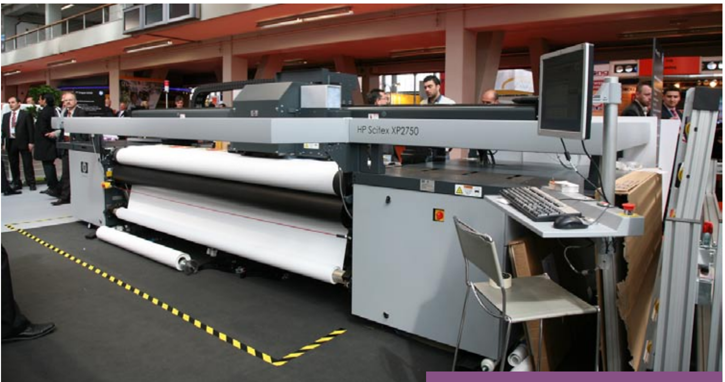
HP Scitex XP 2750 roll-to-roll UV printer.
