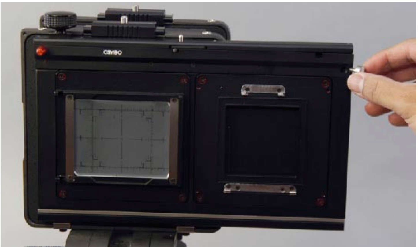
Figure 13. To change between one shot or multishot the click stop plate in the upper right corner must be changed.
