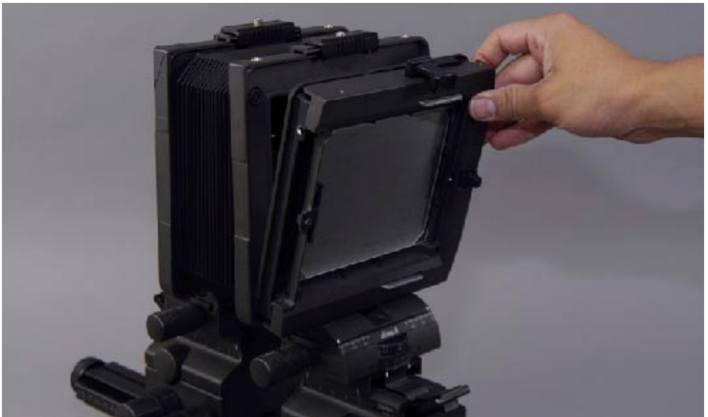
Figure 3. The sliding back adapter is placed in the rear standard of the camera by removing the ground glass.
