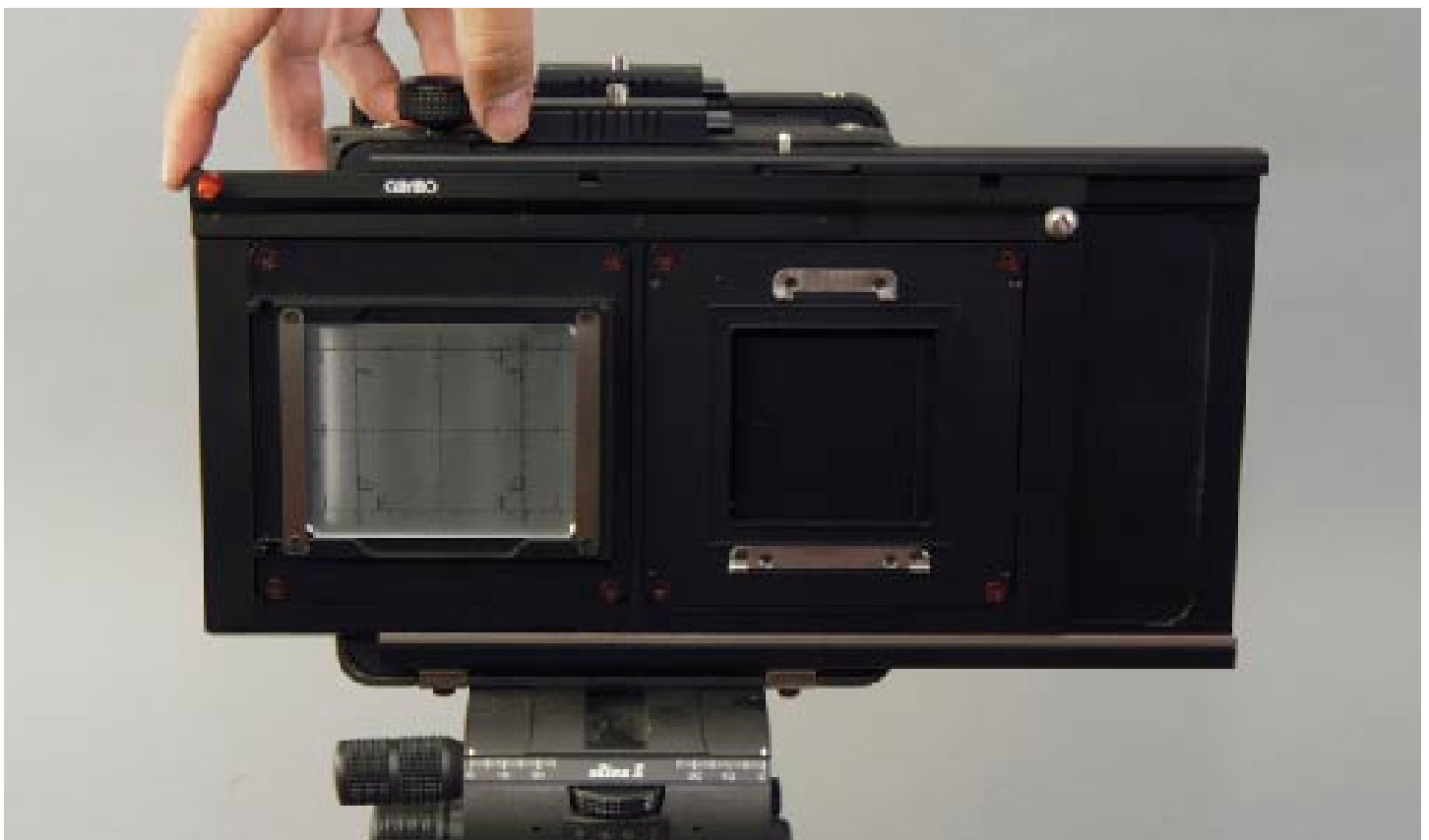
Figure 9. The upper knob moves the sliding plate to the image plane.
