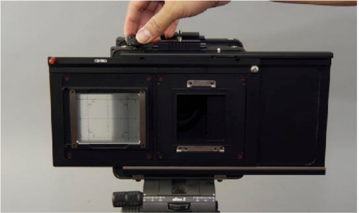
Figure 10. The security pin will lock the digital back to the image plane.
