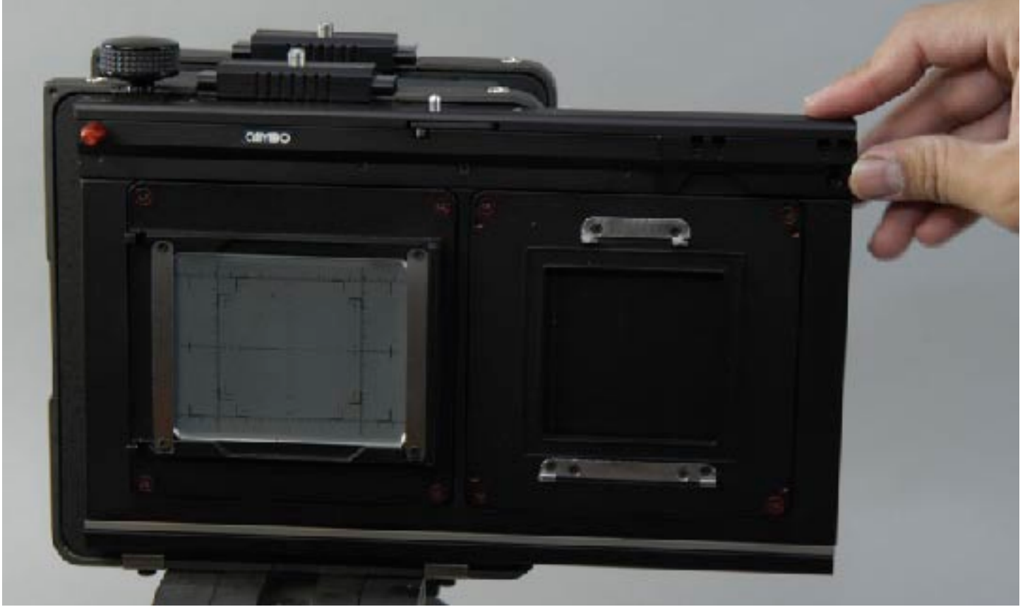
Figure 16. Once in its placed the multiple shot plate can be used with the digital back either in horizontal or vertical position.
