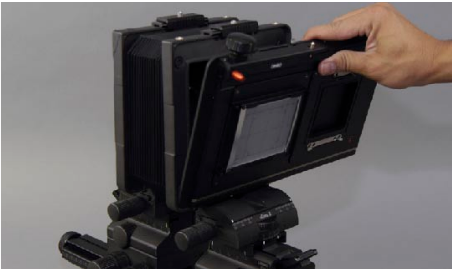
Figure 5. Cambo rear standard ready to receive the sliding back adapter.
