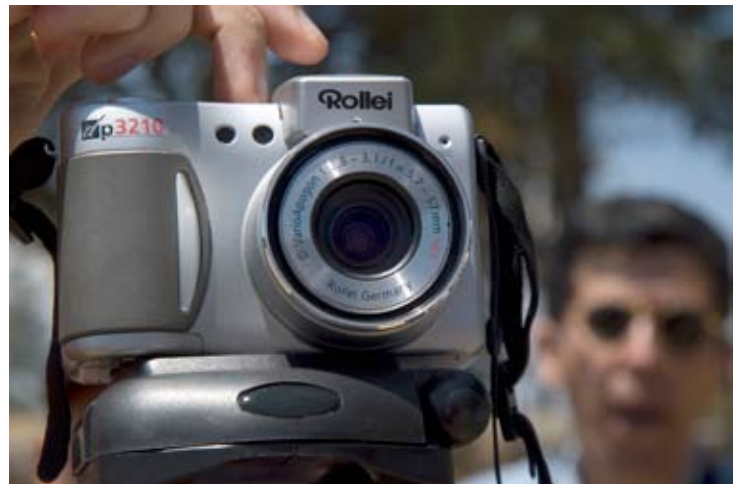
Rollei p3210 digital photogrammetric camera, used to take the photos to create a digital 3D model.
