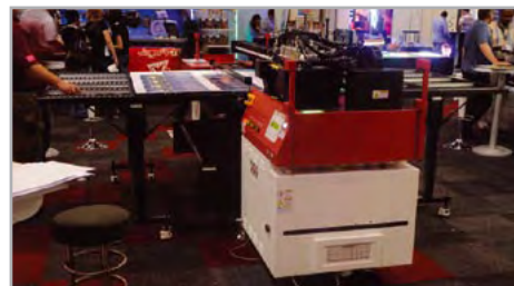
The front and rear tables of the :Anapurna Mv are easily detachable from the main chassis.
