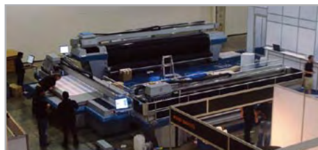
The front and rear tables of the :Anapurna Mv are easily detachable from the main chassis.
