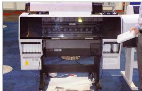
The Epson 7900 is said to use HDR (high dynamic range) ink in an 11-color configuration.
