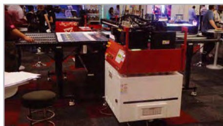
The front and rear tables of the :Anapurna Mv are easily detachable from the main chassis.
