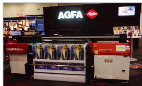
Agfa :Anapurna Mv printing on flexible material. This is an exposed combo UV printer.
