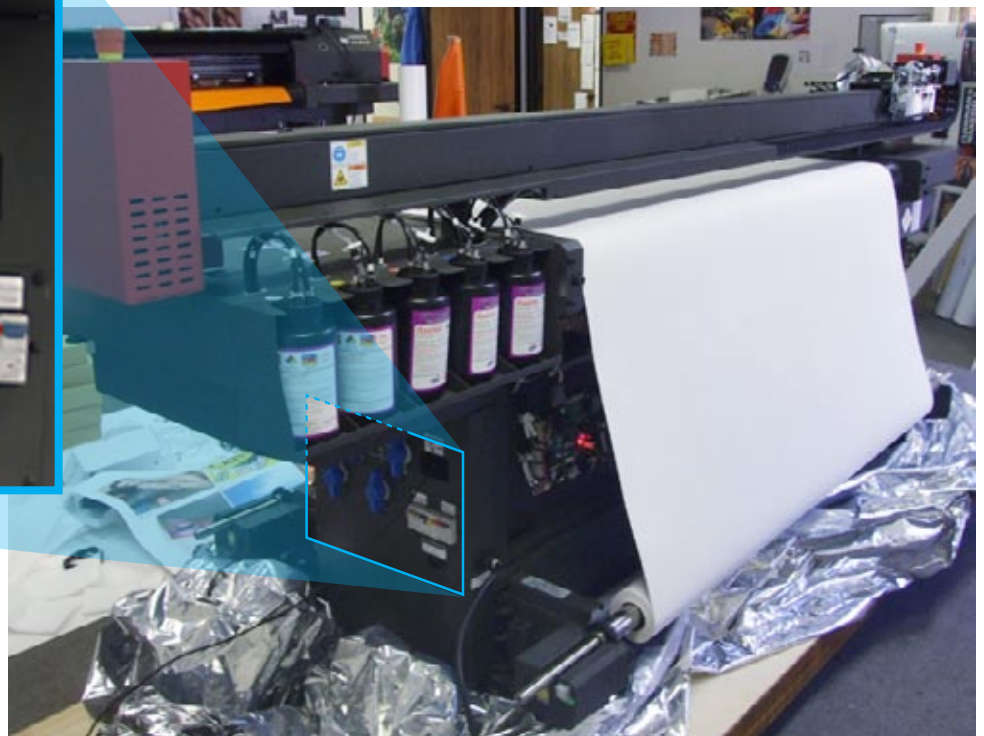
In this rear view of the printer you can see the location of the valves that control the vacuum sections.
