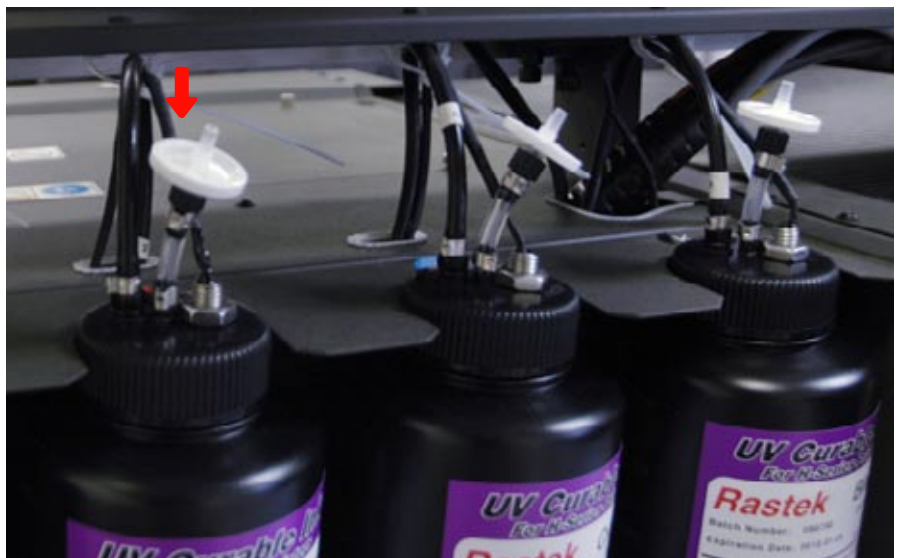
These are the ink filters that need to be changed more constantly.
