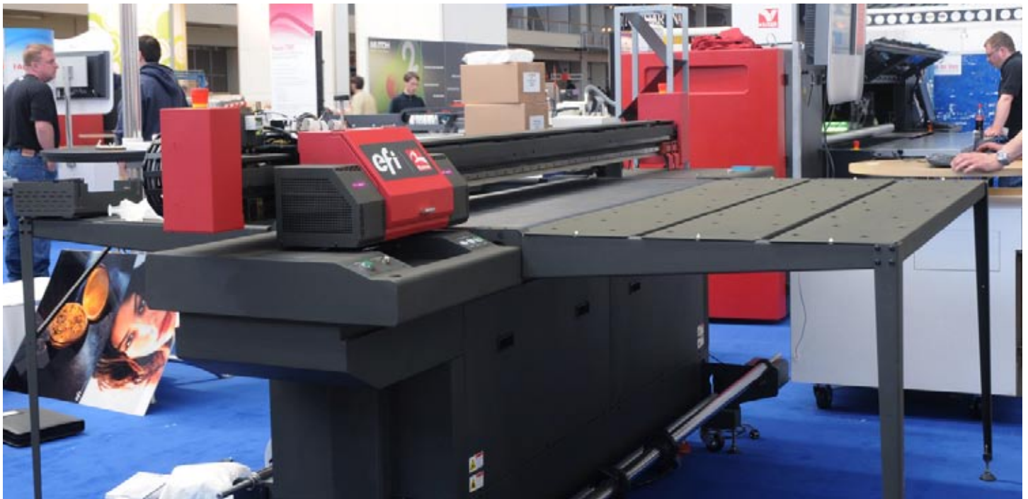
EFI Rastek H650 at FESPA Amsterdam '09. Health regulations are particularly strong in Europe, but no exhaust system was required by the printer in this trade show. Other printers of a more industrial size, WP Digital, HP, or Durst did have exhaust pipes installed.
