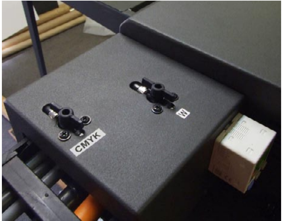
These are the valves to control which ink lines are going to be purged.
