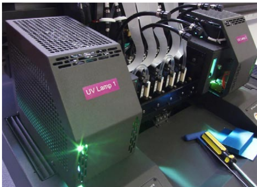
The UV lamps are covered, but there is still some light leakage.
