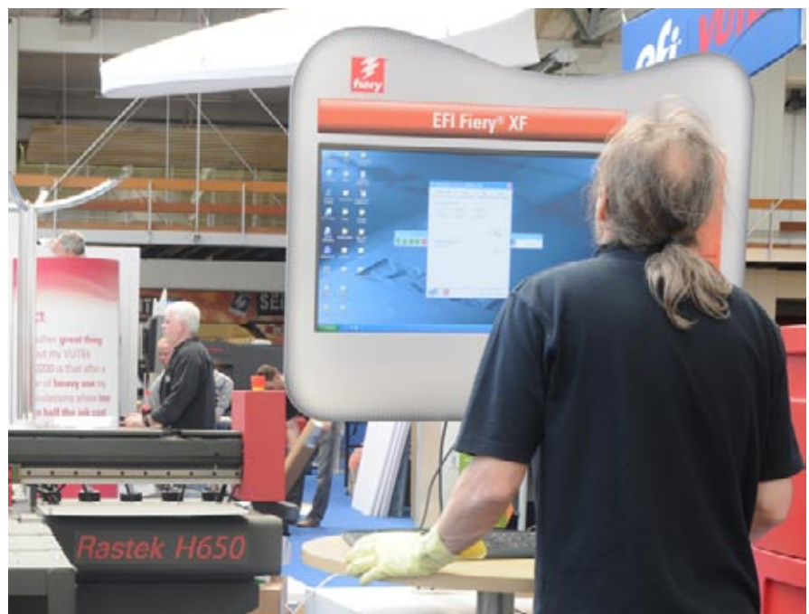
The main operations are controlled via software. The PC is not fixed in the printer, which means you can place it in the position that is more convenient to you.
