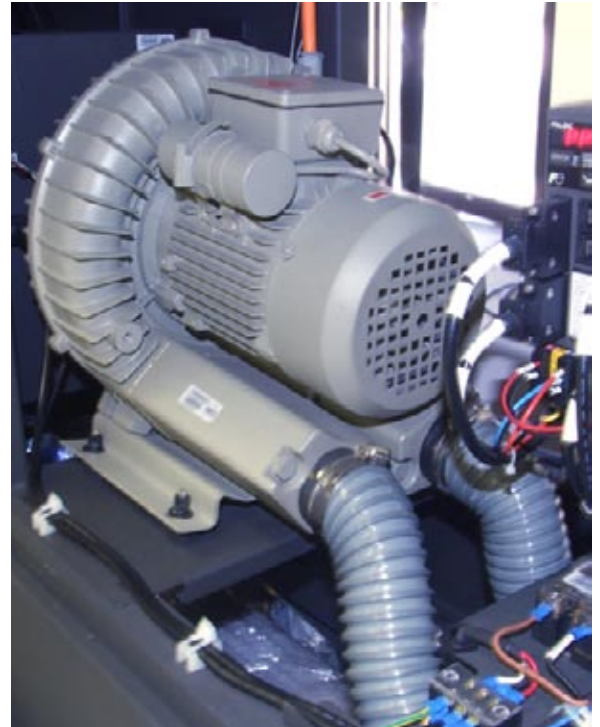
The vacuum is generated by one air pump located below the printing area. To have the pump inside the body of the printer is a plus considering that some printer manufacturers have a bulky air pump sitting next to the printer.
