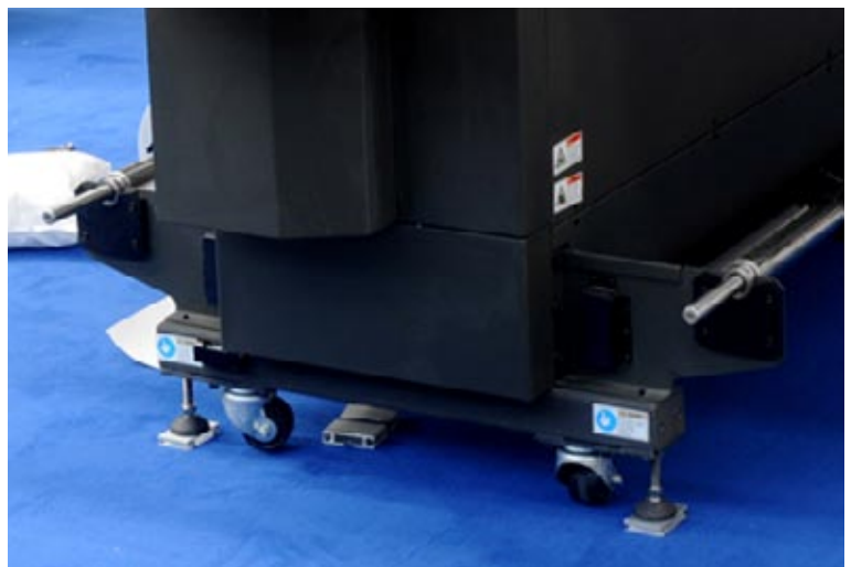
Wheels and leveling supports of the EFI Rastek H650 introduced at FESPA Amsterdam '09. Wheels and leveling supports are separate structures.
