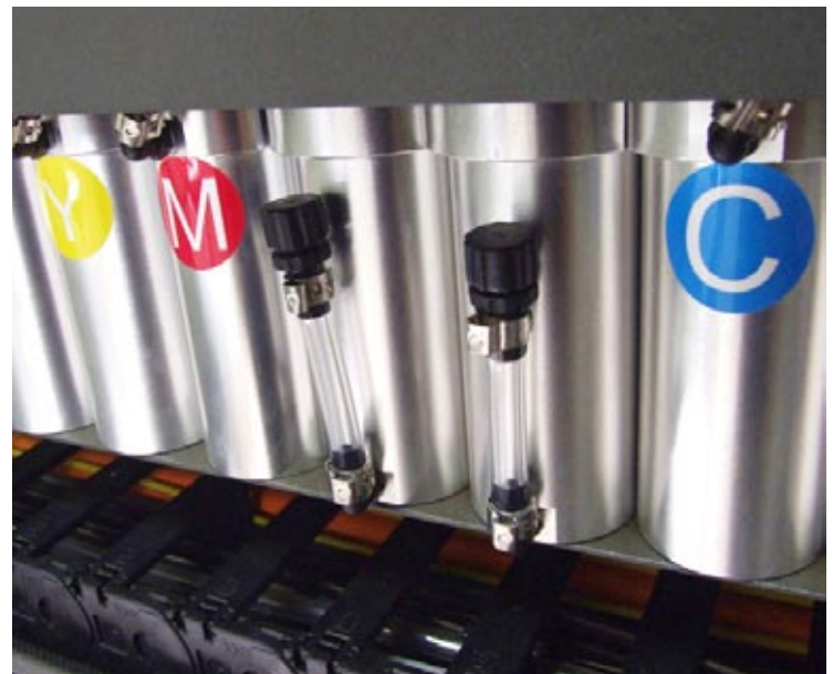
The secondary ink tanks are located behind the printhead carriage.
