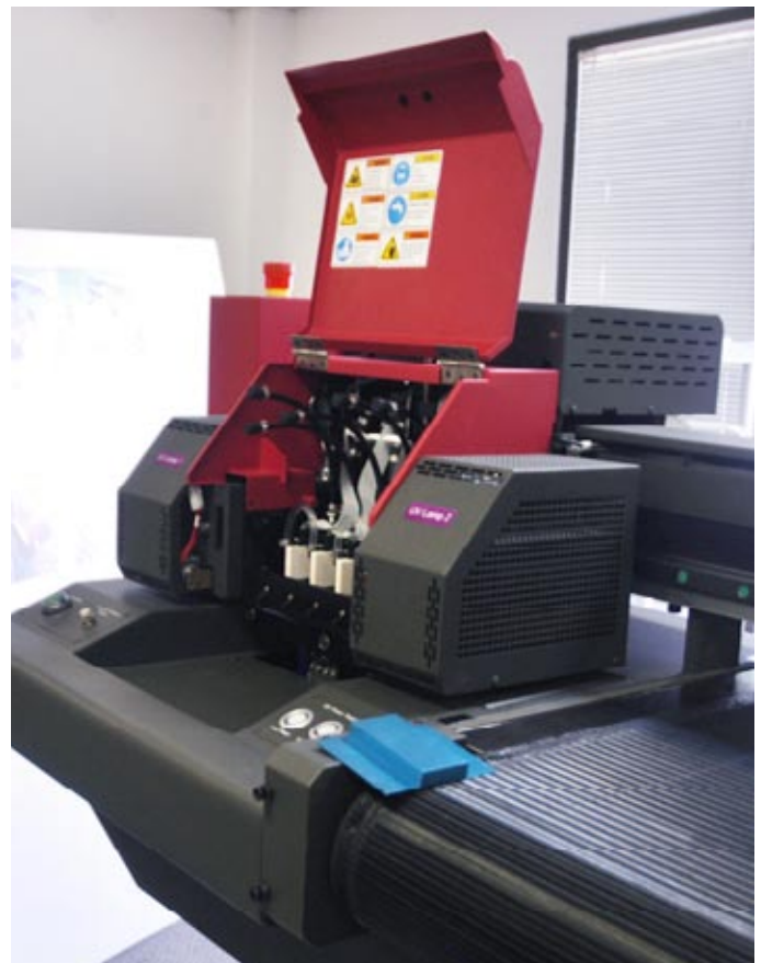
The area of the printheads is easily accessible once you open the hood of the carriage; however, there is a suction system so that you don't have to touch the printheads.
