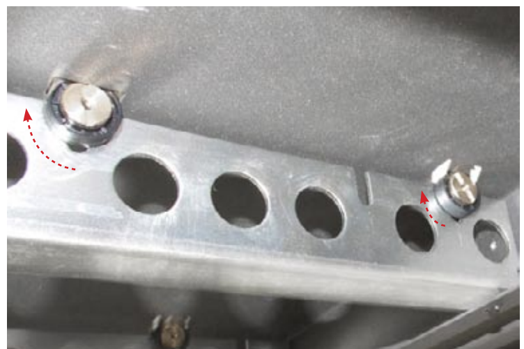
This photo taken from below the table shows the little rollers that help move media forward.
