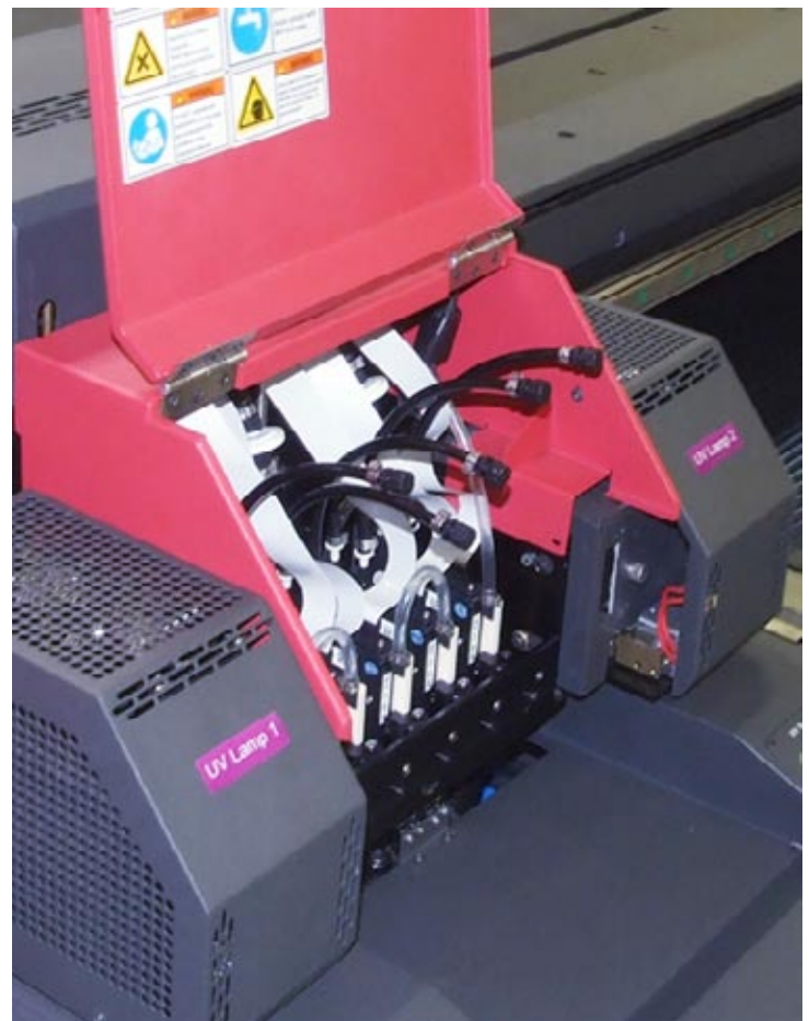
Printheads are aligned in a straight row.
