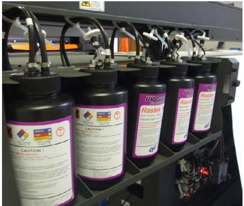
This model has a CMYK + W configuration. The bottle at the far left is the one for white ink.
