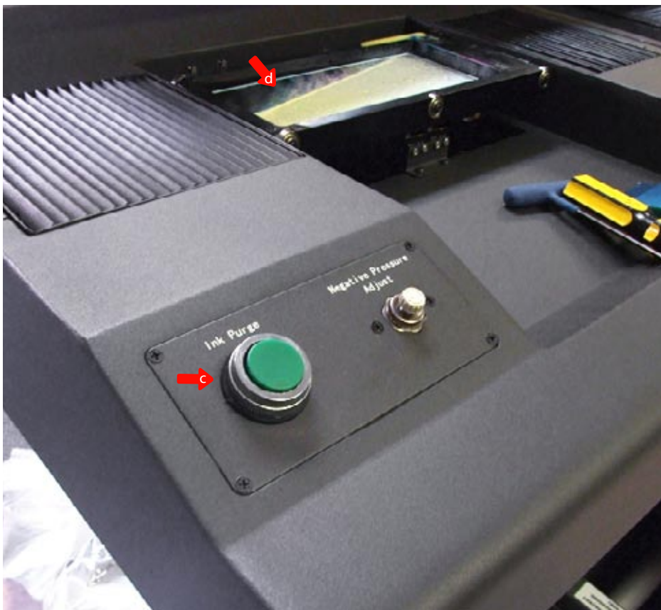
You start the purging procedure by pushing a button (c). Then, ink that is purged from the printheads is collected by a tray (d) and finally goes to the waste bottle (right photo) located at the back.
