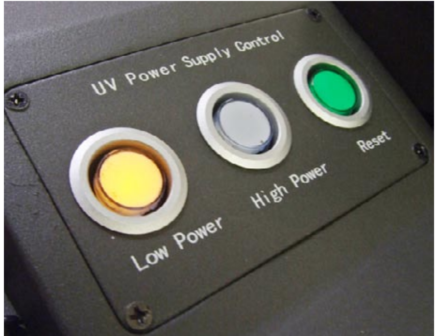
The control buttons for the UV lamps are at the front.
