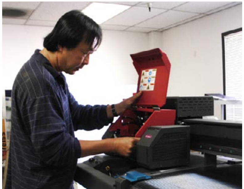
Although the printhead area tends to be the most difficult area to access, there is not much you need to do since the cleaning is done by a suction system (not manually). The technician is working in the printhead area to finish installation of this model.
