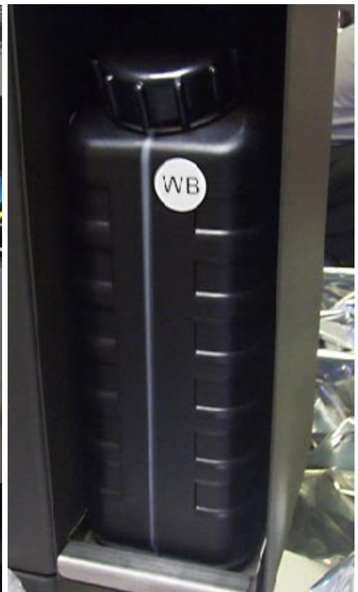
You start the purging procedure by pushing a button (c). Then, ink that is purged from the printheads is collected by a tray (d) and finally goes to the waste bottle (right photo) located at the back.
