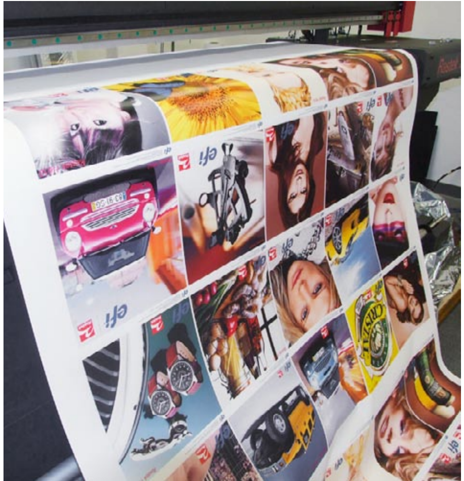
Some substrates come already pretreated, especially media manufactured for inkjet printers, whereas other media whose purpose is not only to be printed on, might require some pretreatment to help ink adhesion.
