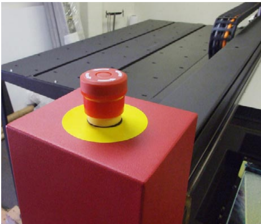
The only controls at the sides are the emergency stop buttons and the valves that control the vacuum sections.
