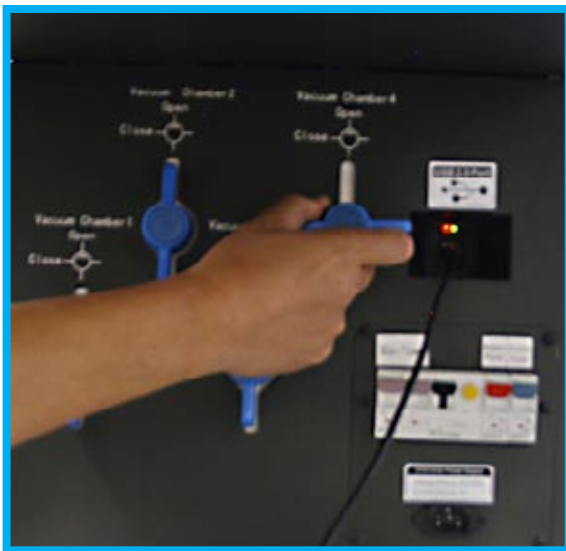
In this rear view of the printer you can see the location of the valves that control the vacuum sections.
