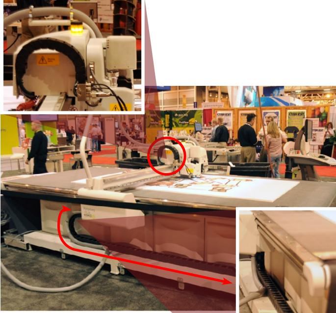
The energy chain is the plastic linked system that holds all the cables and ink tubing so that it does not get rubbed while being moved back and forth to feed the carriage.
