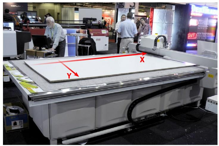
The table is always fixed in one position, the gantry can move in X and Y position.
