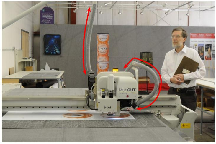
The cutter has a suction hose with a vacuum cleaner to reduces the dust and detritus of the material that is being cut.
