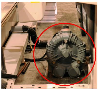
The vacuum system in the table is created by an air pump.
