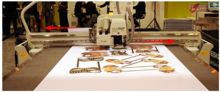
The Kongsberg XL cutter series uses appropriate brushless servo motors. The advantage of using a servo motor is that it provides feedback and can correct its positioning.
