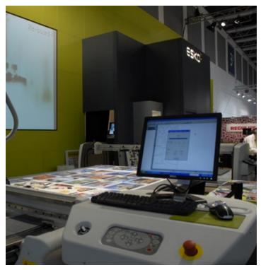
The operational area has a keyboard, a regular computer monitor (about 15 or 16"), and a control pad area with a usual set of buttons to make various selections.
