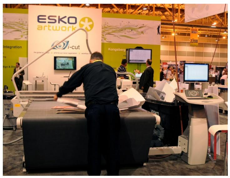
Maintenance is limited to the inspection and cleaning of the table surface, guideway, rollers, racks, pressure reduction valve, base and the surrounding area; The table surface should be kept clean at all times. For cleaning, use iso-propyl alcohol, use a vacuum cleaner to keep the inside of the conveyor belt clean.
