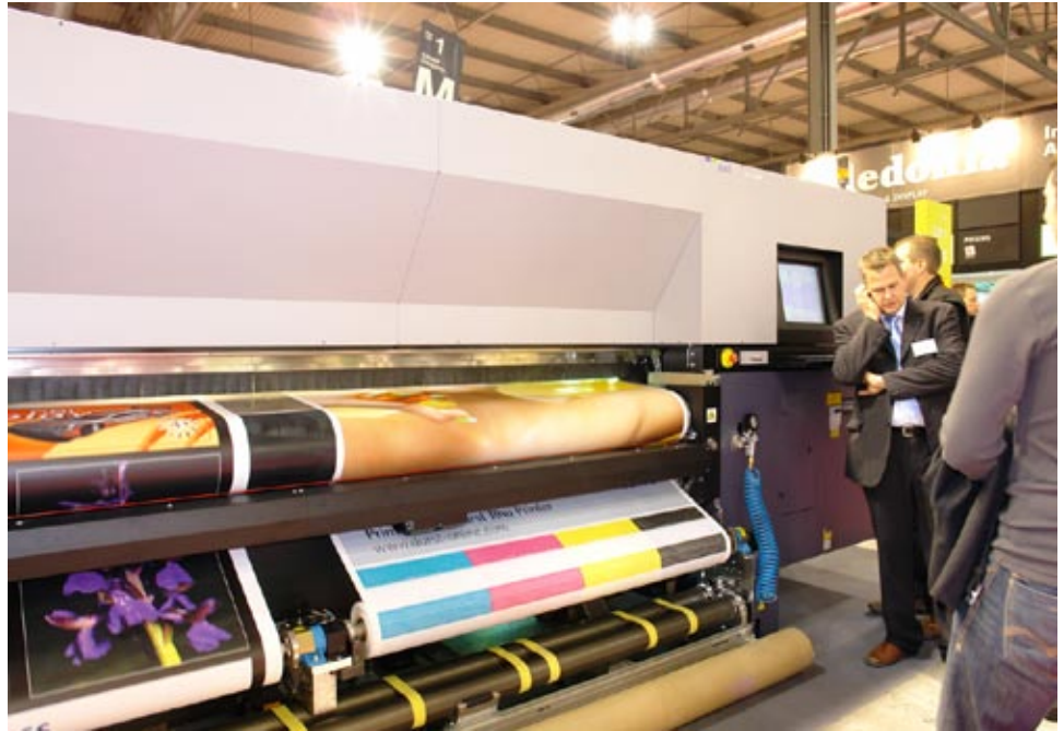
Durst Rho 500R, notice how easy it is to print two or more different rolls of media at same time with this printer.
