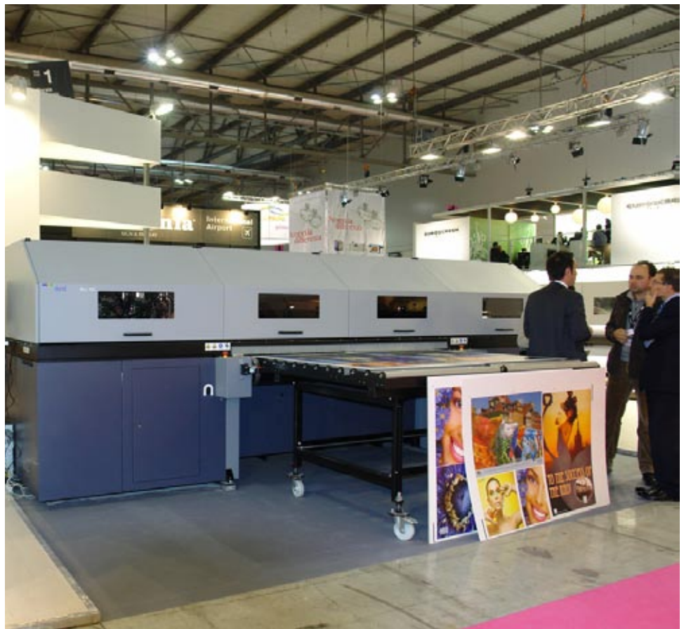
Durst Rho 700, combo UV printer with some printed samples at front.
