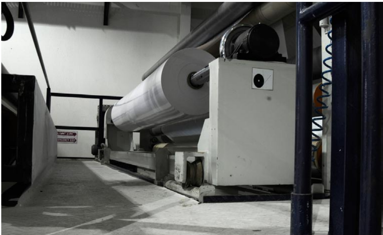
There are two PVC dip coating lines: 3.2 meters and 5 meters. Most Chinese factories are not yet able to handle 5 meter rolls.
