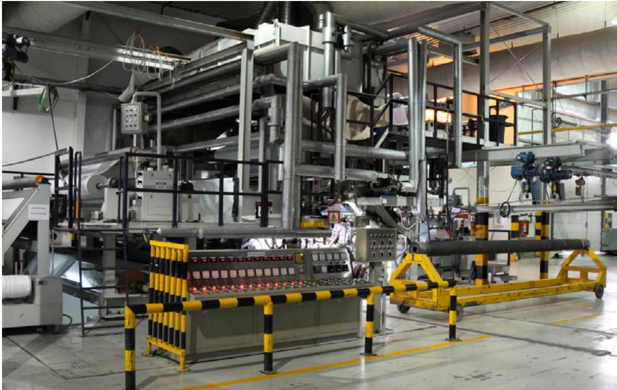
Here is one machine for laminating the knitted material. The knitted material is produced from the new yarn factory.
