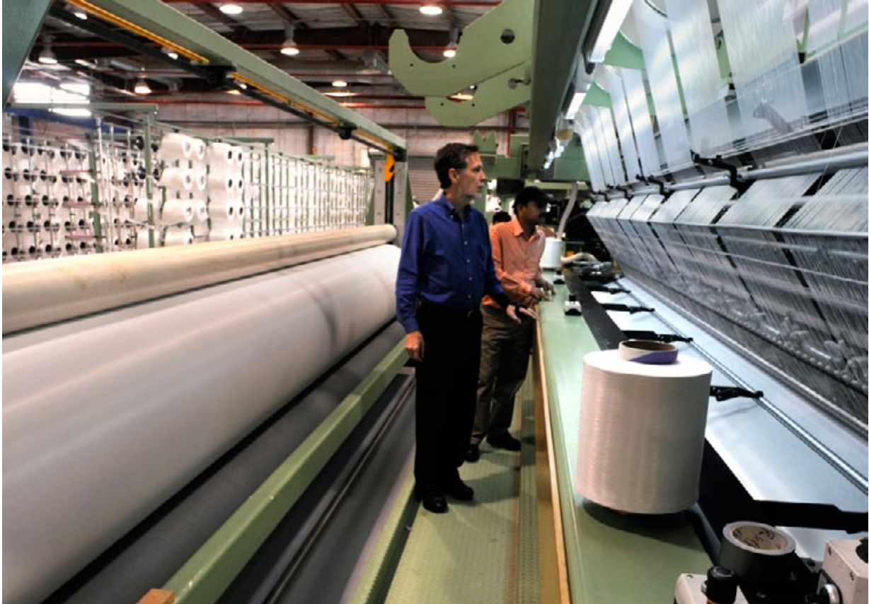
Here I am with one of the experienced operators inside the 5-meter knitting machine.
