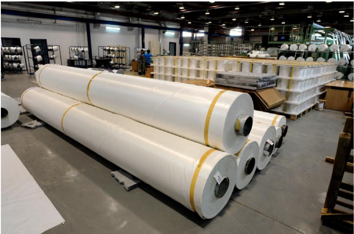
Here are some finished rolls; some are 3.2 meter width and also 5 meters.
