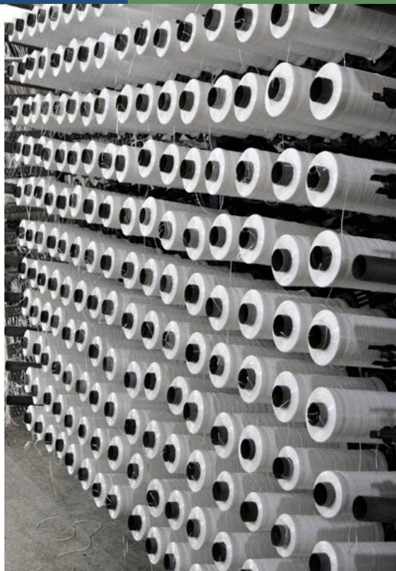
Bobbins with PE thread carefully loaded as part of the weaving process.
