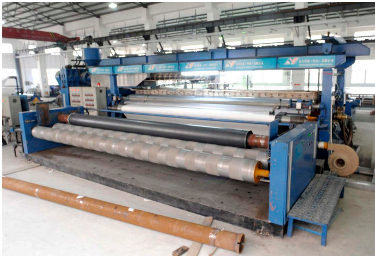
Covering six-meter wide woven PE with PE coating.
