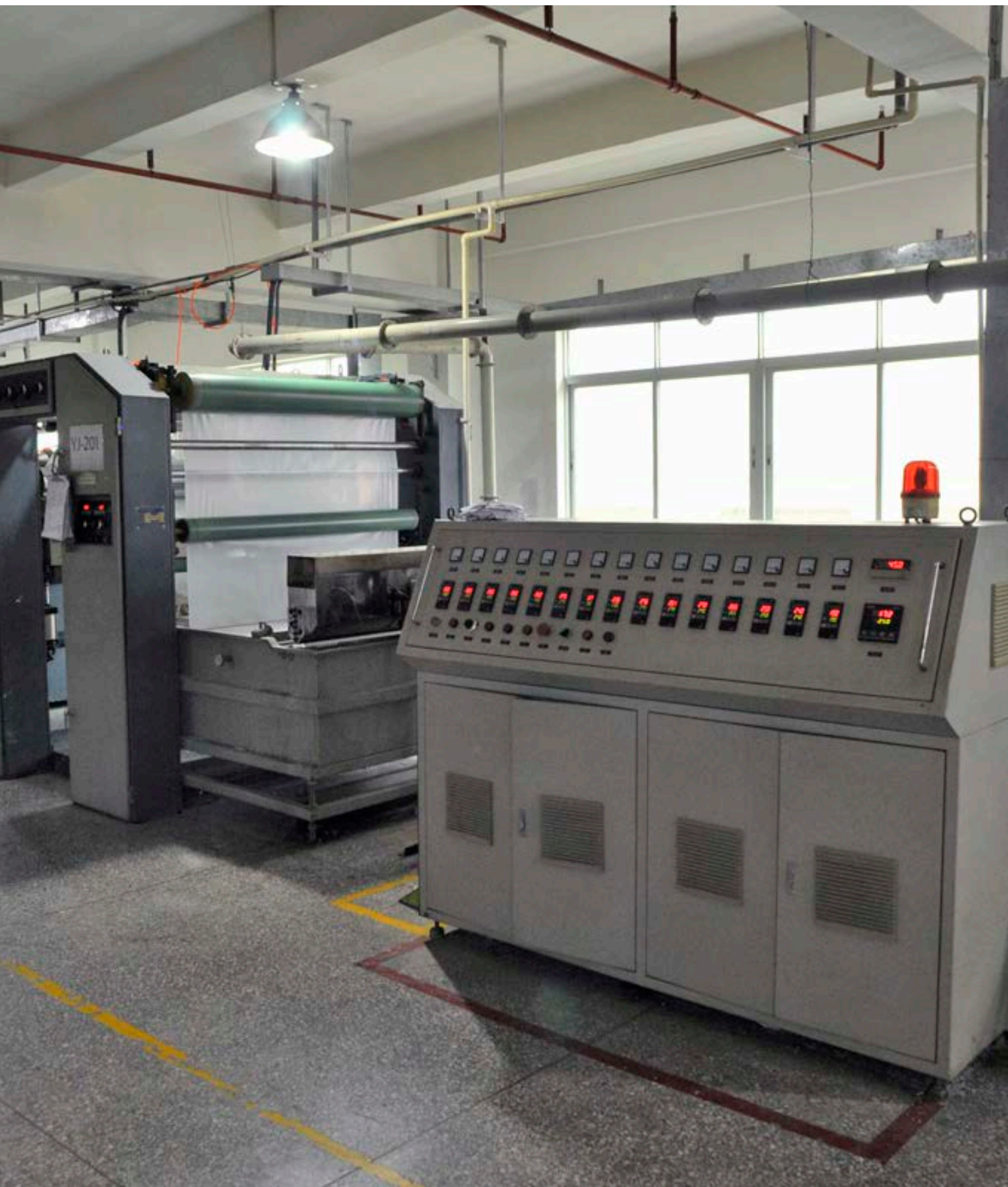
The melted PE material passes behind this control section into the extruder (at the left).
