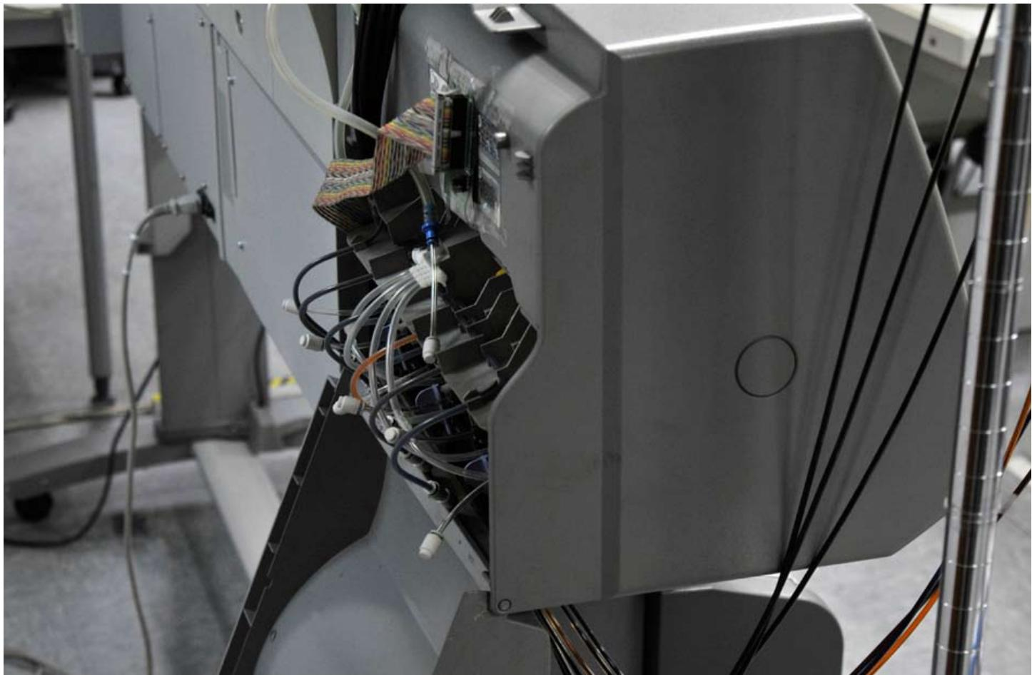
*All the ink feeding system is designed and engineered by Sam-Ink to bypass the original OEM system in order to facilitate bulk-ink feeding. Bulk ink is lower price than cartridges; and of course after-market is less cost than original ink to begin with. You still use cartridges to fill the cartridge space, but the actual bulk ink system bypasses the cartridges.*
