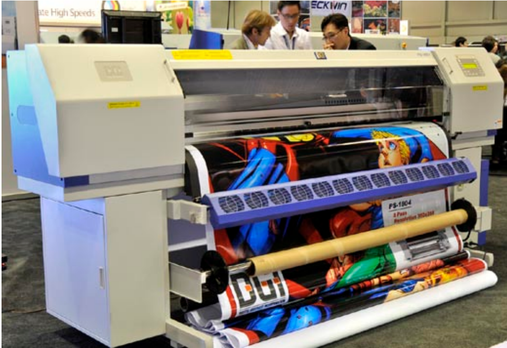
DGI PS-1806 printer with auto feeding media system for large format printing.
