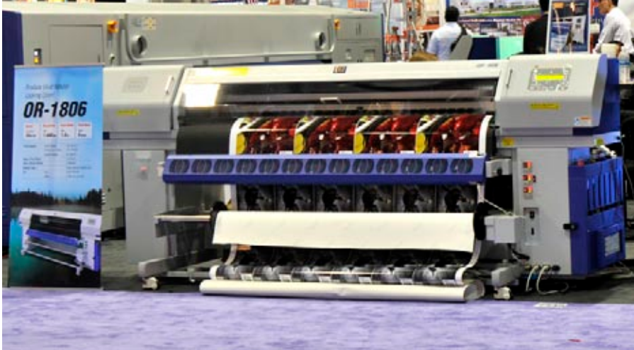
DGI OR-1806 printer with an automated maintenance system (dual action system that uses suction while it purges ink) .
