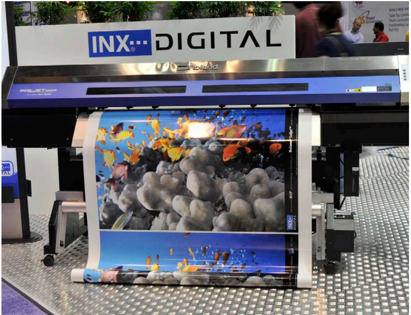
Roland Soljet PRO III XC-540 solvent printer with integrated print/cut capabilities, INX booth.
