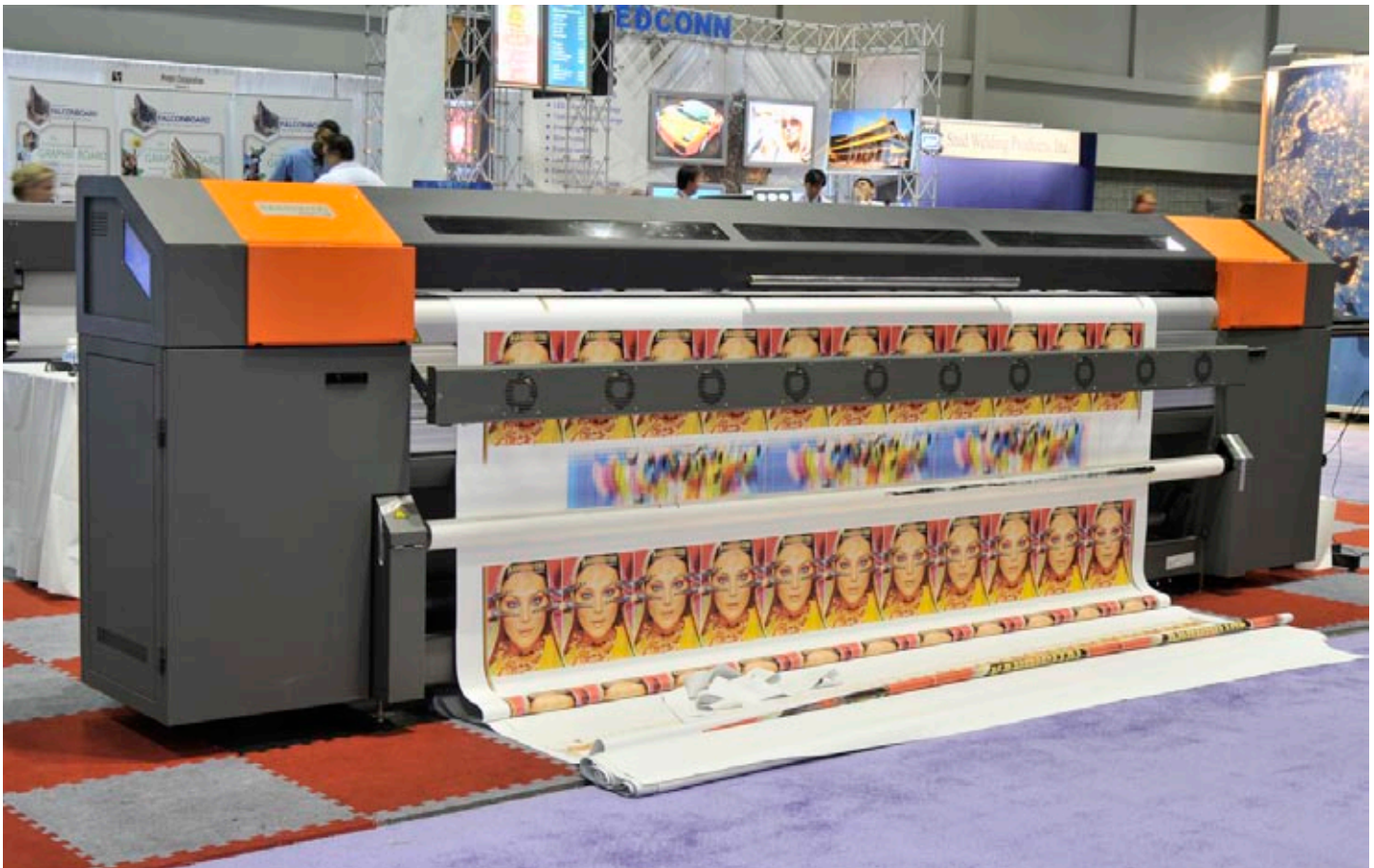
Kanjet 320B printer uses XAAR printheads and has an automatic cleaning system and automatic dry preventing system. However there is no FLAAR recommendation on any Chinese printer if we have not done an inspection of the factory and interviews with end-users.
