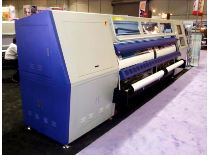
The PS 3206D dual media handling system supports two 1.5 meter supply rolls for dual media printing.
