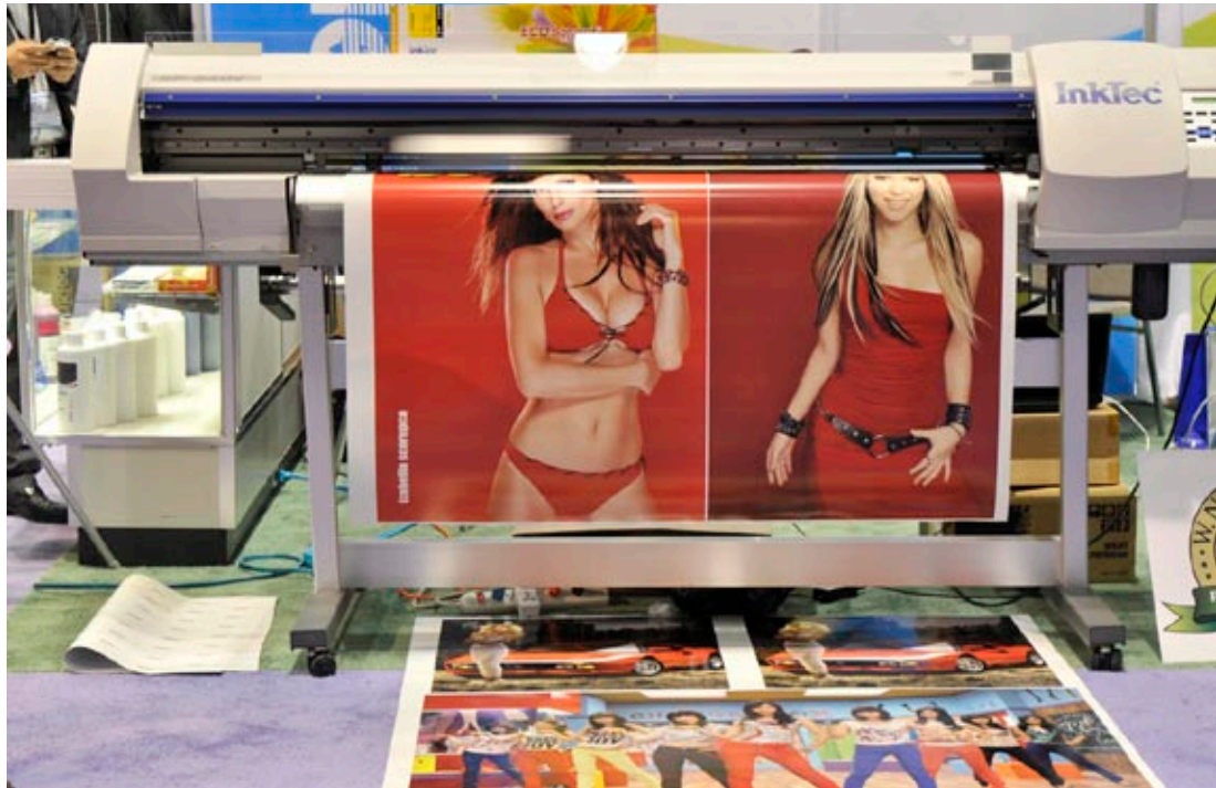
Roland Versacamm SP-540V printer with removable pinch rollers and adjustable printheads (2.2 mm lowest, to 3,2 mm highest), Inktec booth.
