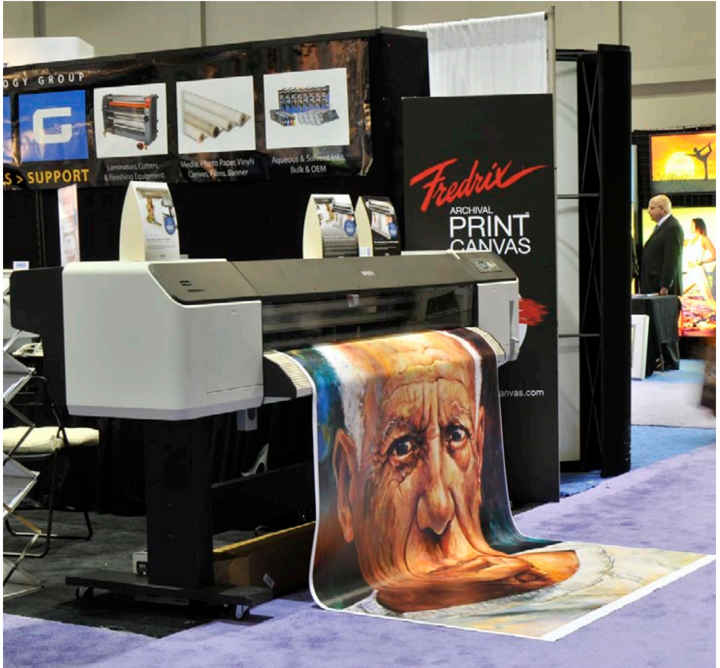
Epson Stylus Pro GS6000 solvent printer at DTG (Digital Technology Group) booth. This printer has a robust take-up reel system for complete, long-run unattended production and a professional roll media handling up to 64 inches wide.
