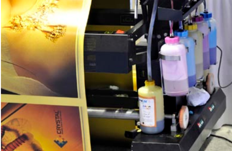
Ink containers close-up. The ink supply system provides constant ink pressure and constant ink heating temperature, which ensures smooth and stable printing.
