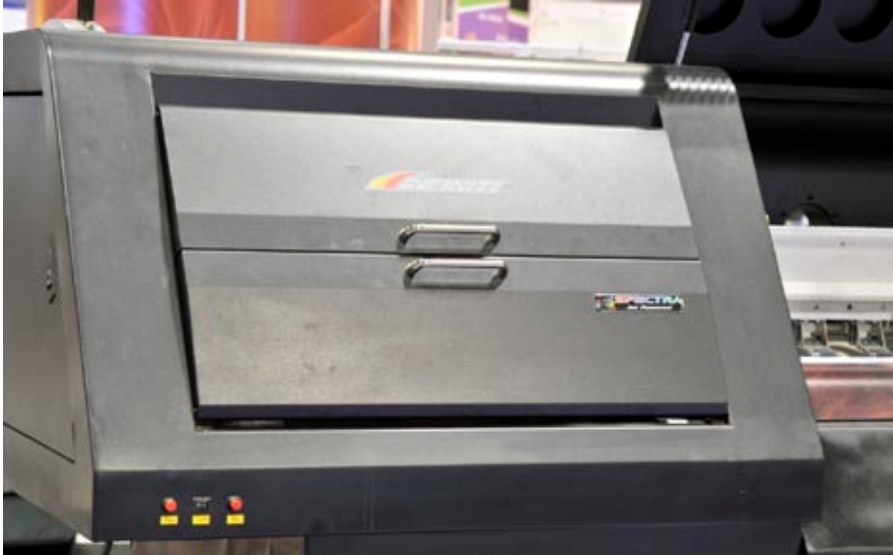
Infiniti 3360 SW 10' superwide printer, has 16 Spectra Skywalker print heads to achieve up to 1200dpi with photo quality.
