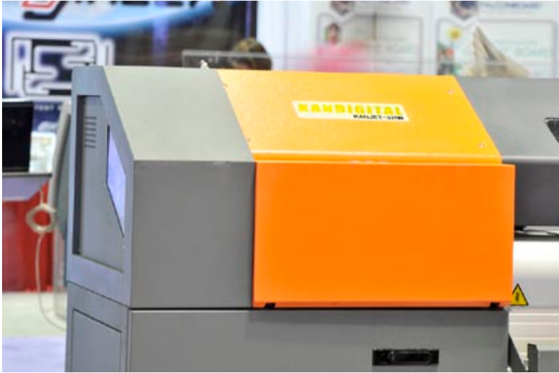
Kanjet 320B printer uses XAAR printheads and has an automatic cleaning system and automatic dry preventing system.
