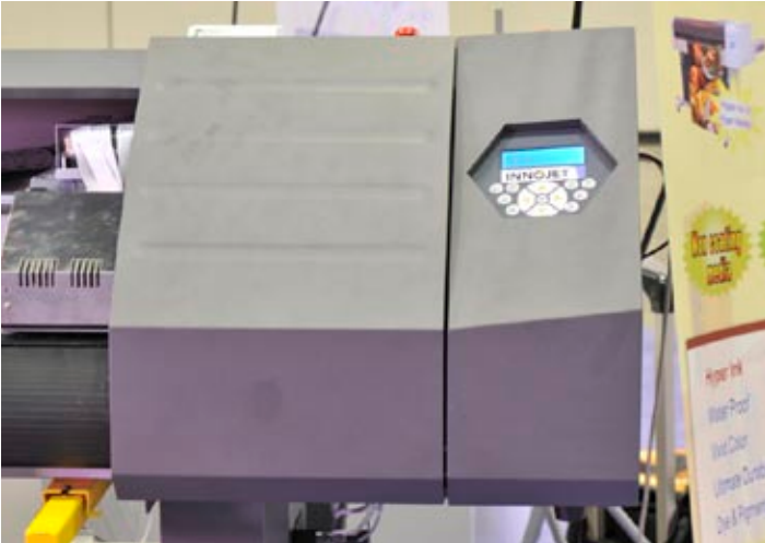
The Innojet 1802 has dual heads that can be replaced separately and can have height adjusted.
