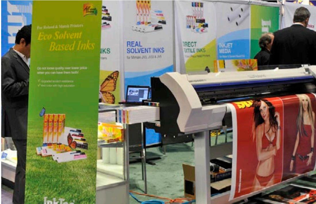
Roland Versacamm SP-540V printer with removable pinch rollers and adjustable printheads (2.2 mm lowest, to 3,2 mm highest), Inktec booth.
