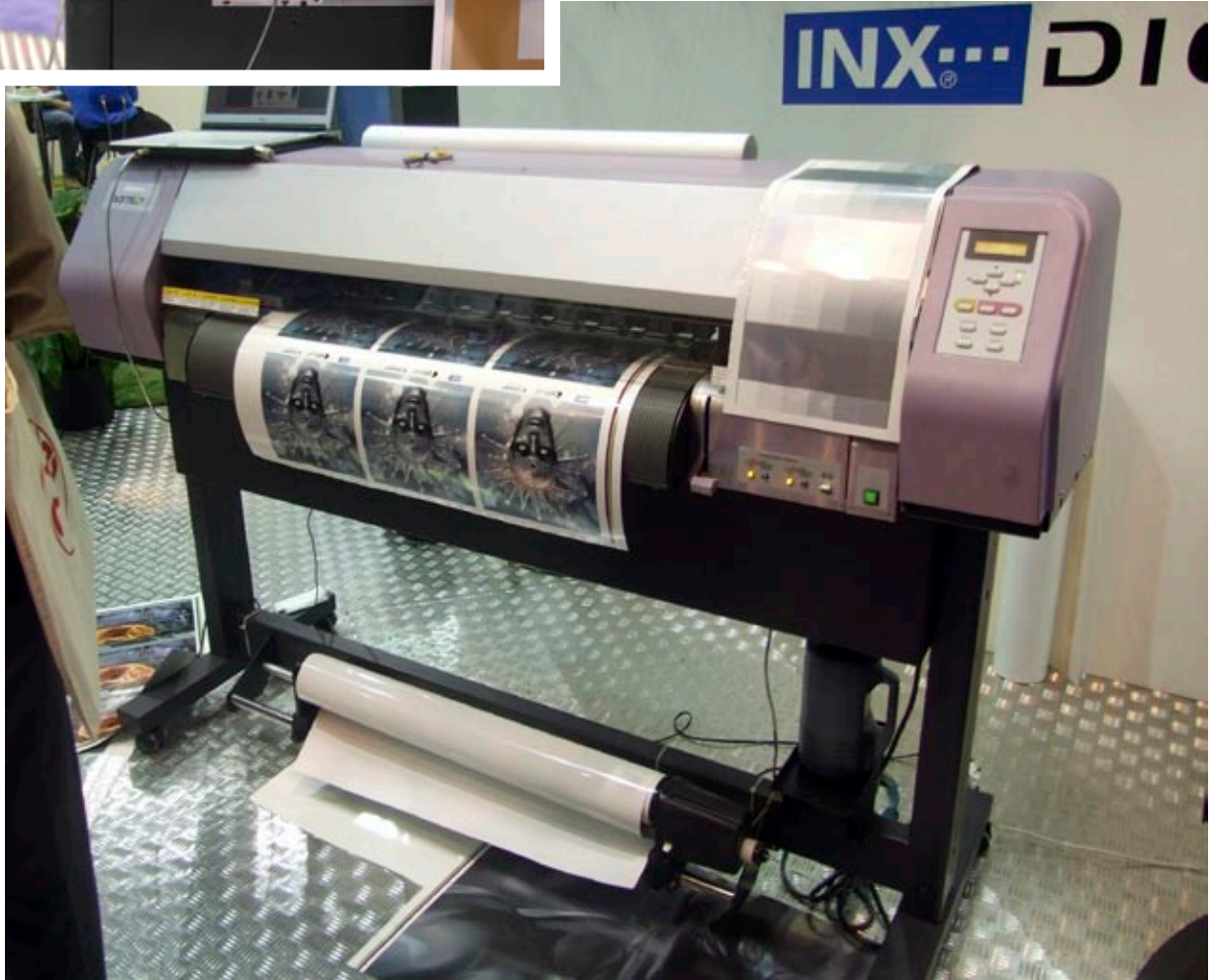
Mimaki JV3-75SP II uses an automatic take-up device uses tension to allow for unattended and continuous printing.
