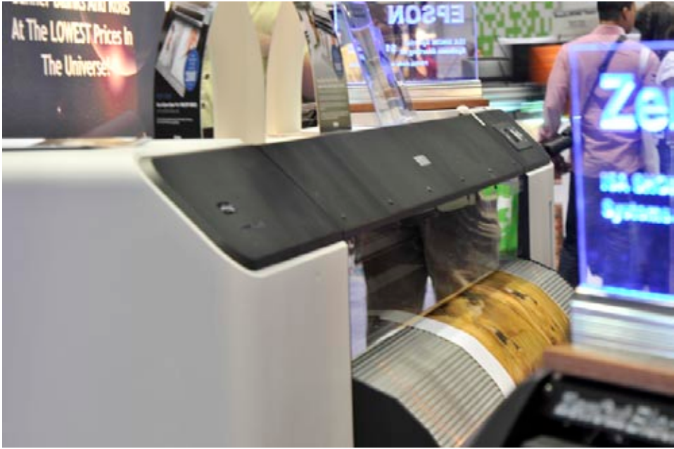
Industry standard, rear-in, front-out, roll-to-roll media handling for the Epson Stylus Pro GS6000.
