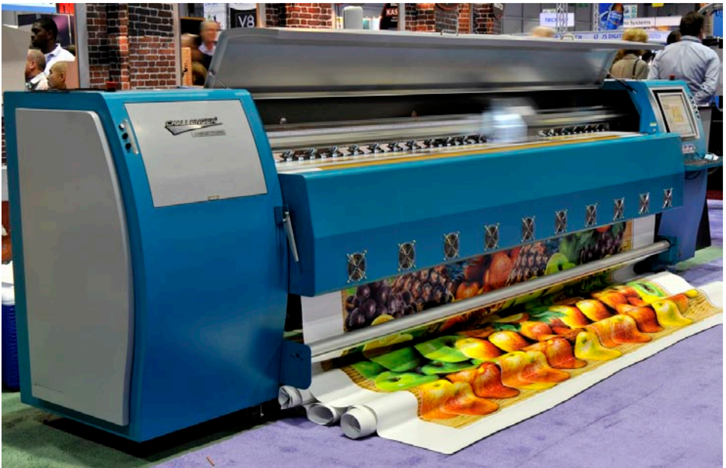
Challenger Jumbo Jet FY-3266j at DGS booth, It has improved automatic cleaning system, one printhead at a time.
