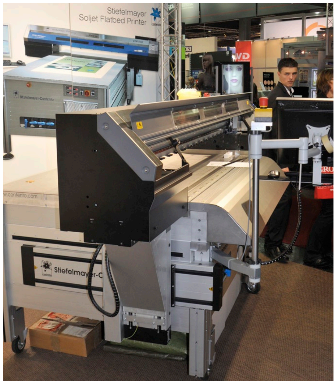
Stiefelmayer-Contento's modified Roland SolJet Pro III XJ-640 printer with custom made flatbed.
