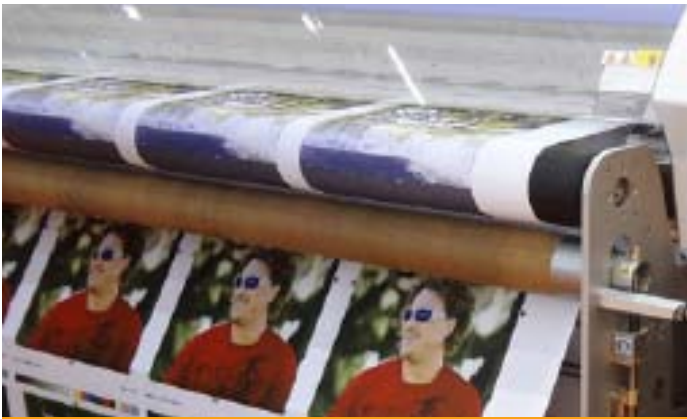
Tension roller system on the ATPColor textile printer.
