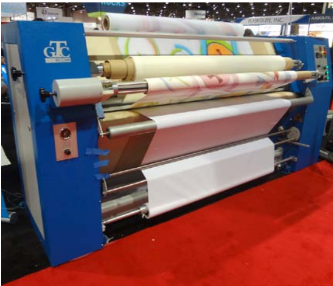
Klieverik GTC, calendering machine.
