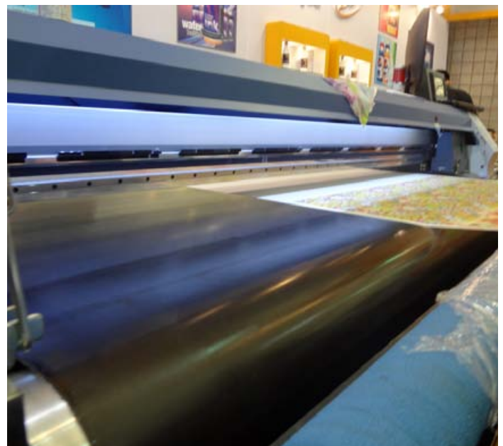
Sticky belt close-up (upper) and complete textile printer (below).
