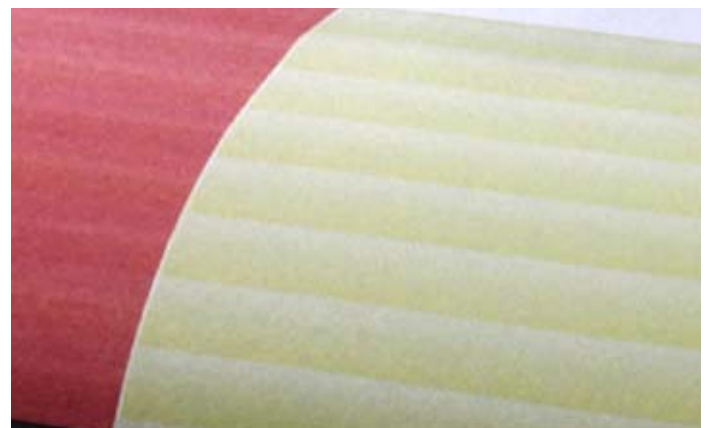
Banding lines in printed fabric sample.
