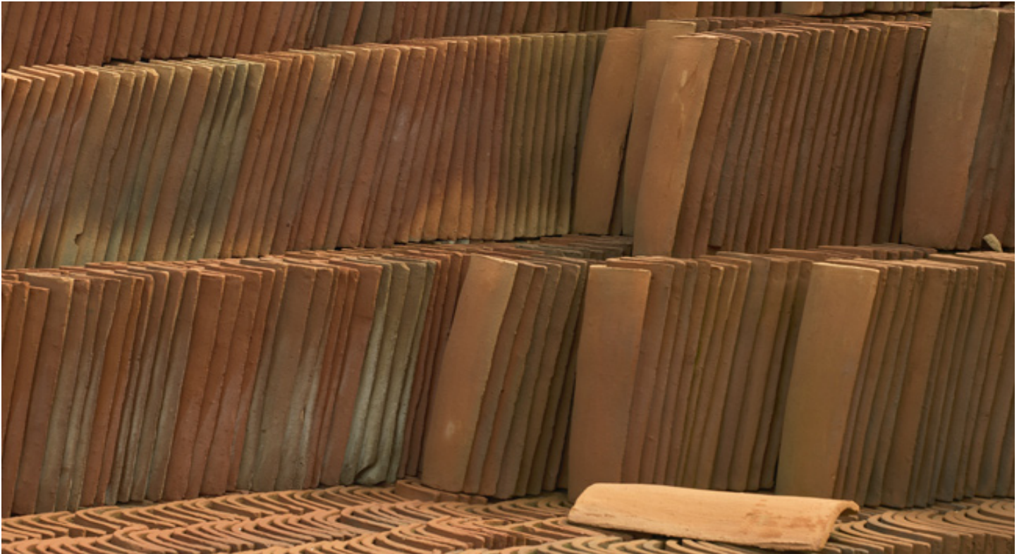
Photograph by Nicholas Hellmuth resulting from Phase One P 30, provided courtesy of Global Graphics Inc. Roofing tiles after they have been fired. The slight variation in color depends on how far they are from the heat source and probably how much air gets to this particular part of the pile.
