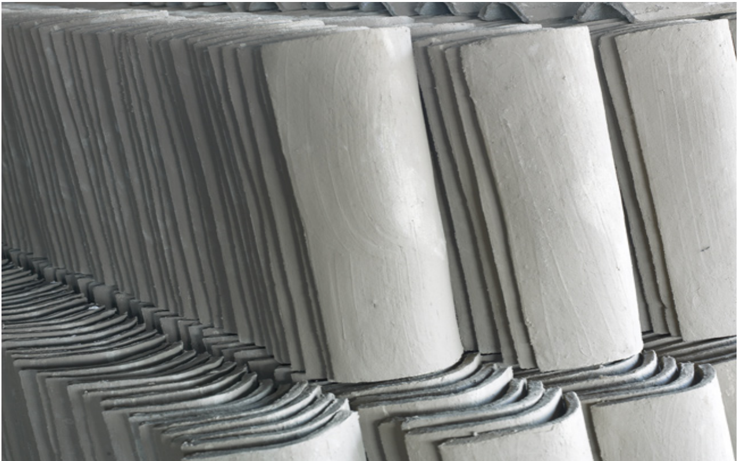
Photograph by Nicholas Hellmuth resulting from Phase One P 30, provided courtesy of Global Graphics Inc. Unfired hand-made roofing tiles waiting to be fired, El Tejar, Guatemala, Central America.
