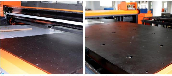
Here you can see there are two kinds of tables, the one that works with vacuum, at the right, and the one that is especially designed to print on glass, at the left.
