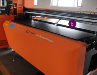
The previous generation of this printer had a system of pinch rollers (a) where the pressure movement was manually adjusted, which took a lot of time. In the next generations this system of pinch rollers will disappear and media will only be pressed down with the pressure roller (b).
