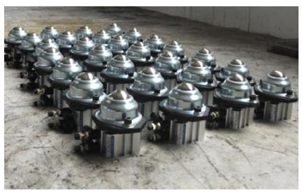
SkyJet glass lifter balls that allow you to raise and lower the glass sheets easily.
