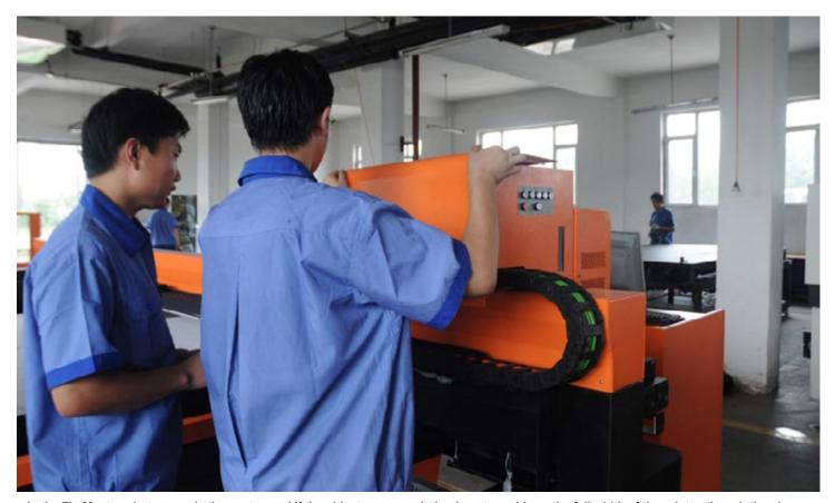
In the FlatMaster what moves is the gantry, and if the object you are printing is not as wide as the full width of the printer, the printhead carriage can hover only over the length of your media.
