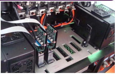
As you can see in this photo, in the previous generations the printhead position was aligned to each other. In the current models the printheads are staggered.
