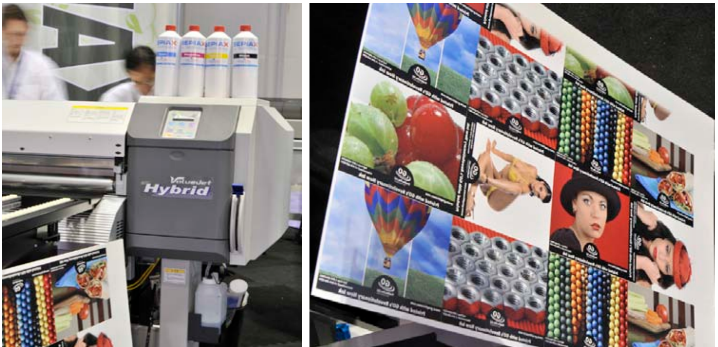
The fact that the vehicle of the pigments is water-based implies that there are not as many dangerous vapors as in a solvent-based ink.
