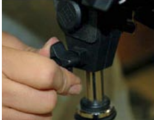
2. Secure it on the light stand, not too tight, some light stands can get damaged, but enough to firmly hold the light.
