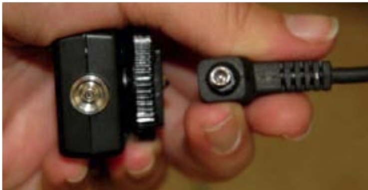
Nikon AS-15 adaptor, connected to a PC cord which is connected to the main light.
