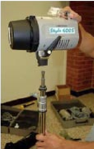
1. Set the light on the light stand (firmly holding the light).
