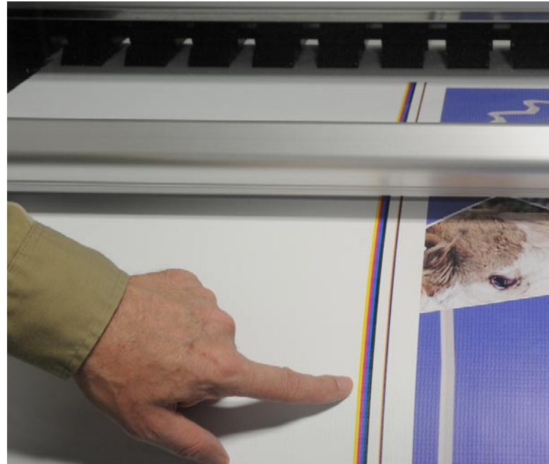
Here you can see an example of a color stripe produced by the Seiko ColorPainter H-104s mild-solvent printer.
