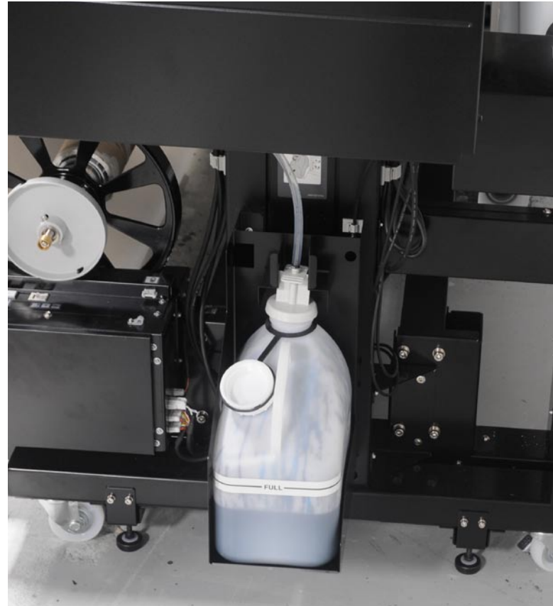
Ink that is purged goes to the waste ink container. Seiko Color Painter H-104s, 2009.
