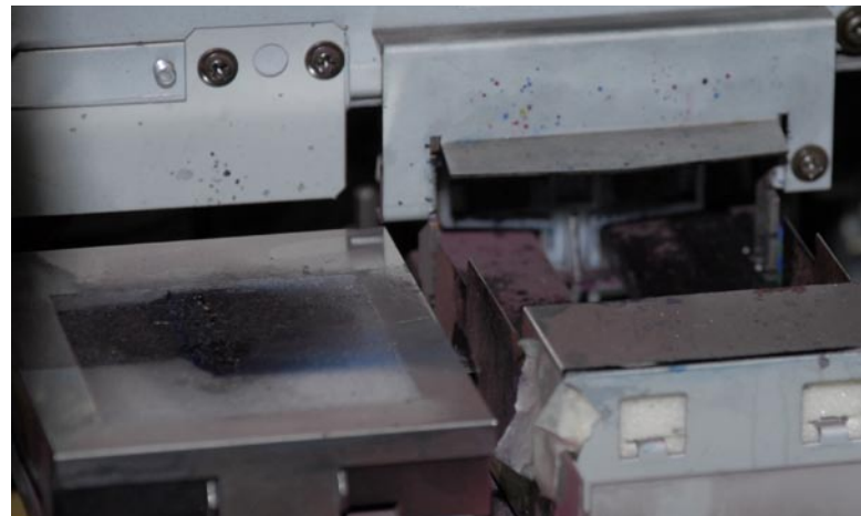
Roland SolJet PROII, spitting ink area, at Perfect Art Guatemala site visit.
