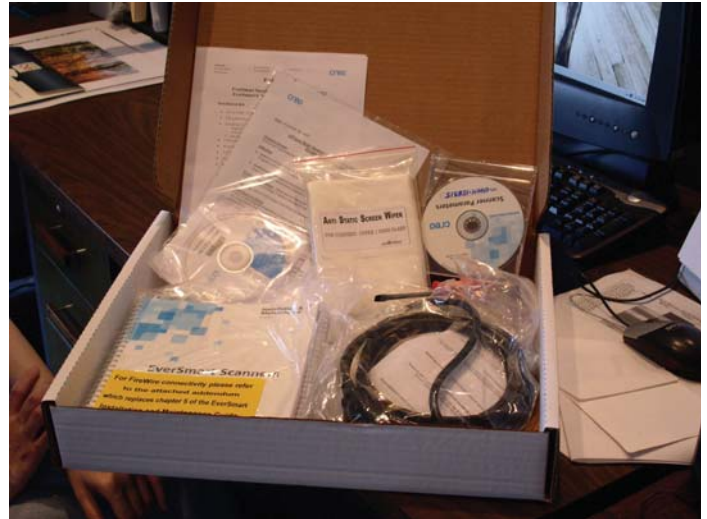
The EverSmart&SUP Installation kit which includes a power cord, 35mm slide holders, the calibration target, calibration slide, and barcode labels.
