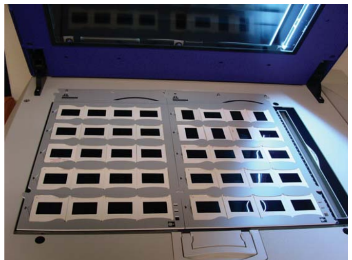
Two 35mm slide holders loaded onto the EverSmart Supreme scanner.
