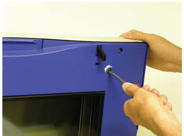
Unlocking the top florecent light in the scanner.
