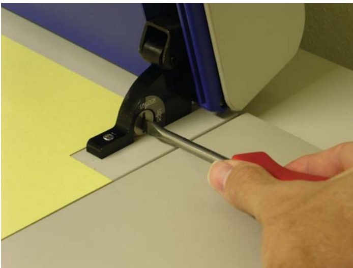
Unlocking the lower florecent light in the EverSmart Supreme scanner.
